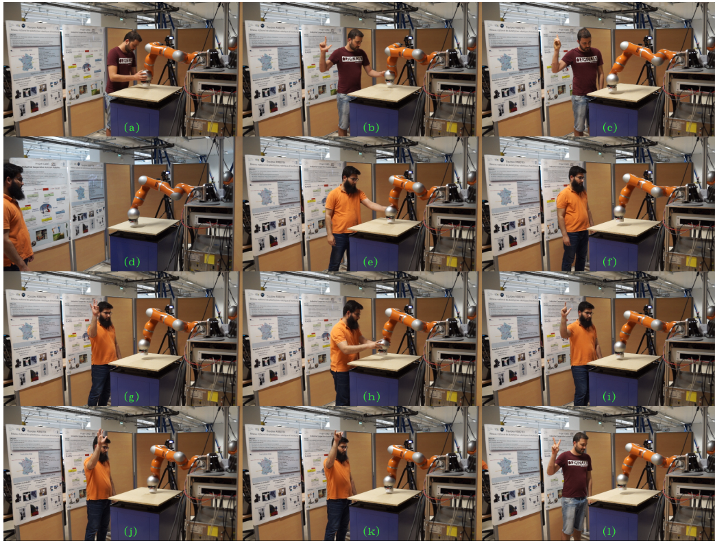
Figure 3.14 Screenshots from the robotic experiment by operators Op1 and Op2 (a) Op1 manually guiding the robot to a waypoint in the workspace. (b) Op1 records the way-points using Record gesture. (c) Op1 replay the taught waypoints by Replay gesture. (d) Op2 stands far from the robot so it moves with full speed. (e) Op2 stops the robot by applying external force (or accidental touch). (f) Op2 stands near the robot, so it moves slowly ensuring operator's safety. (g) Op2 gives Reteach command to the robot. (h) Op2 sets the new waypoints manually. (i) Op2 gives Record command. (j) Op2 stops the robot by Stop gesture. (k) Op2 resumes the robot operation by Resume gesture. (l) Op1 ends the robot operation by giving End command.
