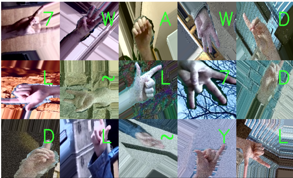
Figure 3.9 Image processing operations applied to the training images include color-shift, zoom, shear, rotation, axes flip and position shift processes.
