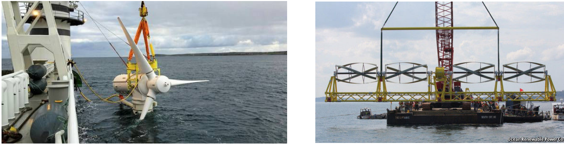
Figure 1.2: From left to right, example of axial flow turbine (Atlantis AR1500) and transverse flow turbine (TidGen)
