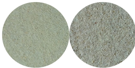
FIGURE 3.2 – Photos des sables S_{328} ( D_{50} = 328\mu m ) et S_{617} ( D_{50} = 617\mu m )
