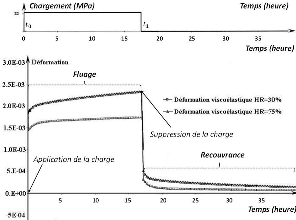
FIGURE 1.8 – Fluage-recouvrance sous climat constant [6].
