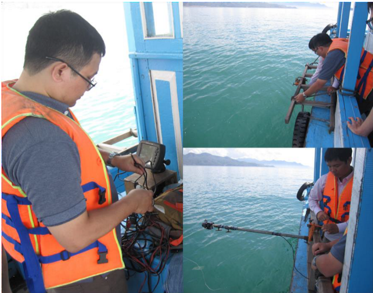
Figure 4.4: Field photo showing the course of a bathymetric survey during NT1.
