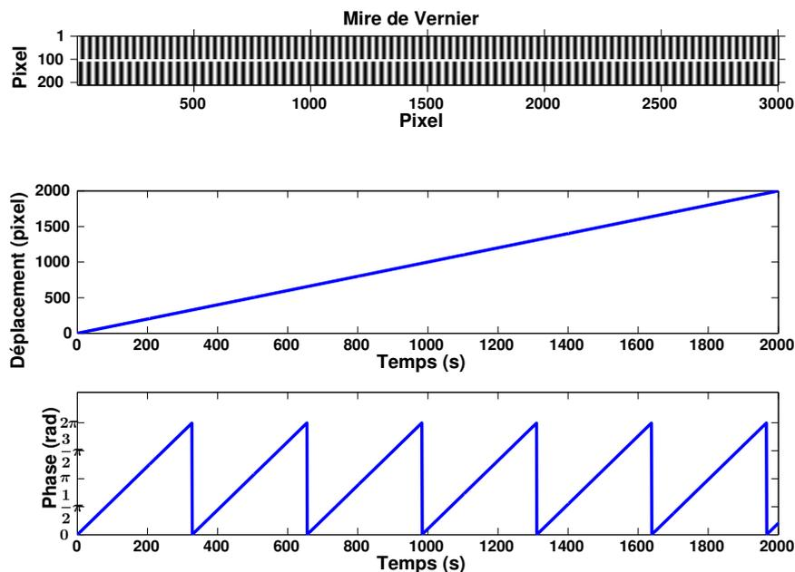
FIGURE 3.6 – Mire de Vernier créée arbitrairement :  $\tilde{\lambda}_1 = 31.41$  pixels,  $\tilde{\lambda}_2 = 34.74$  pixels,  $n_1 = 59.26$ ,  $n_2 = 53.58$ ,  $\tilde{\Lambda} = 327.7$  pixels
