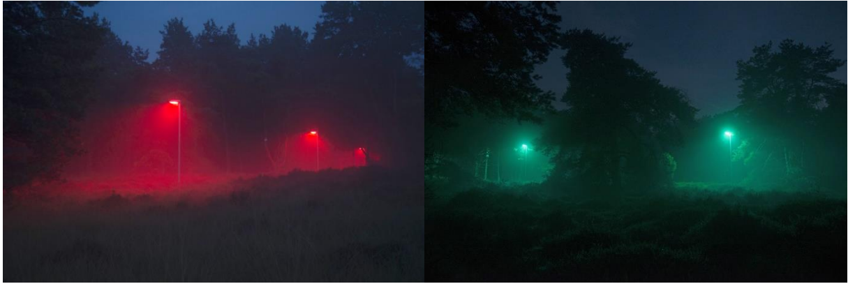
Fig. 35. Pictures of the installations of the large scale project LichtOpNatuur testing the effect of different color spectra on a diversity of taxa (photos by K. Spoelstra)
