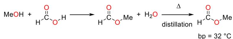
A distillation setup was charged with methanol (6.1 mL, 140 mmol methanol containing 4% of methylformate) and 3 equiv. of formic acid (16 mL, 420 mmol). The reaction mixture was heated to 35 °C to ensure the distillation of methylformate (bp<sub>MeOCHO</sub> = 32 °C). The reaction was carried out for 5 h, providing methylformate in 86 % yield (120 mmol, 7.3 mL) with 99 % purity.
