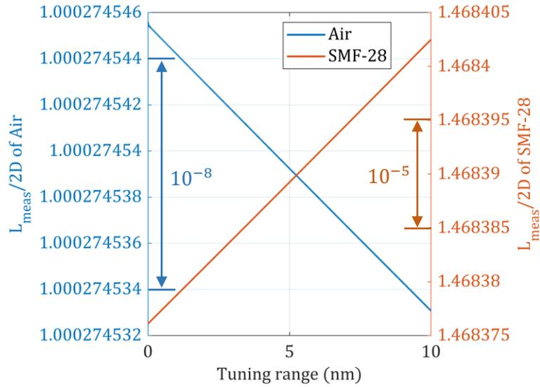
Fig. 2.3. Ratio between the measured OPD and the round-trip geometric length of air ( $T=15\text{ }^{\circ}\text{C}$ ,  $P=101\text{ }325\text{ Pa}$ , relative humidity = 0% and 450 ppm  $\text{CO}_2$ ) and SMF-28 fiber.
