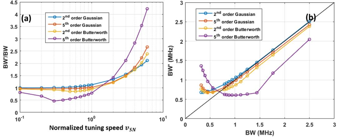
Fig. 3.8. The bandwidth of the filtered signal at different chirp rates. (a) Ratio between  $BW$  and  $BW'$ ; (b) The bandwidth of the filtered signal. Chirp rate  $v_s = 624$  GHz/s.  $v_{SN}$ : normalized chirp rate defined in Eq. 3.31.
