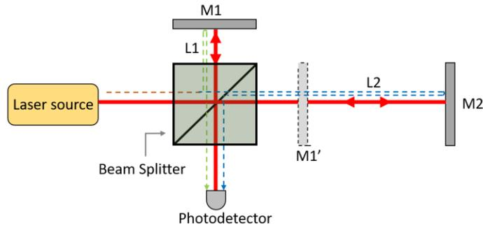
Fig. 2.1. Illustration of Michelson type interferometer. Red solid lines: laser beam. Green and blue dashed lines: light paths of the reference and the measurement.  $M_1$ ,  $M_2$ : mirrors;  $L_1$  and  $L_2$ : light paths.
