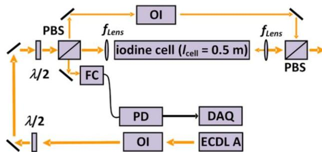
Fig. 1.19. Setup for high-resolution saturation spectroscopy. ECDL A, frequency-scanning external cavity diode laser; OI, optical isolator; FC, fiber coupler; PD, photo detector;  $\lambda/2$ , half-waveplate; PBS, polarizing beamsplitter; DAQ, data acquisition. After Ref. [48].
