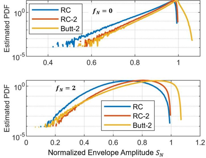
Fig. 4.6. Estimated PDF with different filters. (a) PDF in frequency position  $f_N = 0$ . (b) PDF in frequency position  $f_N = 2$ . Parameters used are  $\tau = 5$ ,  $v_{SN} = 0.1$  and  $\Delta v_N = 0.04$ .
