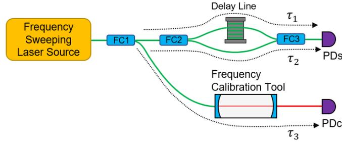
Fig. A1. Model of frequency FSI based on Mach-Zehnder interferometer. FC: Fiber coupler. PDs and PDC: Photodetector for receiving the interference signal and the calibration signal.  $\tau_1$ ,  $\tau_2$  and  $\tau_3$  are the time delays of the light paths as marked.
