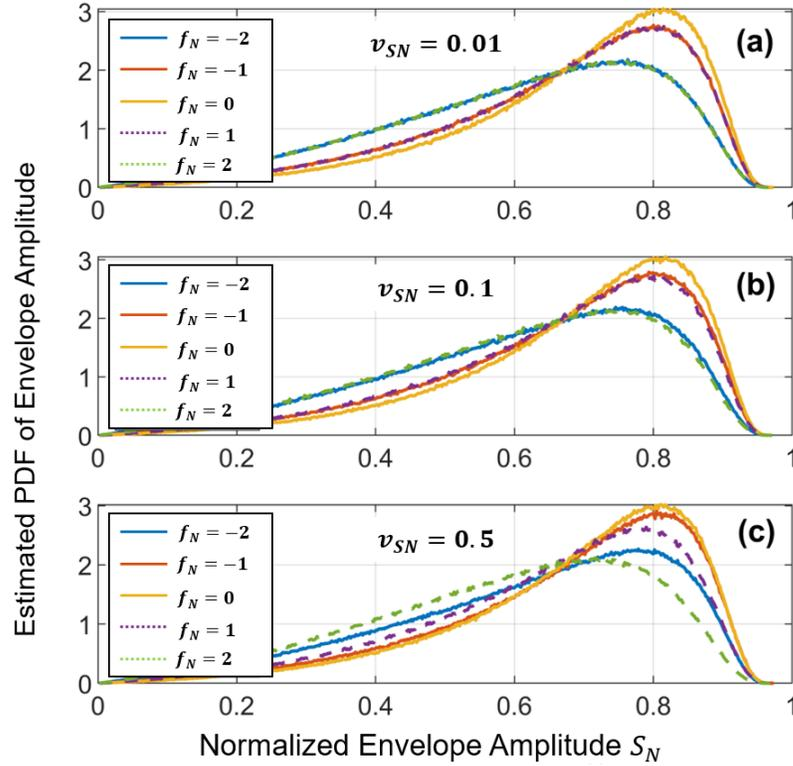
Fig. 4.5. Estimated PDF at different frequency positions  $f_N$  with different normalized tuning speed  $v_{SN}$ . (a)  $v_{SN} = 0.01$ . (b)  $v_{SN} = 0.1$ . (c)  $v_{SN} = 0.5$ . Parameters used are  $\tau = 5$ ,  $\Delta v_N = 0.32$  with RC filter.
