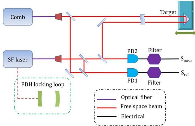
Fig. 1.16. Schematic of ADM system using frequency comb as light source to perform MWI. BS, beam splitter; PD, photodetector;  $S_{meas}$ , measurement signal; and  $S_{ref}$ , reference signal. SF: single frequency laser. After Ref. [33].
