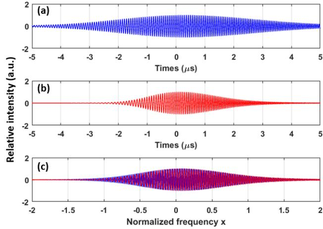
Fig. 3.6. The filtered signal at different chirp rate. (a)  $\nu=624\text{GHz/s}$ ,  $BW=2.5\text{MHz}$ , 5<sup>th</sup> Gaussian filter. (b)  $\nu=2.5\text{ THz/s}$ ,  $BW=5.0\text{ MHz}$ , 5<sup>th</sup> Gaussian filter. (c) The filtered signal as a function of the normalized frequency  $x = \frac{2(f-f_c)}{BW}$ , where  $f_c$  and  $BW$  are the central frequency and the bandwidth of the NBF respectively.
