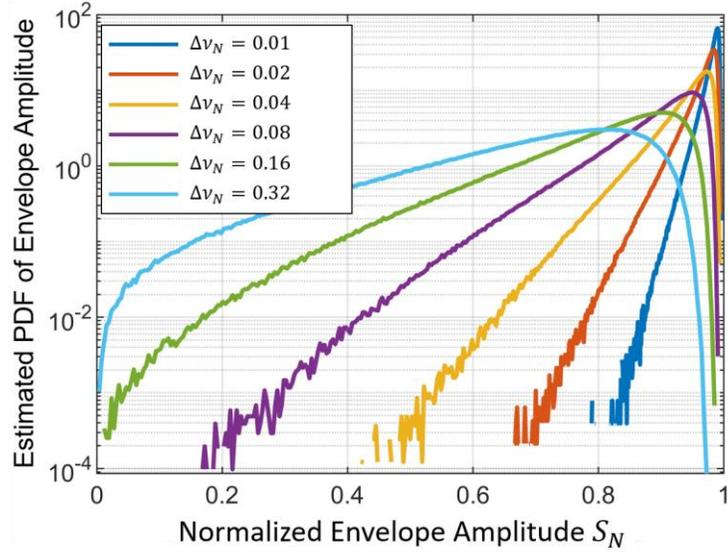
Fig. 4.4. Estimated PDF of envelope amplitude  $S_N$  at the passband central frequency ( $f_N = 0$ ) for different phase noise levels  $\Delta v_N$ . ( $\tau = 5$ ,  $v_{S_N} = 0.1$ . The definition of the parameters is summarized in Appendix D.)
