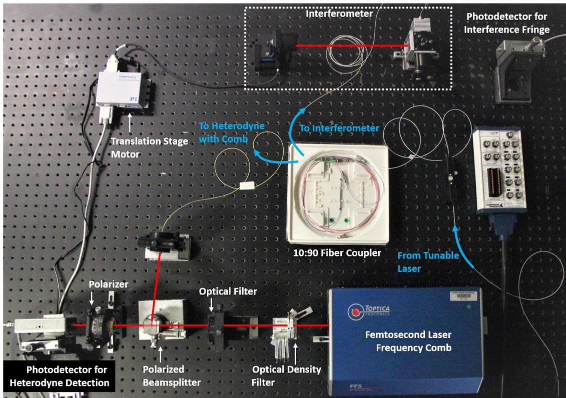
Fig. 5.1. Photograph of the comb-referenced ADM system.
