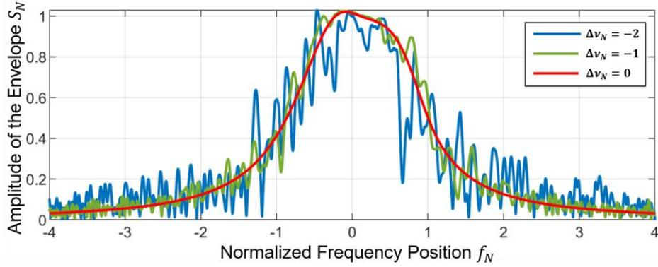
Fig. 4.7. The envelope of the filtered calibration signal with different phase noise level. Parameters used are  $\tau = 5$ ,  $v_{SN} = 0.5$  with RC-2 filter. The asymmetry profile generated without phase noise  $\Delta v_N = 0$  is caused by the linear chirp of the input signal. The definition of the parameters is summarized in Appendix D.
