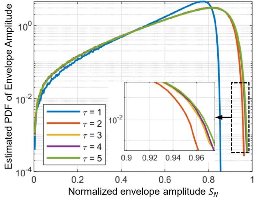
Fig. 4.3. Effect of the integration time truncation,  $\tau$ . The parameters here  $f_N = 0$ ,  $v_{SN} = 1$  and  $\Delta v_N = 0.5$ , where the definition of the parameters is summarized in Appendix D.
