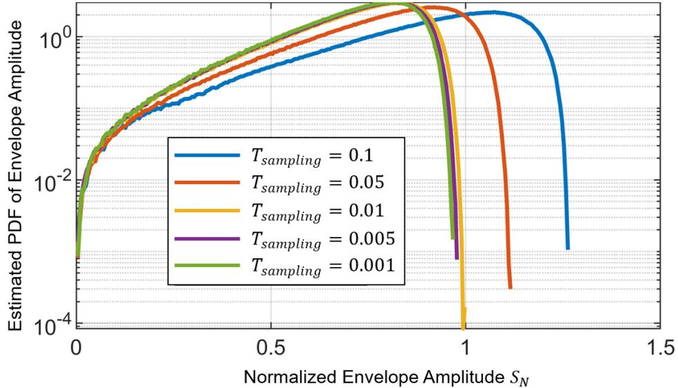
Fig. 4.2. Effect of sampling time interval  $T_{sampling}$ . The estimated PDFs are generated by setting the parameters at the largest value required:  $\tau = 5$ ,  $v_{SN} = 1$  and  $\Delta v_N = 0.5$ , where the definition of the parameters is summarized in Appendix D.
