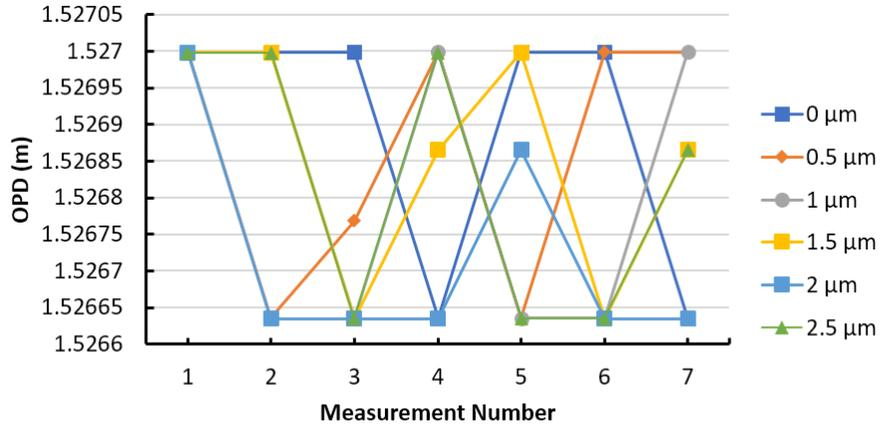
Fig. 5.10. Measurement result using direct Fourier transform method. The different series correspond to displacements of the target by 0.5  $\mu\text{m}$ , 1  $\mu\text{m}$ , 1.5  $\mu\text{m}$ , 2  $\mu\text{m}$  and
