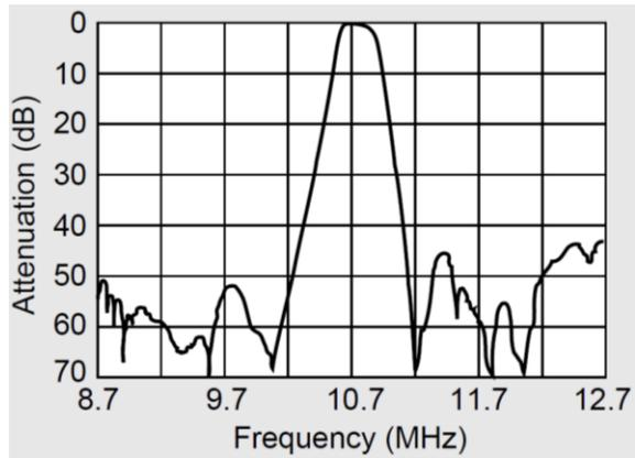
Fig. C1. Transfer function of the Ceramic filter (Model SFE10.7A, Murata).
