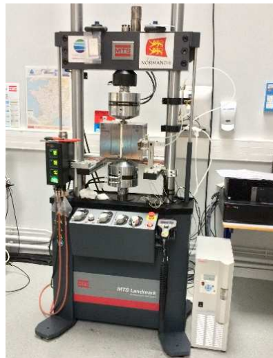
Figure 5-6. The tensile stress rig used for stress-ageing at intermediate temperature.
