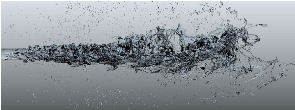
Figure 3.8: Atomization of a water jet in quiescent air. Taken from [Le Chenadec and Pitsch, 2013].
