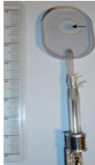
Figure 1.10: Scheme and photography of a nano-cell. (a) Description of a nano-cell: 1 - sapphire or garnet plates, 2 - titanium or platinum strips, 3 - glue, 4 - sapphire tube, 5 -glass side-arm. (b) Photograph of a nano-cell containing Cs atomic vapor: L varying in range from 50 nm to 2 \mu\text{m} . One may see the interferometric pattern which is formed by the reflection of visible light from the internal surfaces of the NC.
