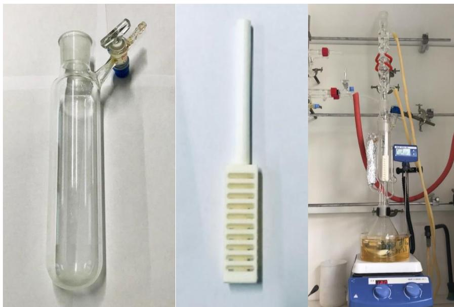
**Figure 3.4** From left to right: Schlenk tube, home-made Teflon sample holder and lastly, Soxhlet system used to clean the slides after silanization.
