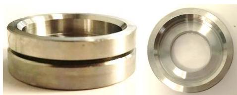
**Figure 3.6** Glass slides metallic holder with an internal diameter of 19 mm and external of 3.5 cm.
