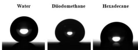
Fig. 7. Picture of the droplets deposited on PPy-NOF<sub>6</sub> surfaces with all probe liquids. Electropolymerization by cyclic voltammetry (3 scans) in a 0.1 M solution of  $\text{Bu}_4\text{NClO}_4/\text{acetonitrile}$ .
