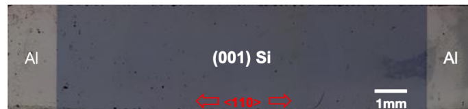
Fig. 3.3 p -type silicon cantilevers with ohmic contacts ( Al ) visible at each end used in the experiments reported on in Chapter 5. The (001) oriented silicon active layer is marked as Si with boron doping ( \rho < 0.01 \Omega \text{ cm} ). The long axis of the cantilever is parallel to the \langle 110 \rangle crystal direction as indicated by the red arrows.
