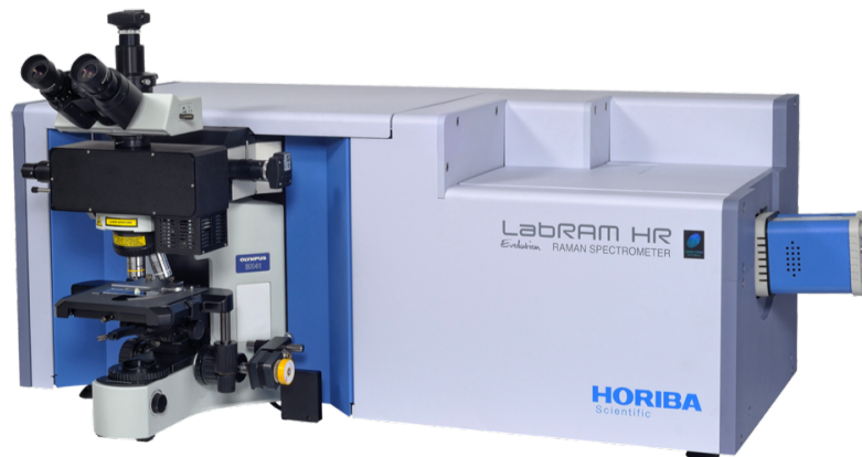
Fig. 5.6 Picture of the Raman spectrometer, a LabRAM HR Evolution produced by Horiba. Extracted from www.horiba.com .
