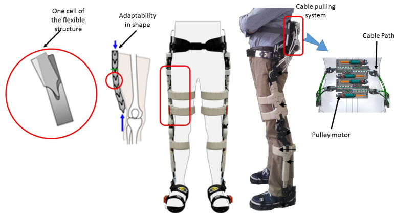
Figure 3.22 Samsung Semi Rigid Exoskeleton
