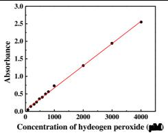
Figure 2. 6 Calibration curve of hydrogen peroxide concentration measurement with TiOSO<sub>4</sub>. Absorbance at  $\lambda$ = 408 nm as a function of concentration with absorbance (1-cm cells). The total volume of liquid is 1000  $\mu$ L sample. 900  $\mu$ L of samples were mixed with 100  $\mu$ L of the commercial solutions of TiOSO<sub>4</sub>
