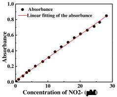
Figure 2. 5 Calibration curves of measurement of sodium nitrite solution with Griess reagents in different concentration ranges. Concentrations of nitrate ranges from 0.2  $\mu M$  to 28  $\mu M$ . Absorbance at  $\lambda = 522$  nm as a function of concentration with absorbance (1-cm cells). The total volume of liquid is 1000  $\mu L$  sample. 900  $\mu L$  of samples were mixed with 100  $\mu L$  of the commercial solutions of Griess reagents
