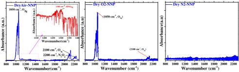
Figure 3. 3 Infrared spectra of feed gases of dry Air,  $O_2$  and  $N_2$ . Discharge conditions for all discharges: 20 kV of input voltage, 1000 sccm of gas flow rate (300 sccm of discharge gas and 700 sccm of  $N_2$ ). Discharge power of gases are 312±49 mW for Air; 293±43 mW for  $O_2$  and 271±4 mW for  $N_2$ . The peaks of 1050 cm<sup>-1</sup> and 2100 cm<sup>-1</sup> are  $O_{3g}$ , the peak of 1310 cm<sup>-1</sup> is  $HNO_{3g}$  and the peak of 2200 cm<sup>-1</sup> is  $N_2O_g$ .
