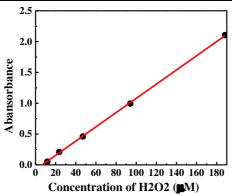
Figure 2. 7 Calibration curve of hydrogen peroxide concentration measurement with Cu ions. Absorbance at  $\lambda$ = 453 nm as a function of concentration with absorbance (1-cm cells). The total volume of liquid is 800  $\mu$ L sample. 800  $\mu$ L of samples were mixed with 50  $\mu$ L of the commercial solutions of the two reactants respectively
