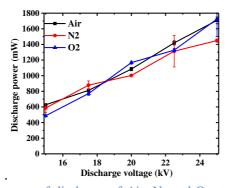
Figure 3. 20 Discharge power of discharge of Air,  $N_2$  and  $O_2$  at different input voltages. Discharge conditions: Flow rate is 300 sccm, height of electrode to water surface is 7 mm, treatment time is 2 min and volume of treated tap water is 3 mL.
