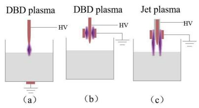
Figure 1. 1 Types of direct gaseous phase discharge outside the aqueous phase. (a) is a DBD plasma touching the water surface, (b) is a DBD plasma non-touching the water surface and (c) is a plasma jet touching water surface, the high voltage electrode is coated with dielectric. The figures are reproduced from [113]
