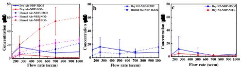
Figure 3. 6: Concentrations of  $NO_2^-$ ,  $NO_3^-$  and  $H_2O_{2aq}$  produced by NBPs at different flow rates. Discharge condition for all NTP: 20 kV of input voltage and 4 min of treatment time. Discharge power of gases are 312±49 mW for dry Air, 322±37 mW for humid Air; 293±43 mW for dry  $O_2$ , 321±35 mW for humid  $O_2$  and 271±4 mW for dry  $O_2$ . Volume of water is 5 mL and the inner tube is immersed inside water for 1 mm. Results are represented as mean ± standard deviation.
