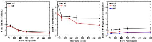
Figure 3. 16 Yield of  $NO_2^-$ ,  $NO_3^-$  and  $H_2O_{2aq}$  at different flow rates. Discharge conditions: Treatment time is 2 min, height of electrode to water surface is 7 mm, input voltage is 20 kV and volume of tap water is 3 mL.
