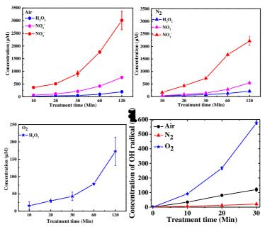
Figure 5. 1 Concentration ( $\pm$ standard deviation) of NO<sub>2</sub><sup>-</sup>, NO<sub>3</sub><sup>-</sup>, aqueous H<sub>2</sub>O<sub>2</sub> and aqueous OH radical as a function of treatment time (min) in plasma treated liquid for Air, N<sub>2</sub> and O<sub>2</sub> NTP (Vpp=20kV,  $\Phi$ =1.5 SLM, tap water: V<sub>L</sub>= 100 ml and TPA-2Na solution: V<sub>L</sub>= 100 ml)
