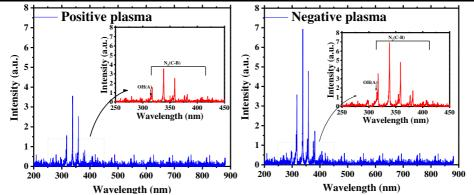
Figure 3. 11 Emission spectra of the Air positive and negative plasmas. HV electrode is fixed 3 mm above the tap water surface and discharge voltage on HV electrode is 20 kV<sub>p-p</sub>, Air flow rate is 300 sccm and the plume is contacting with tap water surface. Emission is accumulated along entire discharges volume.
