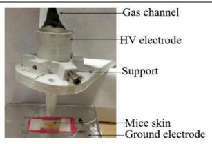
Figure 2. 17 The photo of NTP single jet
