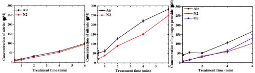
Figure 3. 13 Concentration of  $NO_2^-$ ,  $NO_3^-$  and  $H_2O_{2aq}$  at different treatment times. Discharge conditions: Flow rate is 300 sccm, height of electrode to water surface is 7 mm, input voltage is 20 kV and volume of tap water is 3 mL.
