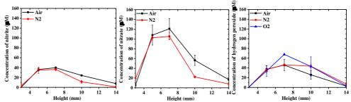
Figure 3. 18 Concentration of  $NO_2$ ,  $NO_3$  and  $H_2O_{2aq}$  t different heights. Discharge conditions: Flow rate of all gases is 300 sccm, treatment time is 2 min, input voltage is 20 kV and volume of tap water is 3 mL.
