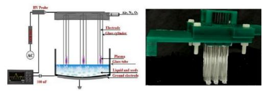
Figure 2. 10 Schematic diagram (left) and Photo (right) of the 3×3 array of glass tubes in side view of the plasma setup. The device is made of 3×3 glass tubes set in an array and fabricated by 3D printer. The gap between electrode and water surface is 7 mm.
