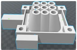
Figure 2. 9 3D model of 9-electrode DBD plasma setup
