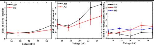
Figure 3. 22 Yield of  $NO_2$ ,  $NO_3$  and  $H_2O_2$  at different input voltages. Discharge conditions: Flow rate is 300 sccm, height of electrode to water surface is 7 mm, treatment time is 2 min and volume of tap water is 3 mL.
