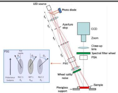
Figure 2. 18 Schematic of experimental setup for the backscattering Mueller matrix measurement [239]
