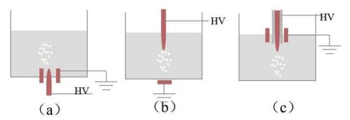
Figure 1. 2 Types of multiphase discharge. (a) is a discharge bubbling from bottom, (b) is a discharge bubbling form tap and (c) is a discharge bubbling from top but with the high electrode coated with a dielectric layer. The figures are reproduced from [113].
