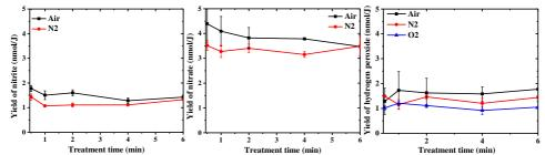
Figure 3. 14 Yield of NO<sub>2</sub><sup>-</sup>, NO<sub>3</sub><sup>-</sup> and H<sub>2</sub>O<sub>2</sub>at different treatment times. Discharge conditions: Flow rate is 300 sccm, height of electrode to water surface is 7 mm, input voltage is 20 kV and volume of treated tap water is 3 mL.
