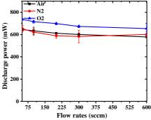
Figure 3. 15 Discharge power of Air,  $N_2$  and  $O_2$  at different gas flow rates. Discharge conditions: Treatment time is 2 min, height of electrode to water surface is 7 mm, input voltage is 20 kV and volume of tap water is 3 mL.
