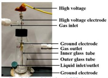
Figure 2. 1 Photo of single electrode DBD plasma setup
