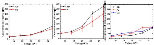
Figure 3. 21 Concentration of  $NO_2$ ,  $NO_3$  and  $H_2O_{2aq}$  at different input voltages. Discharge conditions: Flow rate is 300 sccm, height of electrode to water surface is 7 mm, treatment time is 2 min and volume of tap water is 3 mL.
