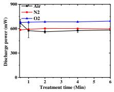
Figure 3. 12 Discharge power of Air,  $N_2$  and  $O_2$  at different treatment times. Discharge conditions: flow rate is 300 sccm, height of electrode to water surface is 7 mm, input voltage is 20 kV and volume of tap water is 3 mL.
