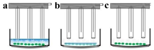
Figure 2. 13 Schematic of electric field treatment with seeds using the 9-electrode in different conditions. The seeds in configuration a can be immersed seeds or soaked seeds, in configuration b is wet seeds and in configuration c is dry seeds
