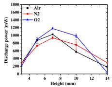
Figure 3. 17 Discharge power of discharge of Air,  $N_2$  and  $O_2$  at different heights. Discharge conditions: Flow rate is 300 sccm, treatment time is 2 min, input voltage is 20 kV and volume of tap water is 3 mL.
