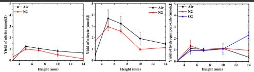
Figure 3. 19 Yields of NO<sub>2</sub><sup>-</sup>, NO<sub>3</sub><sup>-</sup> and H<sub>2</sub>O<sub>2aq</sub> at different heights. Discharge conditions: Flow rate is 300 sccm, treatment time is 2 min, input voltage is 20 kV and volume of tap water is 3 mL.
