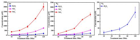
Figure 3. 23 Concentration ( $\pm$ standard deviation) of NO<sub>2</sub><sup>-</sup>, NO<sub>3</sub><sup>-</sup> and H<sub>2</sub>O<sub>2aq</sub> as a function of treatment time in plasma activated water for Air, N<sub>2</sub> and O<sub>2</sub> NTP (Vpp=20kV,  $\Phi$ =1.5 SLM, Height of HV electrode to water surface ranges from 7 to 8 mm, tap water: V<sub>L</sub>= 100 ml)
