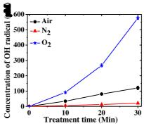
Figure 3. 24 Concentration ( $\pm$ standard deviation) of 'OH<sub>aq</sub> radical as a function of treatment time in plasma activated water for Air, N<sub>2</sub> and O<sub>2</sub> NTP (Vpp=20kV,  $\Phi$ =1.5 SLM, Height of HV electrode to water surface ranges from 7 to 8 mm, tap water: V<sub>L</sub>= 100 ml)
