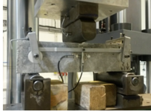
(b) Picture Three-points-flexural testing with apparatus
