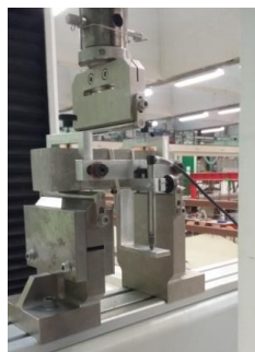
Figure 3: Device for the 3 points flexural test.
