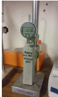
Figure 2: Device to measure shrinkage.
