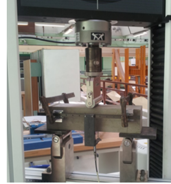
(b) Picture Three-points-flexural testing with apparatus
