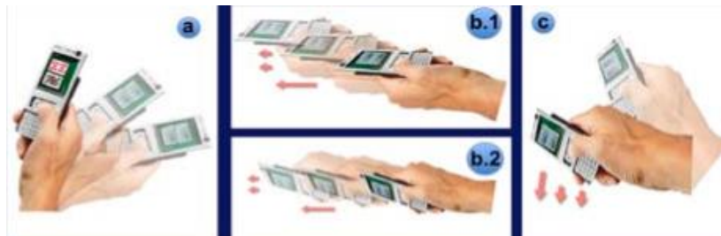
Figure 2.15: Natural gesture interactions with the mobile phone in a multi-display poker game: (a) look into cards, (b.1) fold with cards open, (b.2) fold with cards closed, and (c) check [60]
