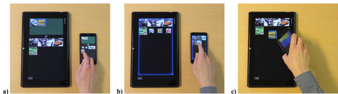
Figure 2.17: Different cross-display object movement methods: a) Tray, b) Transfer Mode, and c) Device Touch [102]
