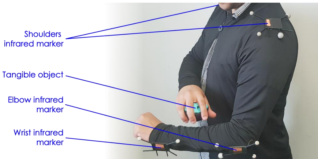
Figure 5.7: Placement of the infrared tracking markers
