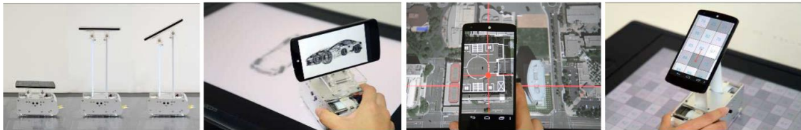
Figure 2.20: G-raff: A Tangible Block Supporting Spatial Interaction in a Tabletop Computing Environment [108]
