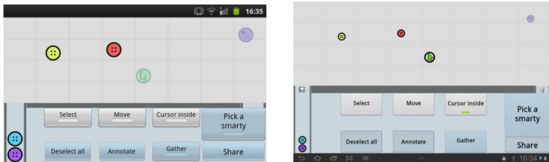
Figure 2.9: Object selection and grouping with three users. The interface running on a phone (left, middle user) and on a tablet (right, right user). Six state button widgets have been added by the application. The "Cursor Inside" action (device on the right) is attached to the active green puck, and acts as a mouse cursor confined inside a window [44].
