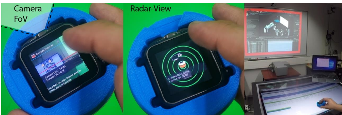
Figure 4.10: TDome's on-board camera detects displays (left) and creates a radar-view of the spatial layout (center). Then the user can select a display by Rolling + Tapping towards it (right).
