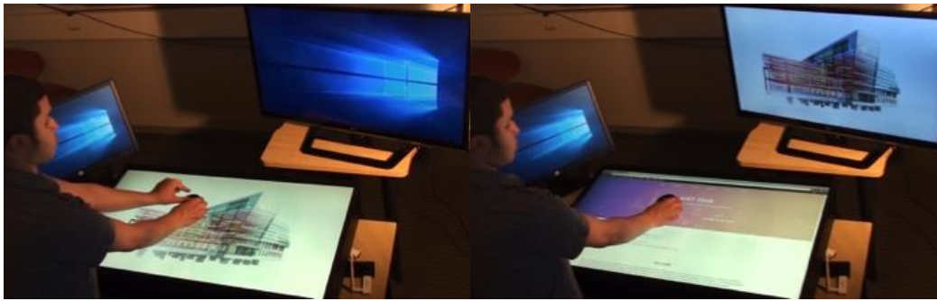
Figure 4.11: A Translation + Spread gesture sends the tabletop content (left) to a secondary display (right).
