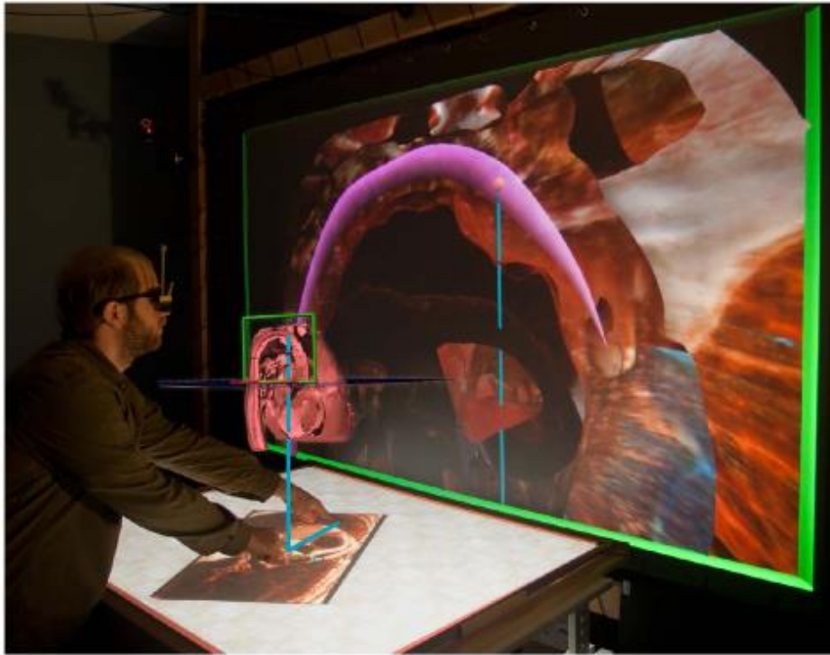
Figure 2.25: A miniature version of the 3D data appears to float in the air above the table surface. (A digital rendering is superimposed on the photograph to demonstrate the effect.) A cutting plane through the volume data is projected (like a shadow) onto the table below, where multitouch gestures are used to navigate and interrogate the data. After navigating to a useful view of these imaging data of a heart, the user is now defining a smooth 3D curve (e.g., the shape of a catheter delivery system) relative to the anatomical data set [118].
