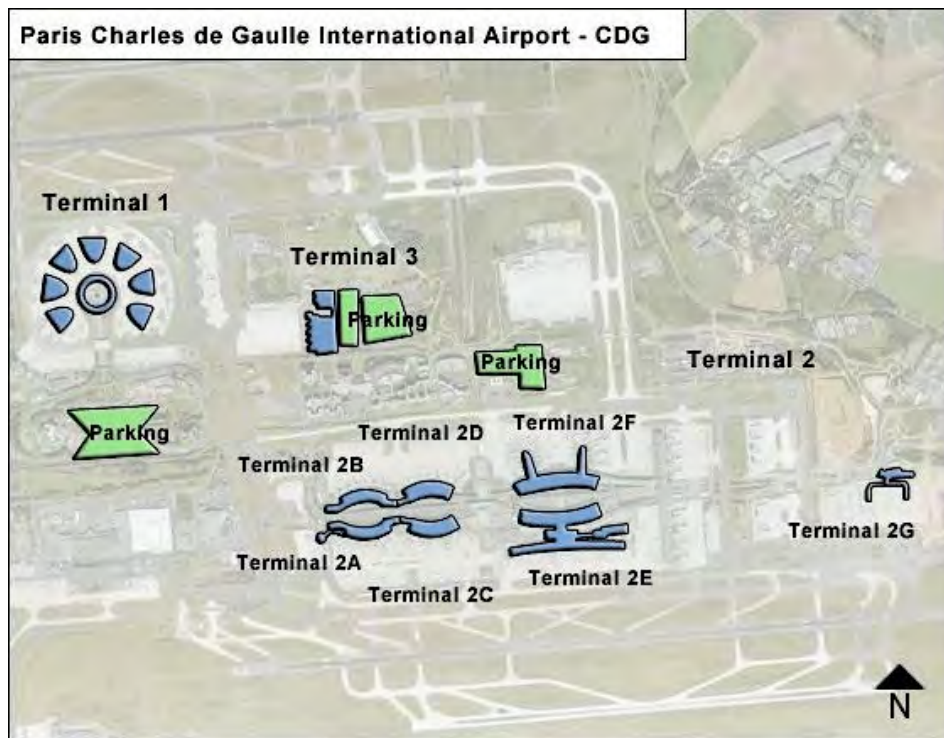
Figure 1.8: Decentralized airport terminal layout, Paris Charles de Gaulle Airport (source: https://www.ifly.com/paris-charles-de-gaulle-airport/terminal-map ).
