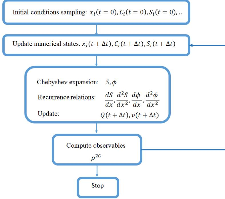
**Figure 3.1:** Schematic representation of the numerical algorithm proposed to integrate the hydrodynamic equations.
