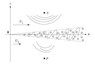
Figure 1.2 – Sketch of the experimental setup of Candel et al. [41]. S is the source position, and P is the microphone position.
