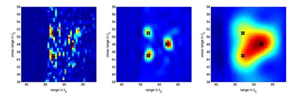
Figure 1.10 – CINT imaging function for three choices of smoothing parameters  $X_d$  and  $\Omega_d$ . The left picture is with no smoothing, the middle picture is with optimal smoothing, and the right picture is with too much smoothing. The three small reflectors are indicated with black dots. Figure is taken from [25].
