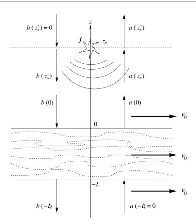
Figure 2.3 – Acoustic waves in an homogeneous flow of thickness L and flow velocity  $v_0$ . The emitting sources f are centered at some  $z_s \ge 0$ . a is the upward wave mode amplitude and b is the downward wave mode amplitude.
