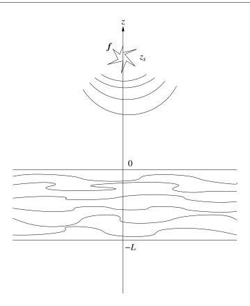
Figure 1.1 – Acoustic waves in a quiescent layered medium of typical thickness L. The emitting sources f is centered at some  $z_s \ge 0$ .
