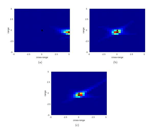
Figure 3.23 – KM passive imaging of a single source through a synthetic turbulent jet flow. Influence of the Doppler compensation coefficient  $\gamma_D$  and refraction compensation mechanism on KM imaging functional: (a) without any compensation; (b) with Doppler compensation coefficient  $\gamma_D$ ; (c) with Doppler compensation coefficient  $\gamma_D$  and refraction compensation mechanism. The source location is shown by a dot  $\bullet$ .
