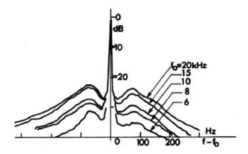
Figure 1.3 – Power spectral density of pressure fluctuations as a function of the centered frequency  $f - f_0$  for a jet velocity  $U_1 = 60$  m/s. Figure is taken from [41].
