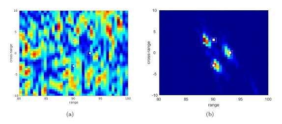
Figure 3.16 – KM active imaging in a moving medium in the configuration of Fig. 3.14 with random velocity  $\mathbf{v}_0$  and constant speed of sound  $\underline{c} = 3000$  m/s. Influence of the Doppler compensation coefficient  $\gamma_D$  on KM imaging functional: (a) without  $\gamma_D$ ; (b) with  $\gamma_D$ . The reflectors to be localized are drawn in white.
