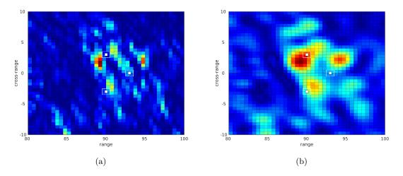
Figure 3.18 – Active imaging in a moving medium in the configuration of Fig. 3.14 with random velocity  $\mathbf{v}_0$  and random speed of sound with mean  $\underline{c} = 3000$  m/s and standard deviation  $\sigma = 3\%$ . Comparison of the KM and CINT imaging functionals for one realization of the random medium. (a) Squared KM imaging functional. (b) CINT imaging functional with  $\Omega_d = \frac{B}{15}$  and  $X_d = 0.9 \times a$ . The reflectors to be localized are drawn in white.
