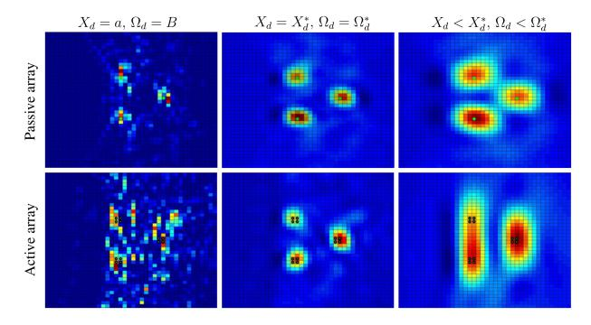
Figure 1.8 – CINT images for three realizations of a random medium with standard deviation  $\sigma = 3\%$ . Figure is taken from [24].
