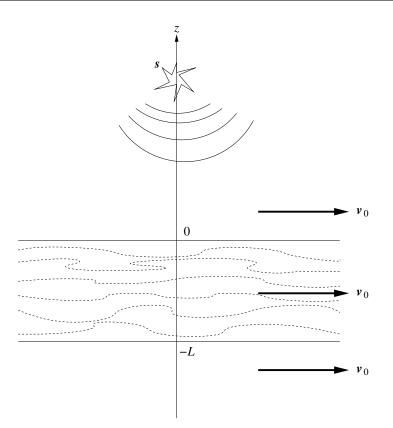
Figure 2.1 – Acoustic waves in a homogeneous flow of thickness L and flow velocity  $v_0$ .
