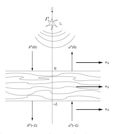
Figure 2.4 – Acoustic waves in a stratified random flow of thickness L and flow velocity  $v_0$ . The emitting sources  $f^{\varepsilon}$  are centered at some  $z_s \geq 0$ .  $a^{\varepsilon}$  is the upward wave mode amplitude and  $b^{\varepsilon}$  is the downward wave mode amplitude.
