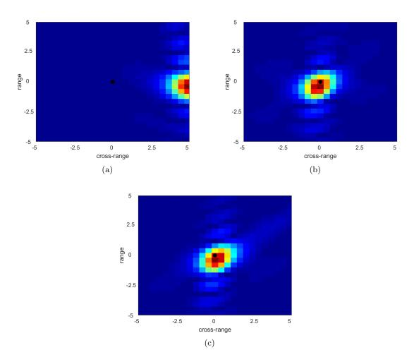
Figure 3.24 – CINT passive imaging of a single source through a synthetic turbulent jet flow. Influence of the Doppler compensation coefficient  $\gamma_D$  and refraction compensation mechanism on CINT imaging functional: (a) without any compensation; (b) with Doppler compensation coefficient  $\gamma_D$ ; (c) with Doppler compensation coefficient  $\gamma_D$  and refraction compensation mechanism. The source location is shown by a dot  $\bullet$ .
