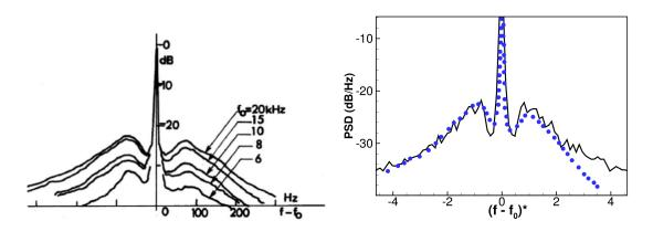
Figure 2 – Power spectral density (PSD) of the scattered pressure field at the outside of the turbulent mixing layer ( $M \approx 0.2$ ,  $Re \approx 1200$ ); experimental results after [41] (left) and numerical simulation (–) compared to experiments (•) for  $f_0 = 15$  kHz after [16] (right).
