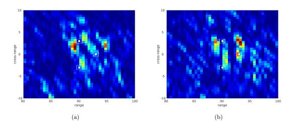
Figure 3.17 – KM active imaging in a moving medium in the configuration of Fig. 3.14 with random velocity  $\mathbf{v}_0$  and random speed of sound with mean  $\underline{c} = 3000$  m/s and standard deviation  $\sigma = 3\%$ . (a) Squared KM imaging functional for the first realization of the medium. (b) Squared KM imaging functional for the second realization of the medium. The reflectors to be localized are drawn in white.
