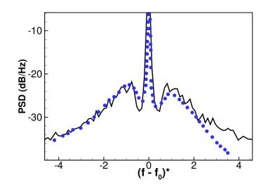
Figure 1.5 – Normalized power spectra of pressure fluctuations as functions of the normalized centered frequency  $(f - f_0)^*$ : (-) numerical simulation of [16] and (•) experimental observation of [41]. Figure taken from [16].
