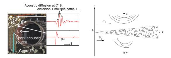
Figure 1 – Anechoic wind tunnel with open-jet test section (nozzle exit  $\emptyset = 2-3 m$ ,  $U_1 \leq 100 m/s$ ); the configuration at CEPRA 19 [50] (left) and a sketch of the experiment (right).
