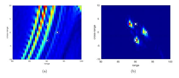
Figure 3.11 – KM active imaging in a moving medium in the configuration of Fig. 3.1 with constant velocity  $\mathbf{v}_0$  in the cross-range upward direction and constant speed of sound  $\underline{c} =$ 3000 m/s. Influence of the Doppler compensation coefficient  $\gamma_D$  on KM imaging functional: (a) without  $\gamma_D$ ; (b) with  $\gamma_D$ . The reflectors to be localized are drawn in white.
