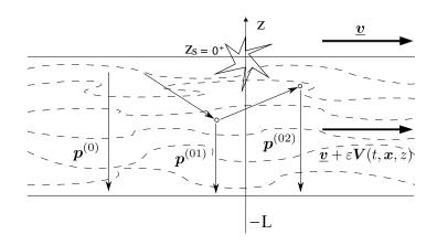
Figure 2.7 – Acoustic waves in a random flow of thickness L and average ambient flow velocity  $\underline{v}$ . Zeroth (ballistic), first, and second order perturbations in the second-order expansion of the transmitted pressure/momentum fields.
