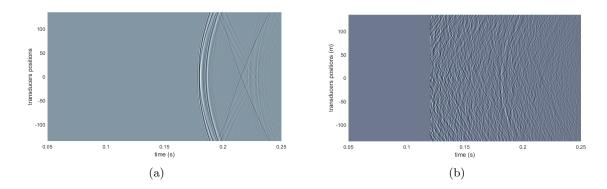
Figure 3.6 – Imaging in a motionless medium in the configuration of Fig. 3.1. (a) Time traces recorded at the receivers in the case of a constant speed of sound  $\underline{c} = 3000 \text{ m/s}$ . (b) Time traces recorded at the receivers in the case of a random speed of sound of mean  $\underline{c} = 3000 \text{ m/s}$  and standard deviation  $\sigma = 3\%$ . The horizontal axis is time (in s) and the vertical axis is the array transducer location (in units of  $\lambda_0$ ).
