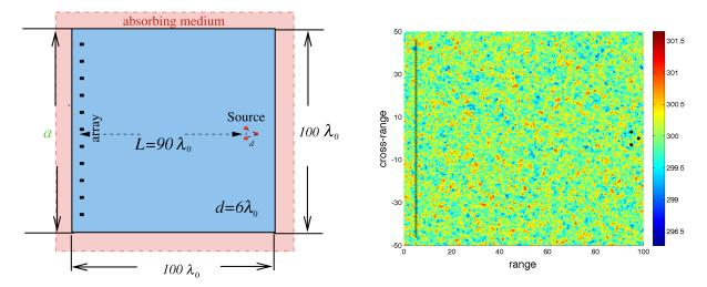
Figure 1.6 – Sketch of the computational setup used by Borcea et al. [24] (left) and typical realization of the random speed of sound  $c_0(\mathbf{r})$  (right). The dimensions of the problem are given in terms of the central wavelength  $\lambda_0$ . The locations of the sources or reflectors to be imaged are shown by dots • and the locations of the transducers are shown by crosses  $\times$ .
