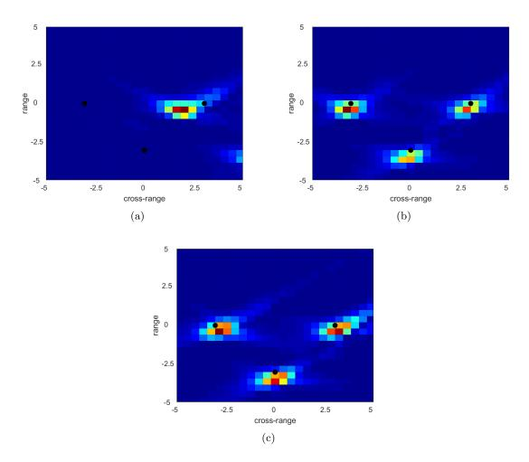
Figure 3.25 – KM passive imaging of three sources through a synthetic turbulent jet flow. Influence of the Doppler compensation coefficient  $\gamma_D$  and refraction compensation mechanism on KM imaging functional: (a) without any compensation; (b) with Doppler compensation coefficient  $\gamma_D$ ; (c) with Doppler compensation coefficient  $\gamma_D$  and refraction compensation mechanism. The source locations are shown by dots •.
