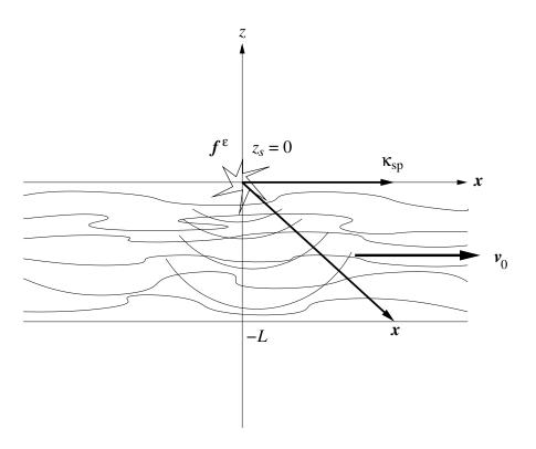
Figure 2.5 – Acoustic waves in a stratified random flow of thickness L and flow velocity  $v_0$ . The source position at  $(x_s, z_s) = 0$ , the observation point at (x, -L), and the stationary slowness vector  $\kappa_{sp}$ .
