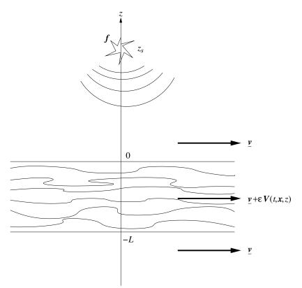
Figure 2.6 – Acoustic waves in a random flow of thickness L and average ambient flow velocity  $\underline{v}$ . The emitting sources f are centered at some  $z_s \geq 0$ .
