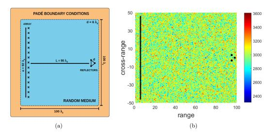
Figure 3.1 – The typical imaging configuration considered in this chapter, after [24]. Dimensions are given in terms of the central wavelength  $\lambda_0$ . (a) The locations of the sources (passive case) or reflectors (active case) to be imaged is shown by dots • and the locations of the transducers is shown by crosses ×. In the case of active imaging the central transducer is used as a source. (b) Typical realization of the random speed of sound  $c_0(\mathbf{r})$ .
