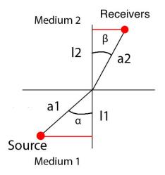
Figure 3.22 – Refracted acoustic wave at the interface between two media with speeds of sound  $c_1$  and  $c_2$ :  $\alpha$  is the angle of the incident wave,  $\beta$  is the angle of the refracted wave. The interface is taken as the mean shear layer between the first and second media in Fig. 3.19.
