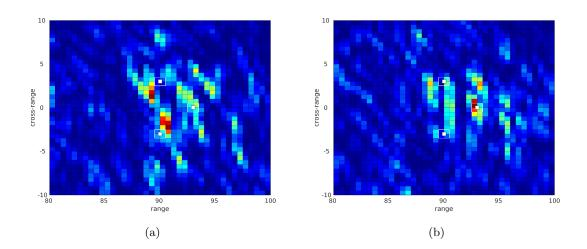
Figure 3.12 – KM active imaging in a moving medium in the configuration of Fig. 3.1 with constant velocity  $\mathbf{v}_0$  in the cross-range upward direction and random speed of sound with mean  $\underline{c} = 3000$  m/s and standard deviation  $\sigma = 3\%$ . (a) Squared KM imaging functional for the first realization of the medium. (b) Squared KM imaging functional for the second realization of the medium. The reflectors to be localized are drawn in white.
