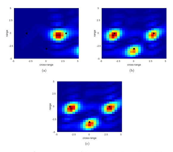
Figure 3.26 – CINT passive imaging of three sources through a synthetic turbulent jet flow. Influence of the Doppler compensation coefficient  $\gamma_D$  and refraction compensation mechanism on CINT imaging functional: (a) without any compensation; (b) with Doppler compensation coefficient  $\gamma_D$ ; (c) with Doppler compensation coefficient  $\gamma_D$  and refraction compensation mechanism. The source locations are shown by dots  $\bullet$ .
