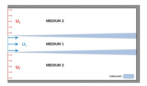
Figure 3.19 – Synthetic jet flow configuration:  $\square$  non-reflection Padé boundary conditions; \_\_\_\_\_\_ jet inflow boundary condition for the central zone with  $U_1 = 100 \text{ m/s}$ ; \_\_\_\_\_\_ jet inflow boundary condition outside the central zone with  $U_2 = 50 \text{ m/s}$ .
