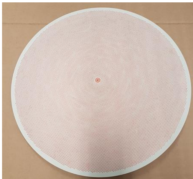
Figure 87: Manufactured four-beams metasurface (printed on a substrate ROGERS TMM6).
