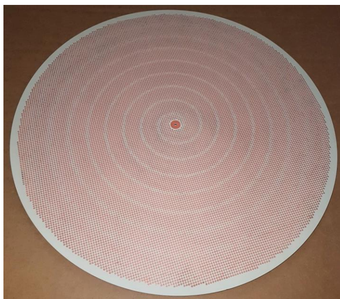
Figure 80: Manufactured broadside RHCP metasurface (printed on a substrate ROGERS TMM6).
