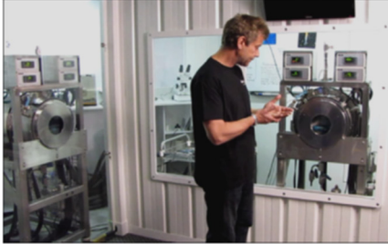
Volume 16.5L – pressure up to 20MPa – temperature 2-40°C – flow rates up to 10L/h
