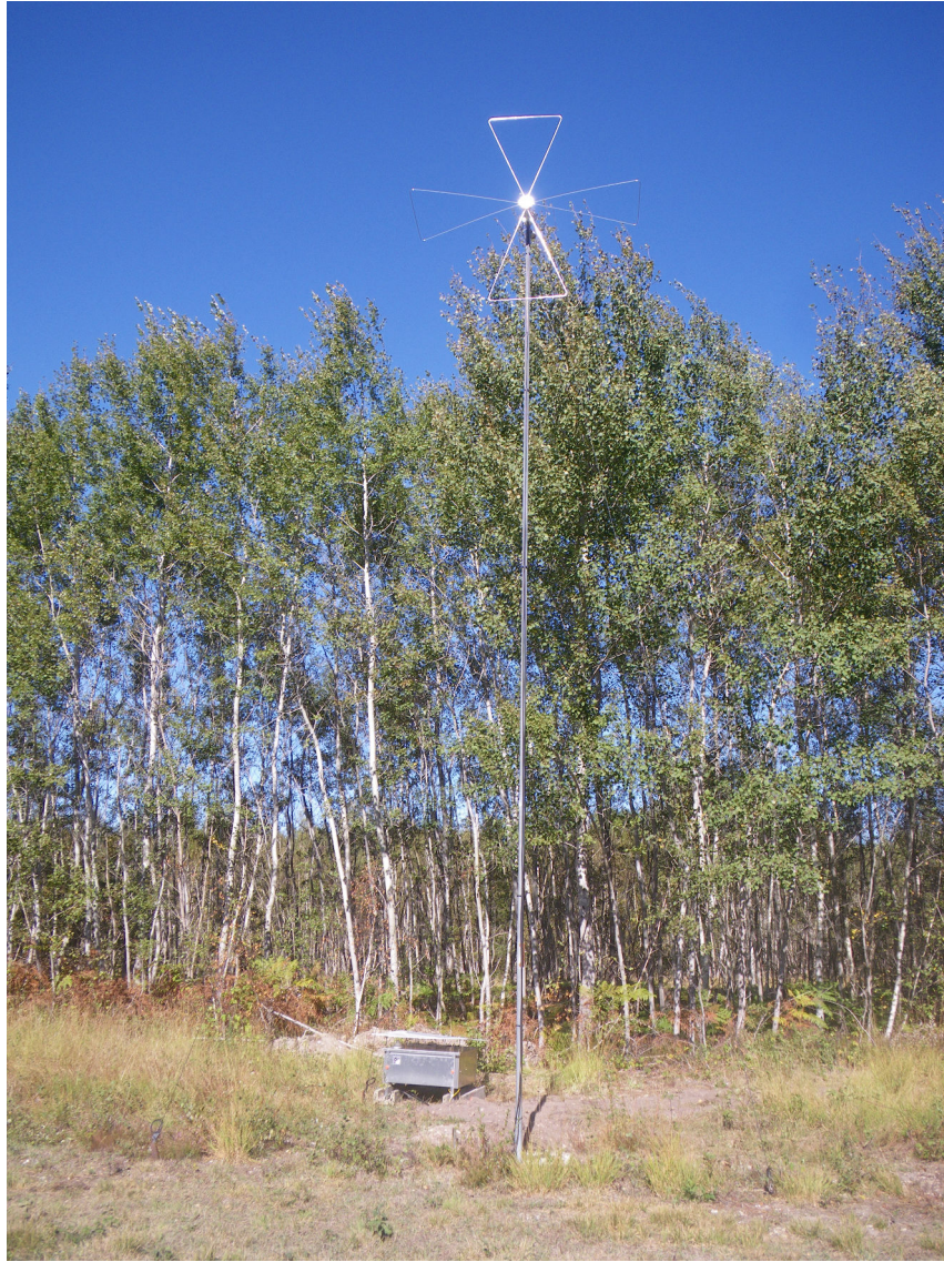
Figure 4.21 – Photography of a LF antenna.
