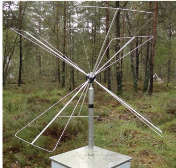
Figure 4.16 – Photography of the three-fold antenna. Each Butterfly antenna is rotated twice to form a direct trihedron inclined by 45^\circ . See [160] for more details.
