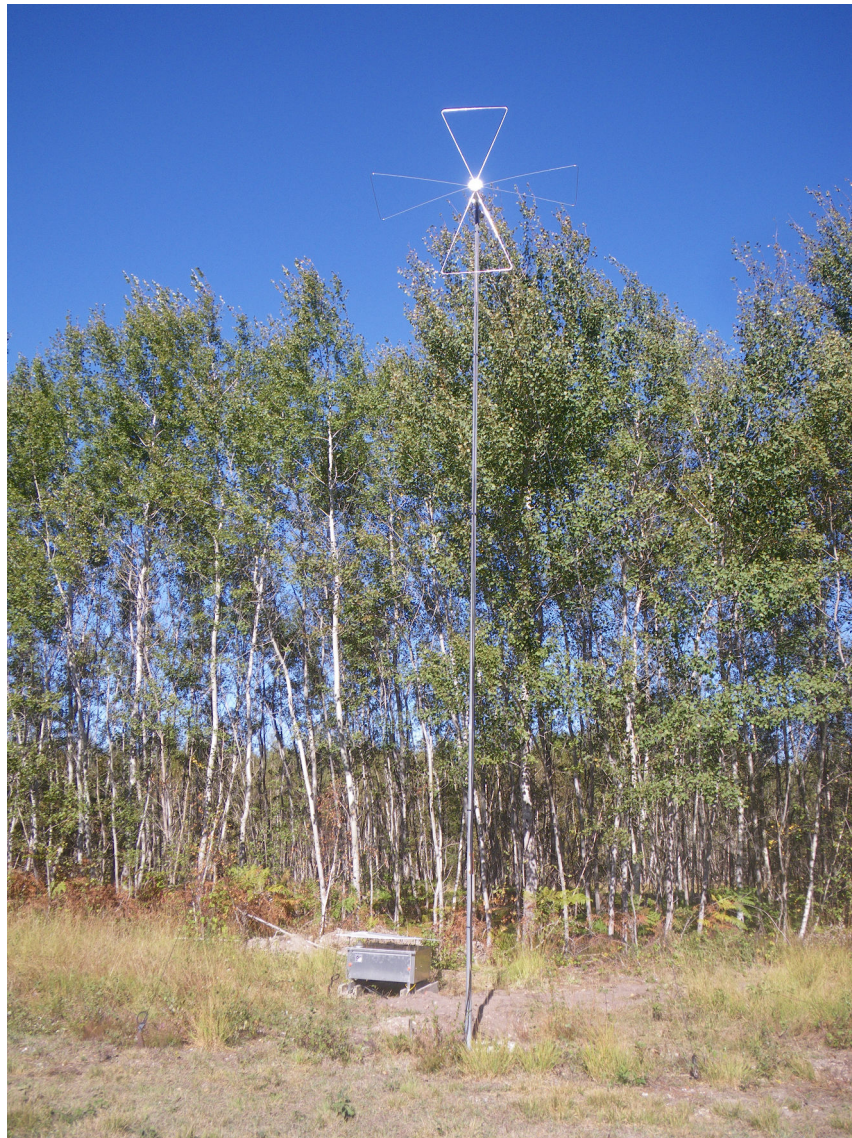
Figure 4.21 – Photography of a LF antenna.
