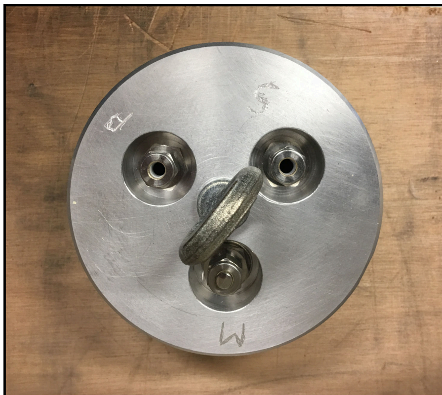
Figure B.3 – Aluminum piece sealing the rubber tube. The piece is pierced for tubing connections. Three mounted airtight tube fittings are visible.
