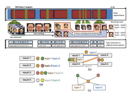
Fig. 3.1 (Top) Indexing each video segment: closed captions-based segmentation, face tracking, and keyword extraction. (Bottom) Abstraction of the search results; (a) indexed video segments; (b) the multiplex network of results; (c) the associated *LIN*.
