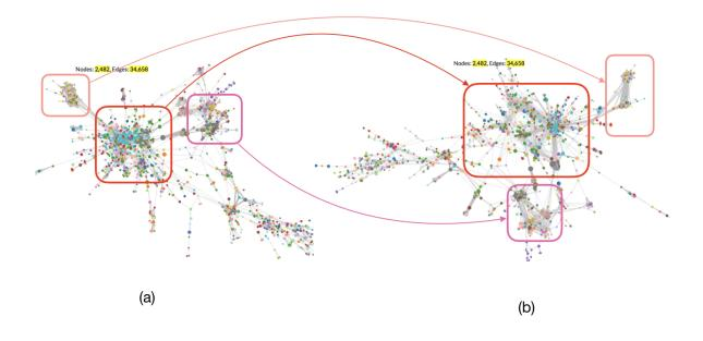
the algorithm. It can be seen that there are very few overlapping of the nodes from different communities. The different colors of hull not only prove the effectiveness of our modification of the force layout algorithm, but also help the user's intuitive understanding and selection of different communities.
