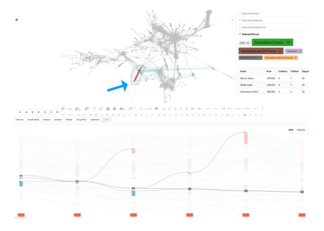
The sankey graph is a supplement to the original dynamic node-link graph. The node-link is a spatial overlay of the dynamic graph time, and the sankey graph is a spatial extension of the dynamic time. The combination of the two is more conducive to studying the evolution of some members or groups over time.
