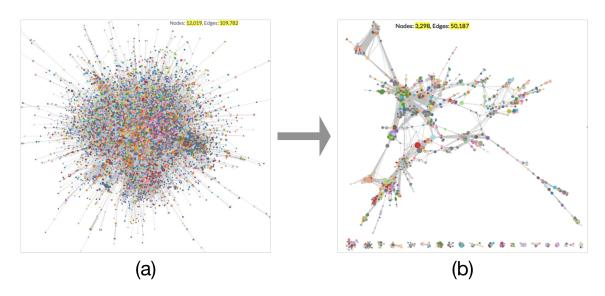
Right after building the network from participation data, its structure remains very complicated and hard to read due to the density of nodes and links. As shown in the figure 4.12 (a), it is difficult to intuitively observe the characteristics of the network. Extracting groups directly from such a complex network often returns unpractical results.
