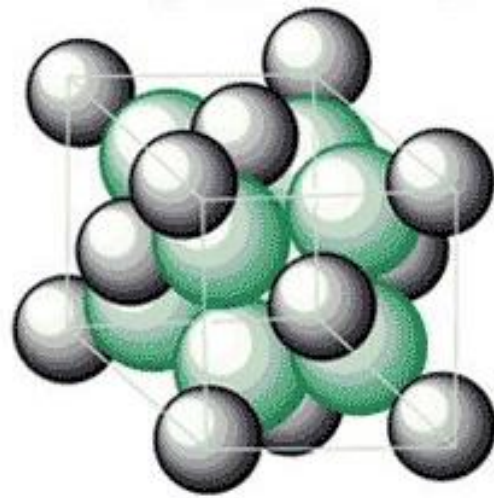
Figure 2-15 : Unit cell of \text{CaF}_2 . The black balls represent the Ca atoms, and the green balls represent the F atoms [83].
