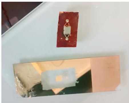
Figure IV.14 – Picture of a PDMS microfluidic device which detached from the silica sample because of a sudden pressure jump in the channels. It can be seen that the interface which give way is the one between sol-gel silica and gold.
