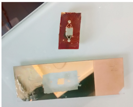
Figure IV.14 – Picture of a PDMS microfluidic device which detached from the silica sample because of a sudden pressure jump in the channels. It can be seen that the interface which give way is the one between sol-gel silica and gold.
