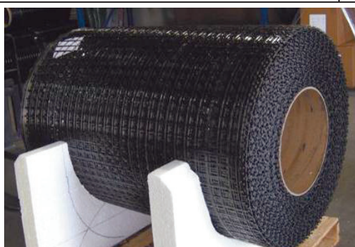
(a) Rouleau de textile GC1 (2.4m x 411.5m)
