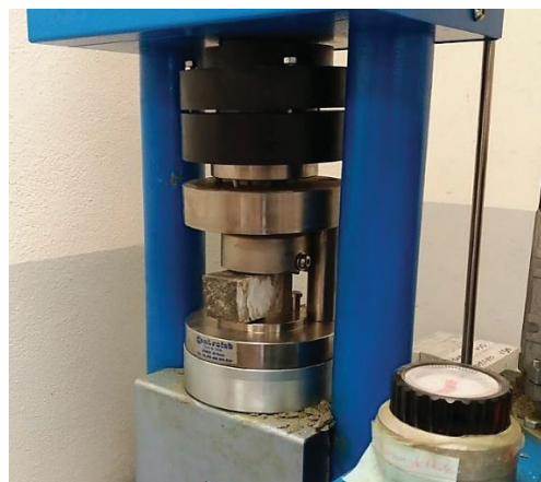
(b) Essai de compression
