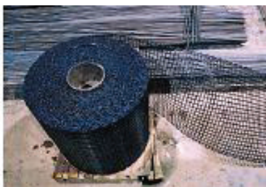
(a) Rouleau de textile GC3 (1.2m x 411.5m)
