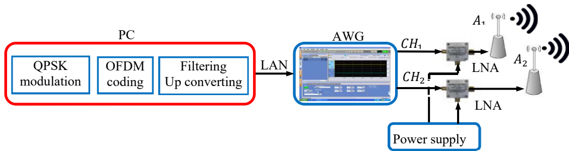
Figure 4-21: The transmitter block diagram
