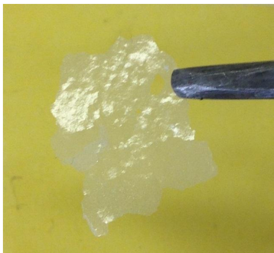
Figure 14: The white film (complex) of N -allyl- N -(4-methoxyphenyl)acrylamide with \beta -CD.
