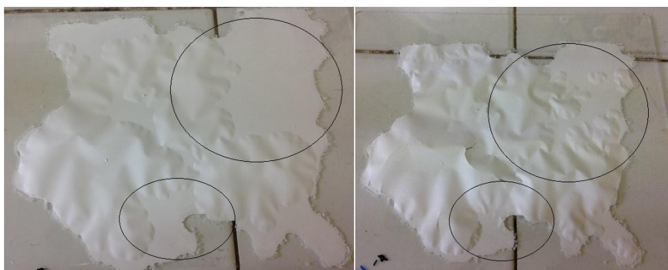
Figure 45: Photo of 1/1 \beta -CD/azepinone 8 complex film (experiment F ) as it detaches itself from the glass plate after 2 days (left), and after 4 days (right).
