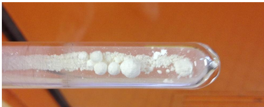
Figure 38: Small balls of \beta -CD/azepinone 8 formed when the complex was irradiated in powder form in a rotating quartz tube.
