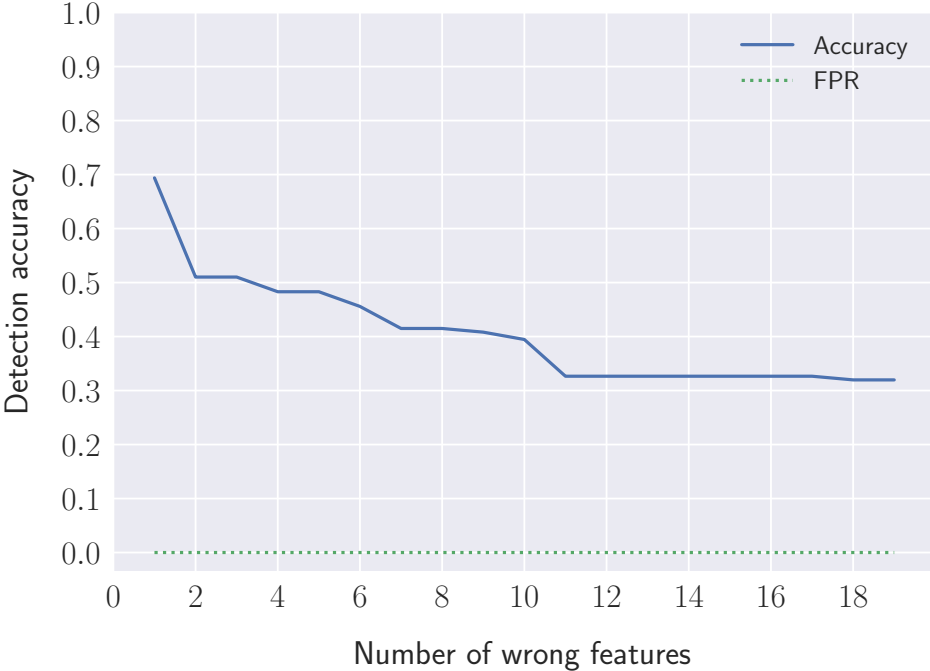
Figure 4.5 Detection accuracy and false positive rate of the browser feature test for different values of N_e (number of wrong features).
