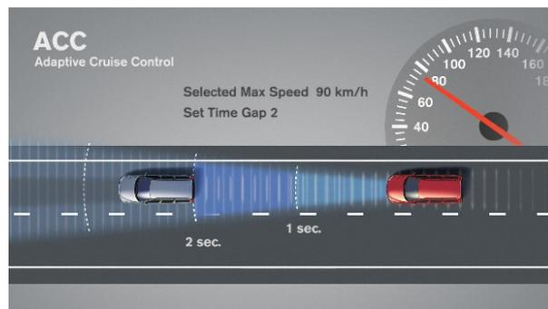
FIGURE 1.14 – Fonction ACC réglable [Source : [http://crankydriver.com/blog/images/Reports/ADAS/acc\\_gap.jpg](http://crankydriver.com/blog/images/Reports/ADAS/acc_gap.jpg)]
