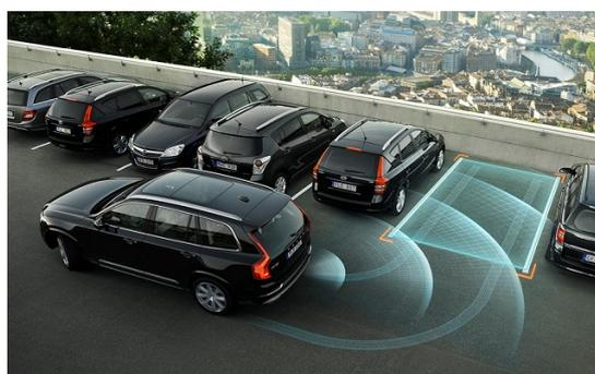
FIGURE 1.16 – Fonction de stationnement automatique [Source : [http://volvo.custhelp.com/app/answers/detail/a\\_id/9559/~park-assist-pilot](http://volvo.custhelp.com/app/answers/detail/a_id/9559/~park-assist-pilot)]
