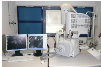
Figure II. 15 : MEB Quanta 400 FEG de FEI du LCTS
