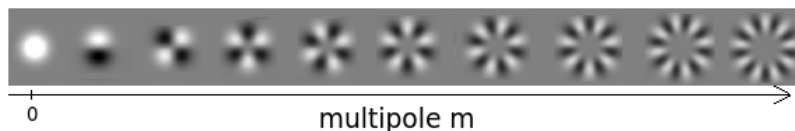
Figure 3.1 – An illustration of the multipolar decomposition as a function of order m . For example at the order m = 0 , the matter distribution is isotropic (monopole), whereas the order m = 1 is the dipole, m = 2 the quadrupole, etc.
