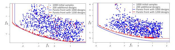
Figure 3.6: Observations and estimated Pareto front (obtained by means of an Evolutionary Algorithm applied to the predictor) of the MetaNACA fitted to the 1000 first points (blue), or to all 1200 points (red). Left d = 8, right d = 22.
