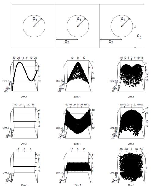
Figure 6.2: Example 6.1: three first eigencomponents of the  $\boldsymbol{\alpha}^{(i)}$ 's for three parametric test cases (columns) with low effective dimension equal to 1 (left), 2 (center) and 3 (right). The rows correspond to different  $\phi$ 's which are the characteristic function (top), the signed distance to the contour (middle) and the discretization of the contour (bottom).
