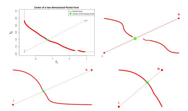
Figure 4.8: Examples of two-dimensional Pareto fronts and their center. Notice that on the bottom, the left and the right fronts are the same, except that the left is substantially extended in the x direction. However, the center has been only slightly modified.
