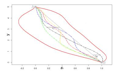
Figure 6.22: Example 6.5: a straight line joining two points, modified by the perturbations  $r_j$  to approximate a curve. Gray: the line joining A and B. Blue, red, yellow and green curve: examples of lines with regular  $r_j$  perturbations. Red envelope: boundaries for the  $r_j$ 's.
