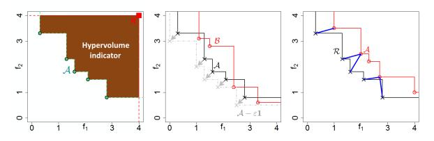
Figure 2.10: Left: hypervolume indicator (brown area) of a non-dominated set  $\mathcal{A}$ . Center: additive  $\varepsilon$ -indicator of  $\mathcal{A}$  (black set) with respect to  $\mathcal{B}$  (red set). Right: IGD indicator of  $\mathcal{A}$  (red set), with respect to the reference set  $\mathcal{R}$  (black set).
