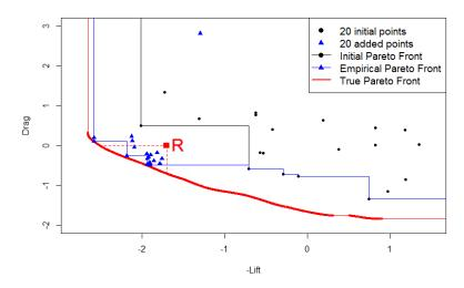
Figure 4.13: Optimization run targeting an off-centered part of the Pareto front through **R**. After 20 iterations, the Pareto front approximation has been improved in the left part, as specified by **R**. The successive reference points  $\hat{\mathbf{R}}$  used by mEI are shown in Figure 4.14.
