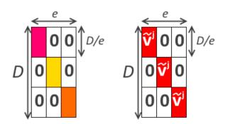
Figure 6.43: Modification of the  $\mathbf{V}^{(j)}$  submatrix in an example with e = 3 elements. Left: the original  $\mathbf{V}^{(j)}$  matrix obtained by eigendecomposition of the sparse  $\mathbf{C}_{\Phi}$  matrix. Right: modified  $\mathbf{V}^{(j)}$  matrix. The average of the pink, yellow and orange vector in the left matrix is  $\tilde{\mathbf{v}}^{j}$ , which is employed in  $\mathbf{V}^{(j)}$  such that these e vectors apply the same transformation to their corresponding element.
