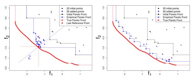
Figure 4.17: Bi-objective optimization with the **C**-mEI algorithm (left). The initial approximation (black) has mainly been improved around the center. Compared with a standard EHI (right), the proposed methodology achieves convergence to the central part of the front. EHI considers more compromises between objectives, but cannot converge within the given budget.
