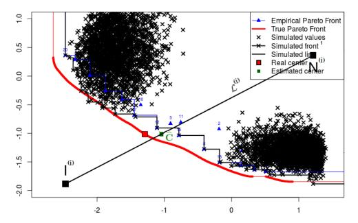
Figure 4.12: One (among the  $n_{sim}$ ) GP simulation targeting the extreme points of the Pareto front to enhance the estimation of I and N. The projection of the closest non-dominated point to  $\mathcal{L}$  on it is the estimated center (in green). The real center (in red) lies close to the estimated center and to the estimated Ideal-Nadir line.
