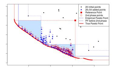
Figure 4.23: Final approximation of the Pareto front by C-EHI with, as a red square, the reference point of the second phase chosen as a solution to problem (4.9),  $\mathbf{R} = \mathbf{R}^*$ . The objective values added during the second phase of the algorithm are circled in red. Compared to the initial front obtained when searching for the center (other blue triangles), the final approximation front is expanded as highlighted by the blue hypervolume.
