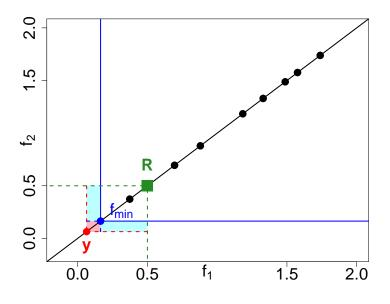
Figure 4.3: *m*-degenerate problem (4.3). The improvement brought by  $\mathbf{y} \in Y$  is measured by the improvement over  $\mathbf{f}_{\min}$  (light red area), but also by a term depending on  $\mathbf{R}$  (light blue area).
