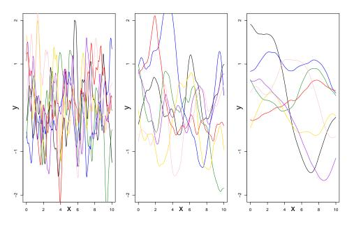
Figure 2.1: Effect of changing the length-scale of the GP. Left:  $\theta = 0.3$ . Center:  $\theta = 1$ . Right:  $\theta = 3$ .
