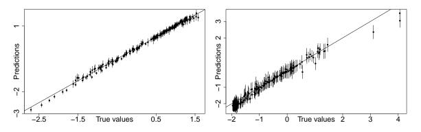
Figure 3.8: Evaluation of the "initial MetaNACA 22" built over the first 1000 points, on the 200 additional designs (to be further incorporated in this model). Predicted values and 95% confidence bounds are plotted against the true value of these designs. Left: negative lift, right: drag.
