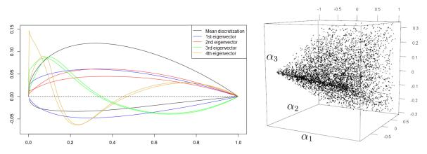
Figure 6.24: NACA airfoil with d = 3 parameters. Left: mean shape and 4 first eigenshapes (black, blue, red, green, yellow). Right: three first eigencomponents  $(\alpha_1, \alpha_2, \alpha_3)$  of the  $\mathcal{A}_N$  manifold.
