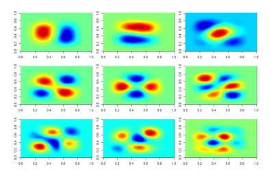
Figure 6.8: Example 6.1, circle with d = 3 parameters, 9 first eigenvectors (left to right and top to bottom) when  $\phi$  = characteristic function.
