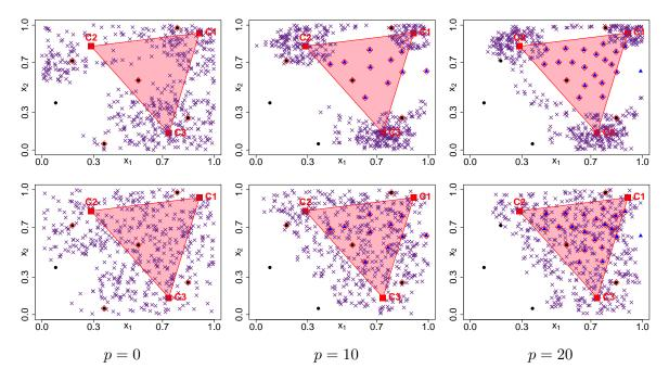
Figure D.8: **x**'s where conditional GP simulations are performed (purple crosses) for estimating **I** and **N** (top row) and for being non-dominated (bottom row). Left to right: after 0, 10, or 20 additional function evaluations. The centers of the  $f_j(\cdot)$ 's are represented by red squares, black dots are the initial DoE points, and the blue triangles correspond to sequential infills. Non-dominated solutions are surrounded by a red diamond.
