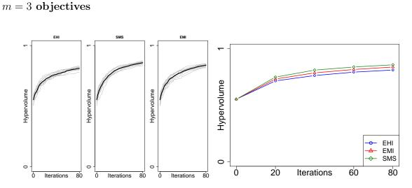
Figure A.4: Evolution of the hypervolume indicator in the remaining budget for the different infill criteria, for d = 8 and n = 20 (budget = 100).
