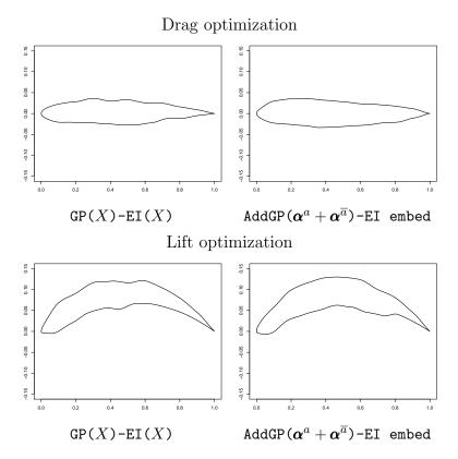
Figure 6.38: Airfoils found by the compared optimization algorithms. Top: drag minimization, bottom: lift maximization. Left: optimization with the GP(X)-EI(X) algorithm, right: optimization with the  $AddGP(\alpha^a + \alpha^{\overline{a}})-EI$  embed algorithm.
