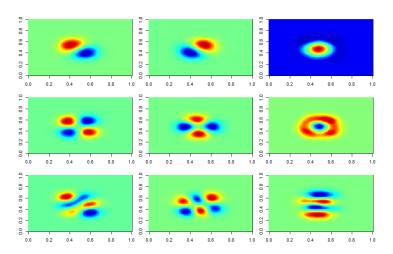
Figure 6.13: Example 6.2, over-parameterized circle with d = 39 parameters, 9 first eigenvectors (left to right and top to bottom) when  $\phi =$  characteristic function.
