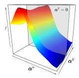
Figure 6.29: Example of a function that primarily varies along the  $\boldsymbol{\alpha}^{a}$  direction, and secondarily along  $\boldsymbol{\alpha}^{\overline{a}}$ . If  $\boldsymbol{\alpha}^{\overline{a}}$  is omitted, one implicitly considers the restriction of  $f(\cdot)$  to the gray plane where  $\boldsymbol{\alpha}^{\overline{a}} = \mathbf{0}$ .
