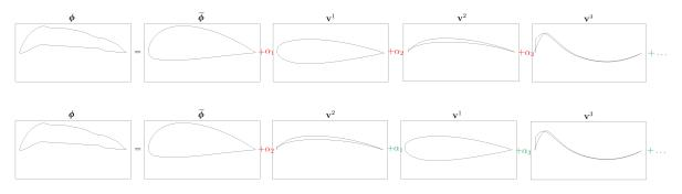
Figure 6.28: Variable selection on the NACA 22 benchmark by penalized maximum likelihood. For the drag (top), the three first eigenshapes that act on the shape, hence on its drag, are selected (red coefficients). For the lift, only the second eigencomponent  $(\mathbf{v}^2)$  is selected (bottom). Indeed  $\mathbf{v}^2$  modifies the camber of the airfoil, hence it plays a major role on the lift. The other eigenbasis vectors (green coefficients) are estimated to be less influential on y.
