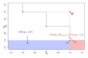
Figure C.7: Areas leading to a new first component (j = 1) of **N**. A point in the red zone (larger than the first extreme point,  $\overline{\boldsymbol{\nu}}^1$ , in the first objective and non-dominated) or in the blue zone (dominating  $\overline{\boldsymbol{\nu}}^1$ ) becomes the new (first) extreme point, and therefore induces a modification of **N**.
