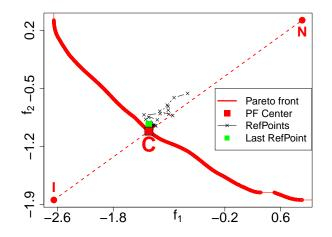
Figure 4.18: Reference points  $\mathbf{R}$  successively used for directing the search during the C-mEI run of Figure 4.17. They lie close to the dashed Ideal-Nadir line (IN) and lead the algorithm to the center of the Pareto front (C).
