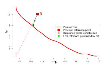
Figure 4.14: Reference points  $\widehat{\mathbf{R}}$  successively used for directing the search during the run of Figure 4.13, where  $\mathbf{R} = (-1.7, 0)^{\top}$  is provided.  $\widehat{\mathbf{R}}$  adjusts to the current approximation front to direct the algorithm in a region of the Pareto front that dominates  $\mathbf{R}$ .
