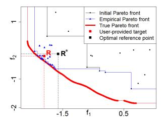
Figure 4.30: Typical run of the R-EHI algorithm with a budget of 20+20 function evaluations, when the target **R** (red square) is provided. Remark that after convergence detection, the eventually chosen  $\mathbf{R}^*$  (black square, see Section 4.6) targets a wider part of  $\mathcal{P}_{\mathcal{Y}}$  than the initially supplied **R** because accurate enough convergence has been forecasted for the remaining iterations inside  $\mathcal{I}_{\mathbf{R}^*}$ .
