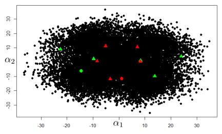
Figure 6.46: Two  $\boldsymbol{\alpha}$ 's (red and green circle) and their discretizations in the  $\mathcal{V}$  basis which correspond to an identical shape (triangle). Symmetries cannot be retrieved directly in  $\mathcal{V}$  (test case with three circles).
