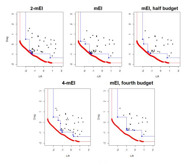
Figure 5.5: Top: example run using 2-mEI (left) with  $2 \times 10$  additional designs, and mEI with 20 (center) and 10 (right) iterations. Bottom: example run using 4-mEI (left) with  $4 \times 5$  additional designs, and mEI with 5 iterations (right). At a fixed wall-clock time, q-mEI converges more accurately to the center than mEI. At a fixed number of evaluations, the degradation is small.
