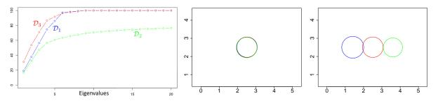
Figure 6.40: Eigendecomposition for different multi-element mappings, 3 circles test case. Left: PCA eigenvalues cumulative sum (in %). Middle: mean shape  $\overline{\phi}$  when  $\phi = \mathcal{D}_1$ . Right: mean shape  $\overline{\phi}$  when  $\phi = \mathcal{D}_3$ .
