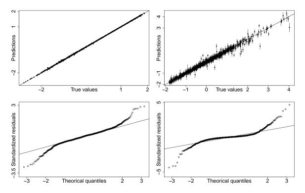
Figure 3.7: Leave-one-out predictions and 95% confidence interval (top) and QQ-plots (bottom) to validate the MetaNACA 8. Left: negative lift, right: drag.
