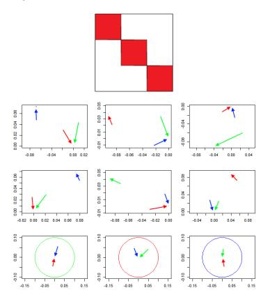
Figure 6.42: Top: shape of the correlation matrix  $\mathbf{C}_{\Phi}$  when enforcing a null correlation (white) between nodes of distinct elements. Bottom: 9 eigenvectors of  $\mathbf{C}_{\Phi}$ . Since correlations between different circles have been removed, each  $\mathbf{v}^{j}$  operates on one element.
