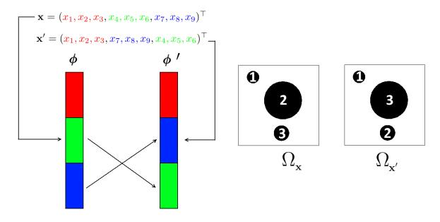
Figure 6.39: Example of permutation of  $\mathbf{x}$  under which the shapes  $\Omega_{\mathbf{x}}$  and  $\Omega_{\mathbf{x}'}$  are invariant. However, the shape representations  $\boldsymbol{\phi}$  and  $\boldsymbol{\phi}'$  yielded by  $\mathcal{D}_1$  are different.
