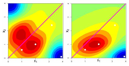
Figure 6.45: Left: example of kriging with invariance with respect to the first bisector (purple line). Right: GP with standard kernel. Predictions are enhanced by providing the symmetry information.
