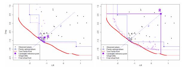
Figure 4.21: Virtual infills (purple circles) obtained by sequentially maximizing  $\text{EHI}(\cdot; \mathbf{R})$  b times, for two different reference points (purple squares). The shape and sampling density of the final virtual front depends on  $\mathbf{R}$ .
