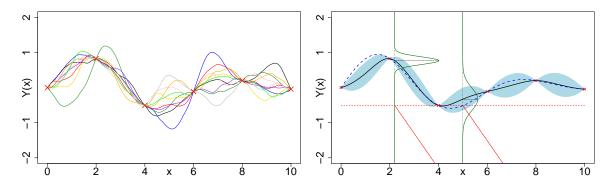
Figure 2.5: Left: samples of the conditional GP which interpolate the data. Right: kriging mean predictor (black curve) and  $[\hat{y}(x) - s(x), \hat{y}(x) + s(x)]$  confidence interval (light blue envelope). The dotted blue line is the true function. The distribution at two untested designs x = 2.2 and x = 5,  $Y(2.2) \sim \mathcal{N}(\hat{y}(2.2), s^2(2.2))$ ,  $Y(5) \sim \mathcal{N}(\hat{y}(5), s^2(5))$ , is the vertical green density.
