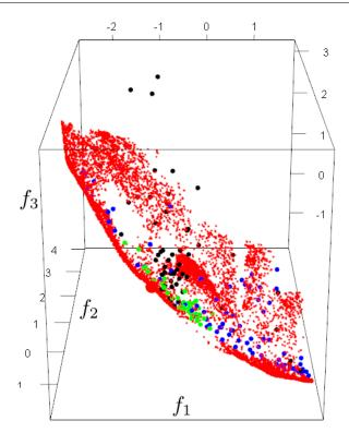
Figure 4.25: Typical C-EHI (green points) and EHI (blue points) runs on the MetaNACA problem with m = 3 objectives. Black dots are evaluations of the initial DoE. The true Pareto front (red) is attained at its center by C-EHI while it is approximated globally yet less accurately by EHI.
