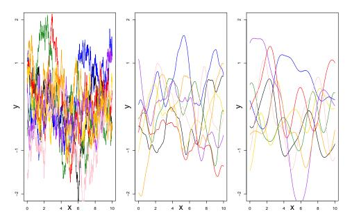
Figure 2.3: Effect of changing the kernel of the GP. Left: exponential kernel. Center: Matérn 5/2 kernel. Right: squared-exponential kernel.
