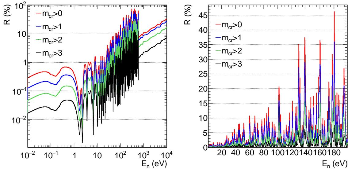
Figure 5.4: Ratio of expected scattered neutron and  $^{233}\text{U}(n,\gamma)$  events depending on the neutron energy and crystal multiplicity for events with  $2.5\text{ MeV} < E_{Sum} < 7\text{ MeV}$ .
