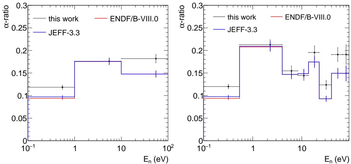
Figure 6.13: Comparison of the average values of the experimental, ENDF/B-VIII.0 and JEFF-3.3  $^{233}\text{U}$   $\alpha$ -ratio for neutron energy decades (left) and neutron energy intervals according to the 33 group energy structure of the WPEC Subgroup 33 (SG33) [120] (right). The corresponding values are summarized in Table 6.2. No dead time corrections have been applied.
