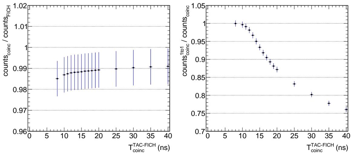
Figure 4.32: Fraction of found coincidences with respect to the total number of fission events in the FICH for different TAC-FICH coincidence windows  $T_{coinc}^{TAC-FICH}$  (left). Fraction of events where exactly one TAC event is found for one FICH event with respect to all found coincidences (right). Both for events with  $amp > 3000$  adc units and  $1.6 \text{ eV} < E_n < 1.9 \text{ eV}$ .
