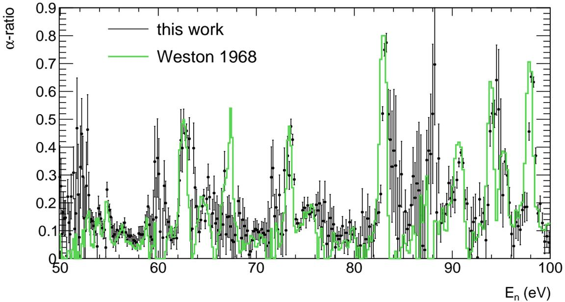
Figure 6.19: Comparison of the point wise experimental  $^{233}\text{U}$   $\alpha$ -ratio from this work and from the experimental data sets from Weston in the neutron energy region from  $50\text{ eV} < E_n < 100\text{ eV}$ . No dead time corrections have been applied.
