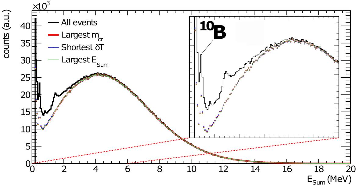
Figure 4.31: Comparison of the different event selection algorithms using either largest  $E_{sum}$ , largest  $m_{cr}$  or smallest  $\delta T^{TAC-FICH}$  as primary criteria. In the zoom in the region for  $E_{sum} < 6$  MeV the suppression of the 480 keV  $\gamma$ -ray emitted in the  $^{10}\text{B}(n,\alpha)$  reaction and the 1435 keV  $\gamma$ -ray from inelastic scattering of fission neutrons on  $^{138}\text{Ba}$  can be observed.
