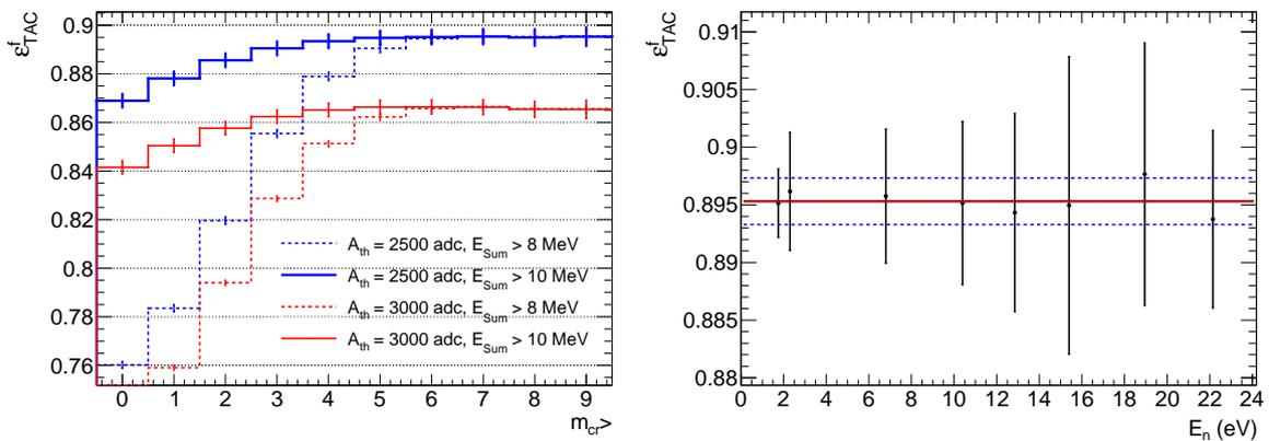
Figure 5.16: Fission tagging efficiency  $\varepsilon_{TAC}^f$  as a function of the crystal multiplicity and sum energy for two different amplitude thresholds  $A_{th}$  in the neutron energy interval from 1.6 eV to 1.9 eV (left). Fission tagging efficiency calculated in several neutron resonances for  $A_{th} = 2500$  adc units,  $m_{cr} > 6$  and  $E_{Sum} > 10$  MeV, their average (red line) and the associated error of the average (blue dashed lines) (right).
