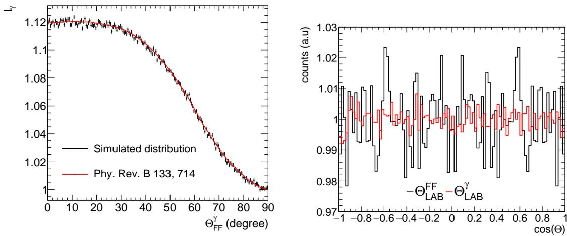
Figure 4.46: Simulated distributions of the emission angles for  $\gamma$ -rays of the PFG cascade in the fission fragment frame of reference [106] (left) and the  $\gamma$ -ray and fission fragment emission angle in the laboratory system.
