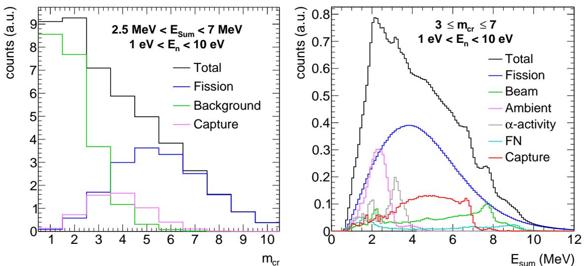
Figure 6.1: Crystal multiplicity distribution of TAC events with  $2.5 \text{ MeV} < E_{sum} < 7 \text{ MeV}$  for the different contributions to the total measured spectrum (left). Sum energy distribution in the TAC corresponding to their source for events with  $3 \leq m_{cr} \leq 7$  (right).
