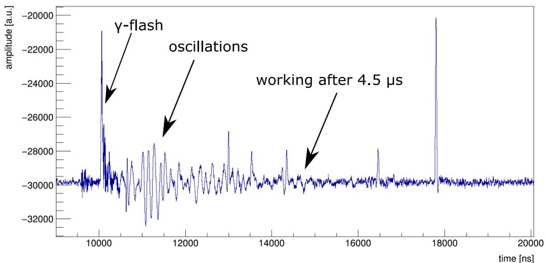
Figure 3.17: Reponse of the FICH to the  $\gamma$ -flash. A time-of-flight of 4.5  $\mu\text{s}$  corresponds to a neutron energy of roughly 7 MeV.
