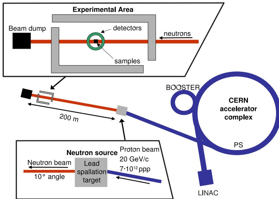
Figure 3.1: Schematical overview of the n\_TOF facility at CERN, only showing experimental area 1, picture taken from [65].
