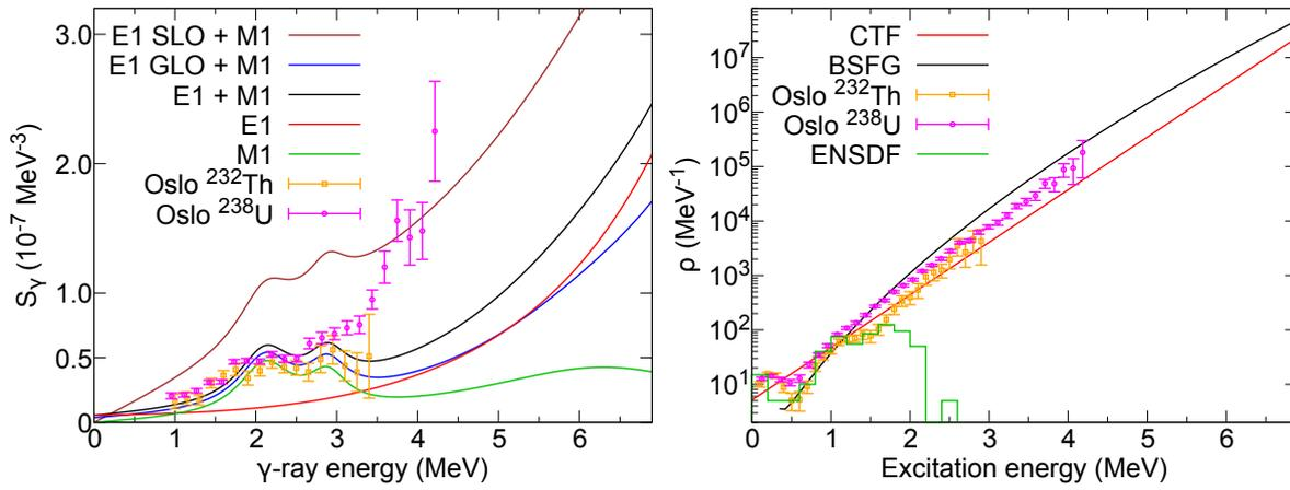
Figure 5.21: Photon strength function used to reproduce the experimental  $^{234}\text{U}$   $\gamma$ -ray decay (black, red, green) [109] compared to suggested model as defined in the RIPL-3 data base [110] (brown and blue lines, SLO/GLO in the legend) and other data sets from the Oslo group (left). Two level density models compared to experimental data from the Oslo group and experimental level counting from ENSDF (right), for detailed explanation see section 5.4.1.
