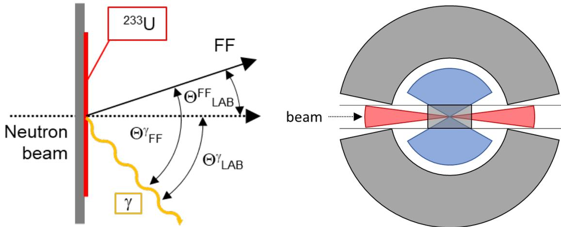
Figure 4.47: Definition of the angles in the simulations (left). Illustration of the TAC and FICH detection efficiencies -  $\varepsilon_{TAC}$  is high (low) in the blue (red) region;  $\varepsilon_{FICH}$  is high (low) in the red (blue) region (right).
