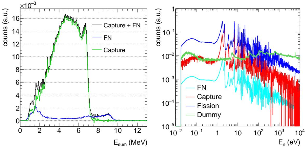
Figure 5.13: The shape of the fission neutron spectra is scaled to the remaining background contribution above 7 MeV in the capture response for the strong capture resonance at 2.2-2.4 eV and  $m_{cr} > 2$  (left). The contributions to the TAC response as a function of the neutron energy (right).
