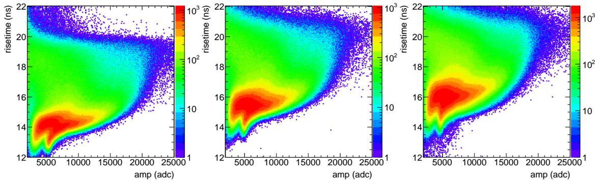
Figure 4.21: Rise time versus amplitude of FICH signals from the two single  $^{233}\text{U}$  deposit FICH channels 4 (left) and 8 (middle) and FICH channel 7 (right) reading signals from two ionization cells. For short rise times (i.e.  $\cos\theta_{LAB}^{FF} \approx 1$ ) the light and heavy fission fragment peaks become visible.
