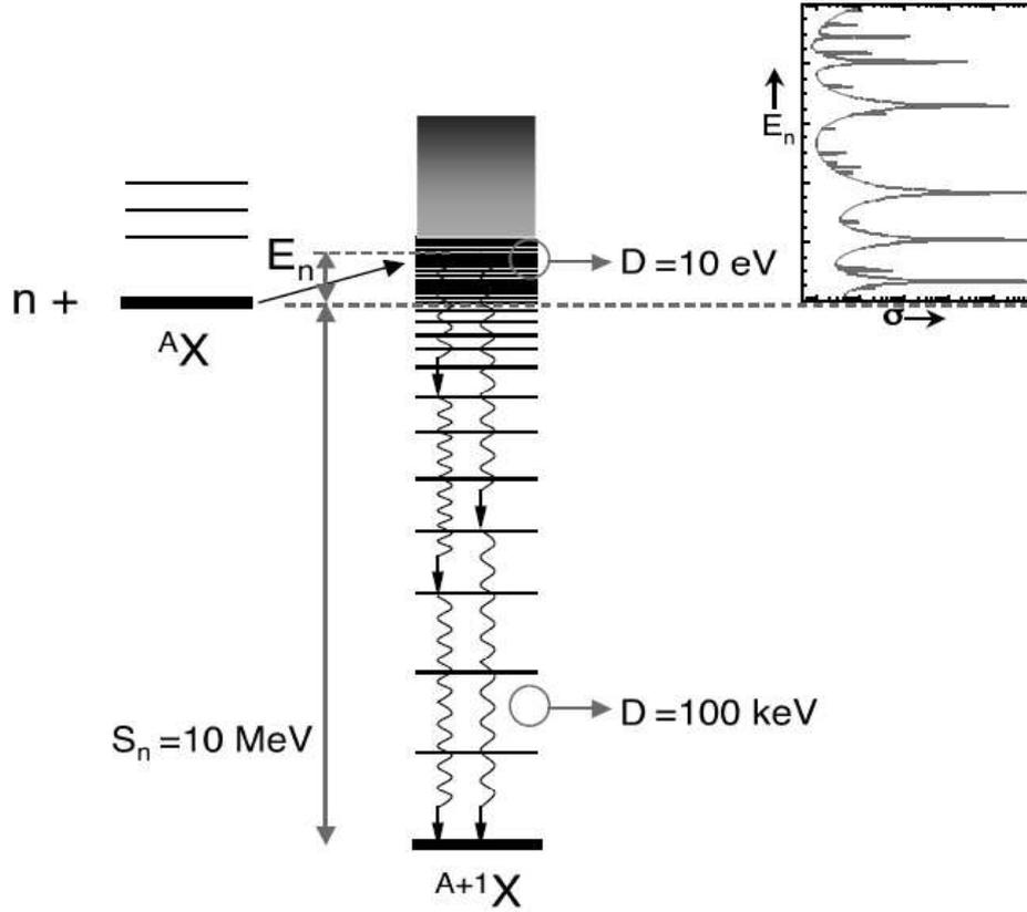
Figure 2.2: Schematic view of the formation a compound nucleus  $A+1X$  followed by the emission of  $\gamma$ -rays, corresponding to the radiative capture process. Typical values of the average level spacing  $D$  at different excitation energies are given as well as the neutron separation energy  $S_n$ .
