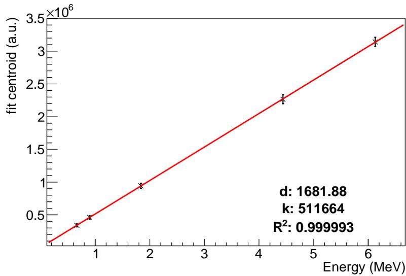
Figure 4.4: Calibration curve for BaF<sub>2</sub> module 7.
