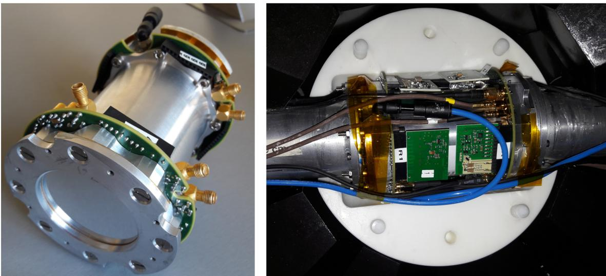
Figure 3.13: Pictures of the dummy fission chamber in the lab (left) and the  $^{233}\text{U}$  loaded fission chamber with electronics and gas connected and embedded in one half of the absorber inside the TAC (right).
