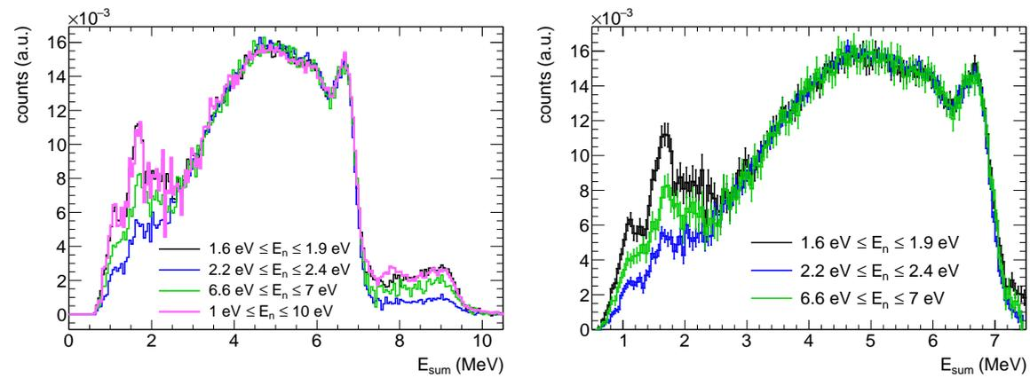
Figure 5.9: Sum energy spectra for TAC events with  $m_{cr} > 2$  in several neutron energy intervals without (left) and with (right) statistical errors displayed. The spectra have been normalized in the region  $3.5\text{ MeV} < E_{sum} < 7\text{ MeV}$  to compare the shapes.
