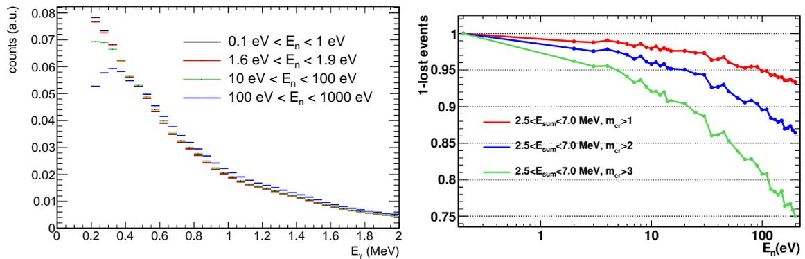
Figure 6.3: Individual  $\gamma$ -ray energies in the prompt fission cascades for different neutron energy intervals from this work (left). Decrease of the efficiency with neutron energy in the  $^{235}\text{U}(n,\gamma)$  cross section measurement [60, 107] performed at n\_TOF applying the fission tagging technique taken from [107] (right).
