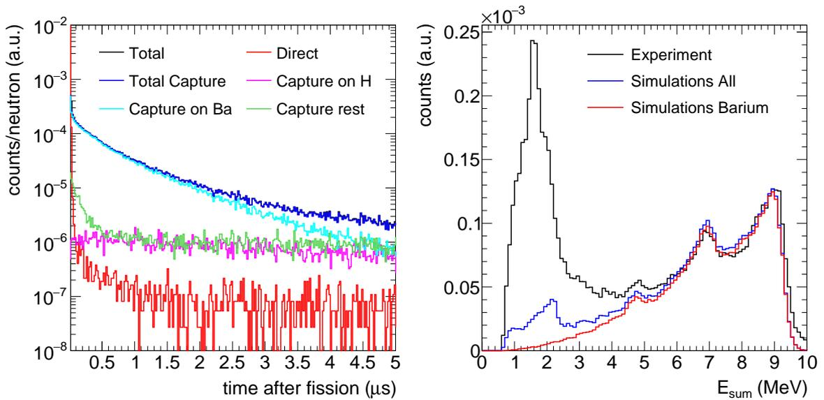
Figure 5.11: Distribution of events with  $m_{cr} > 2$  registered in the TAC (simulated) as a function of the time after neutron emission (left). Comparison of the simulated and experimental sum energy response of the TAC to fission neutrons for events with  $m_{cr} > 2$  and  $14 \text{ ns} < \delta T < 1 \mu\text{s}$  (right).
