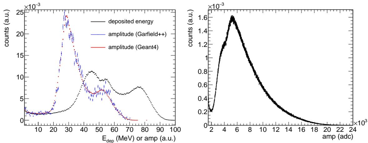
Figure 4.37: Deposited energy and calculated amplitude of fission fragments from a  $\text{U}_3\text{O}_8$  layer with a density of  $8.2 \text{ g/cm}^3$  and an areal density of  $\sigma = 305 \mu\text{g/cm}^2$   $^{233}\text{U}$  (left). Experimental amplitude spectra of FICH channel 4 with an areal density of  $\sigma = 305 \mu\text{g/cm}^2$   $^{233}\text{U}$  (right).
