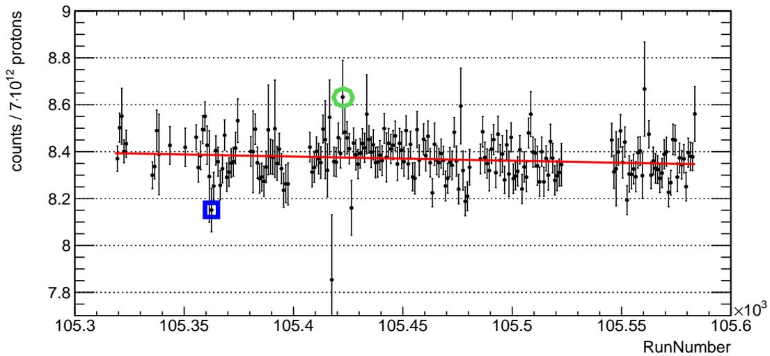
Figure 4.24: Gain drift over time: number of events with  $amp > 3500$  adc units per protons per Run - typically 4 hours make a Run. The red line is a linear fit to the data points, with  $p_0 = 27.0097$  and  $p_1 = -1.77E - 4$ .
