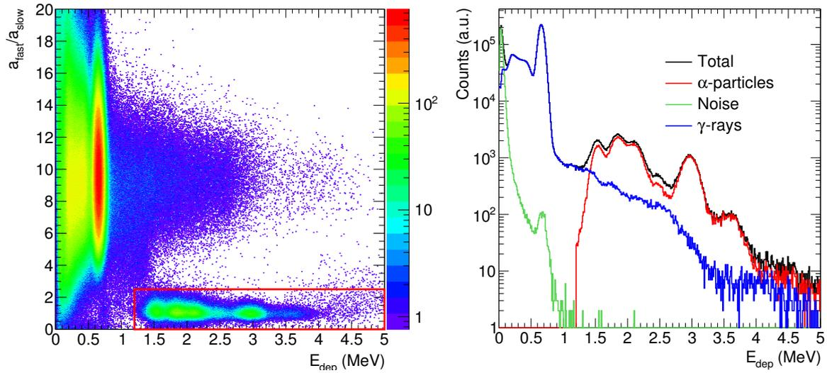
Figure 4.2: Particle discrimination of  $\alpha$ -particles in a  $\text{BaF}_2$  crystal with improved  $\alpha$ -particle cut indicated by the red framed region (left). Contributions to the total spectrum in a crystal (right) measured with a  $^{137}\text{Cs}$  calibration source (approx. 340 kBq).
