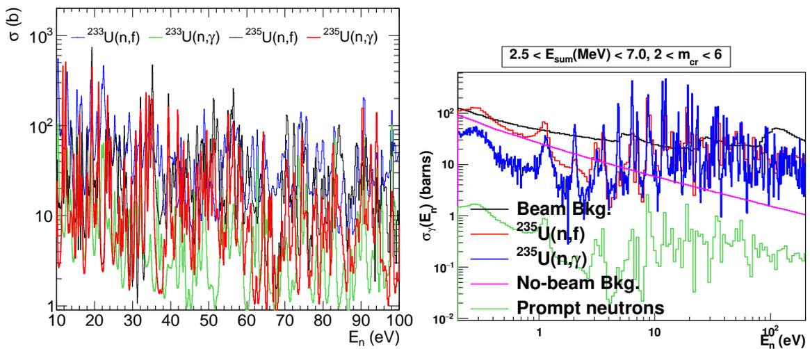
Figure 6.4: Capture and fission cross sections for  $^{233}\text{U}$  and  $^{235}\text{U}$  taken from ENDF/B-VIII.0(left). Background conditions in the  $^{235}\text{U}(n,\gamma)$  cross section measurement [60, 107] performed at n\_TOF applying the fission tagging technique taken from [107] (right).
