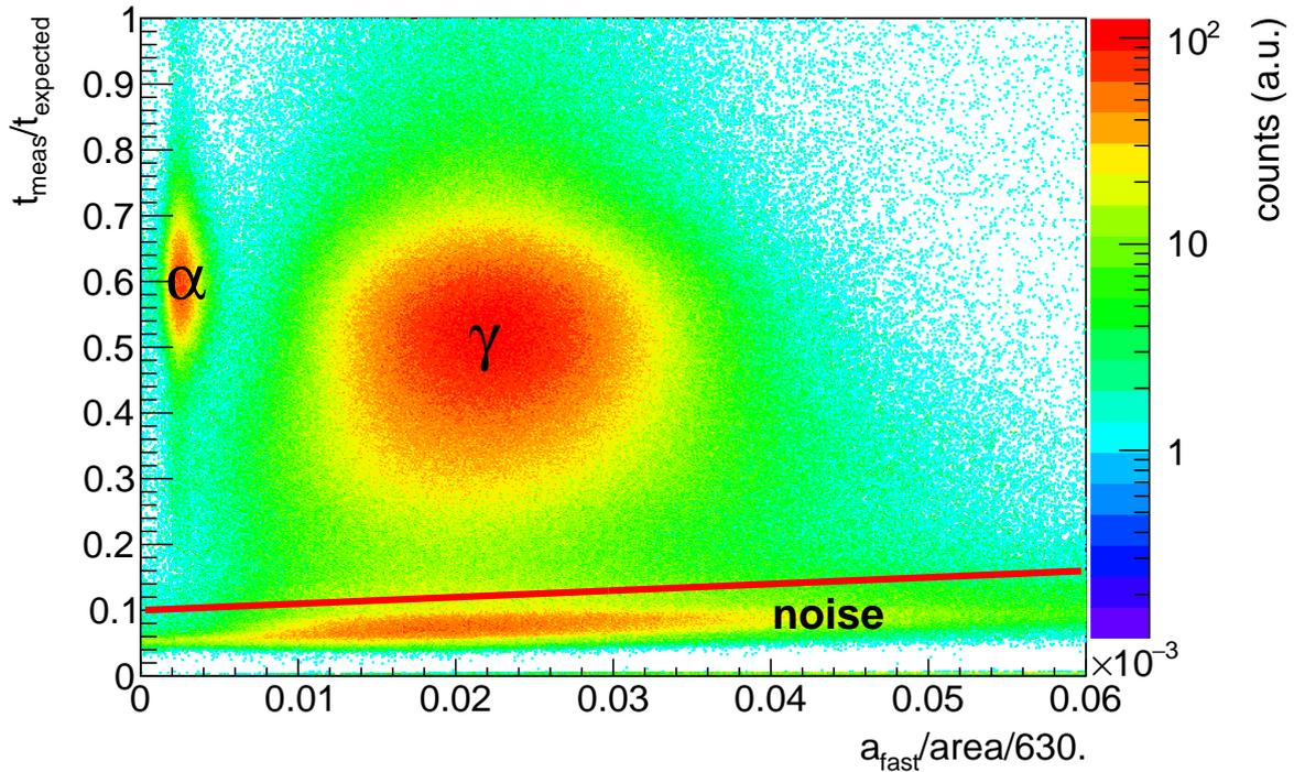
Figure 4.1: Particle discrimination in BaF<sub>2</sub>. The region below the red line corresponds to noise. The upper left hotspot corresponds to  $\alpha$ -particles while the central region corresponds to  $\gamma$ -rays.
