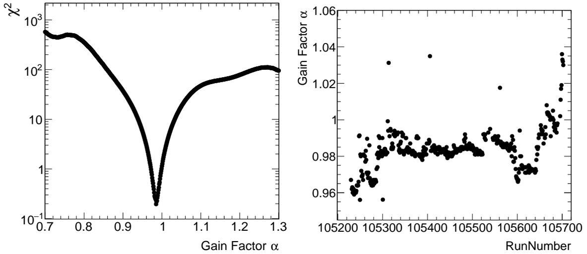
Figure 4.6:  $\chi^2$  for various gain factors  $\alpha$  for BaF<sub>2</sub> module 7 and Runnumber 105570 (left). Gain variation over time for BaF<sub>2</sub> module 7 (right).
