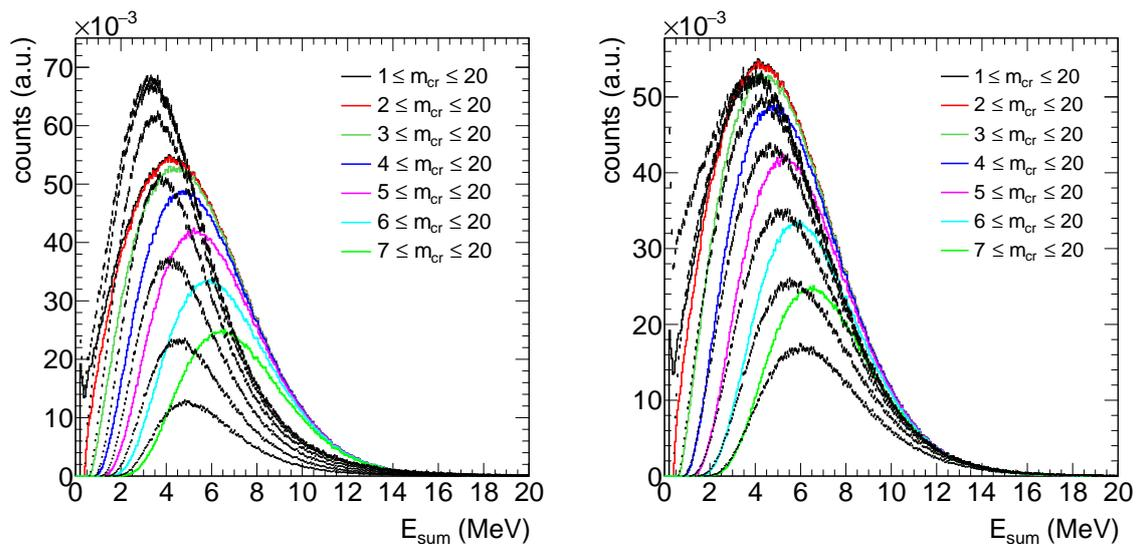
Figure 4.41: PFG spectra (dashed lines) using the model of Valentine [103] (left) and a modified model based on Valentine with modified parameters [104] used in a previous  $^{233}\text{U}(n,\gamma)$  measurement at n\_TOF (right) compared to the experimental data (solid lines).
