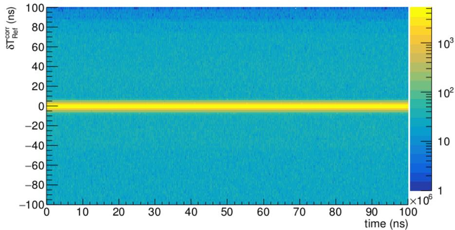
Figure 4.12: Time stability of the time differences (corrected for the constant time offset)  $\delta T_{Ref}^{corr}$  between all detectors and the reference detector. This nicely shows that there is no drift of the time window over the DAQ time window or time-of-flight.
