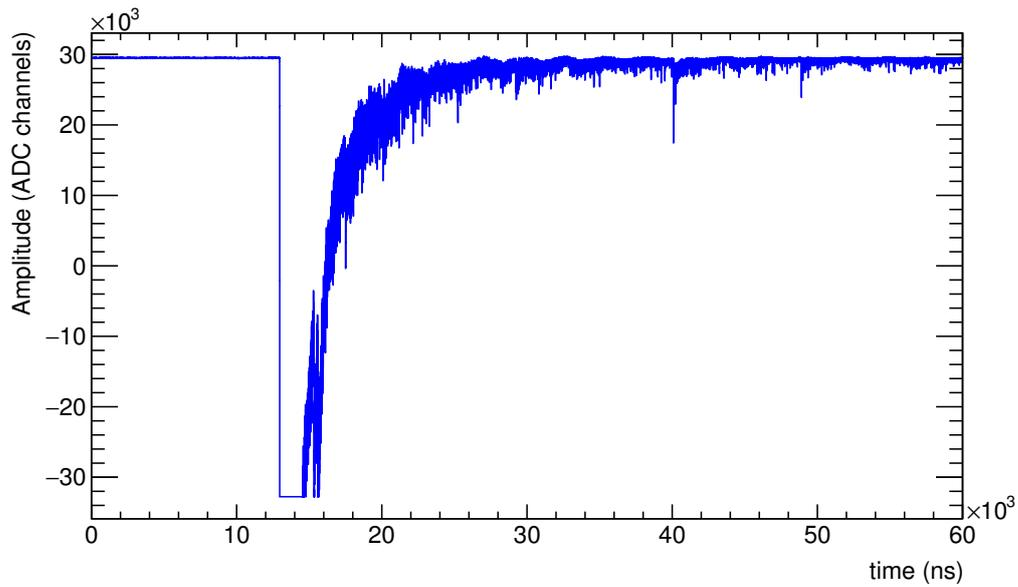
Figure 3.6: Example of the response of a  $\text{BaF}_2$  module to the  $\gamma$ -flash.
