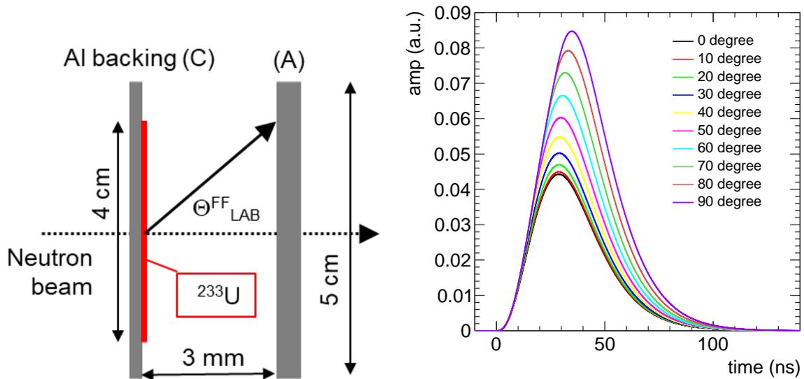
Figure 4.18: Definition of some quantities in the FICH simulations (left). Pulse shapes depending on the fission fragment's angle of emission  $\theta_{LAB}^{FF}$  in the lab frame simulated using GARFIELD++. In the simulations an equal amount of electrons was used (= same deposited energy) to calculate the signals.
