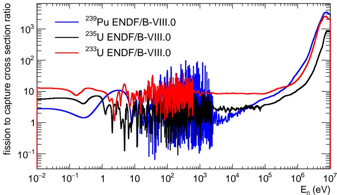
Figure 1.3: Inverse  $\alpha$ -ratio for  $^{233}\text{U}$ ,  $^{235}\text{U}$  and  $^{239}\text{Pu}$ .  $^{233}\text{U}$  has the largest inverse  $\alpha$ -ratio leading to a reduction in the amount of transuranic waste per energy unit produced.
