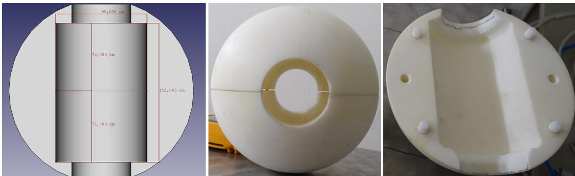
Figure 3.10: CAD drawing (left) and pictures (middle and right) of the neutron absorber used in the measurement.
