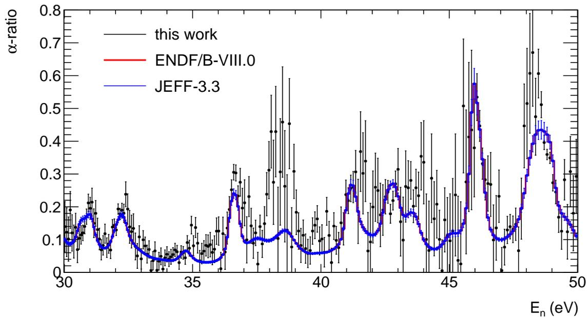
Figure 6.11: Comparison of the point wise experimental  $^{233}\text{U}$   $\alpha$ -ratio to the  $^{233}\text{U}$   $\alpha$ -ratio from ENDF/B-VIII.0 and JEFF-3.3 in the neutron energy region from 30 eV to 50 eV. No dead time corrections have been applied.
