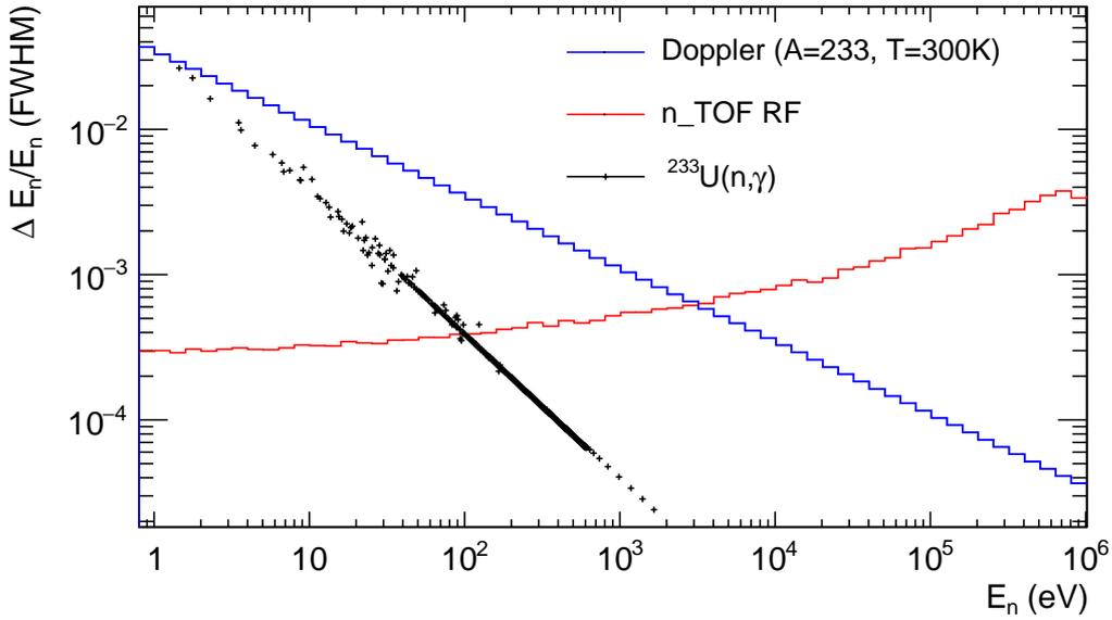
Figure 3.5: Comparison of the effects of Doppler Broadening ( $T = 297\text{ K}$ ) for  $^{233}\text{U}$  and of the n\_TOF resolution function on the resolution of the  $^{233}\text{U}$   $\alpha$ -ratio measurement. The resonance widths  $\Gamma_\gamma$  of the  $^{233}\text{U}(n,\gamma)$  resonances according to ENDF/B-VIII.0 are plotted.
