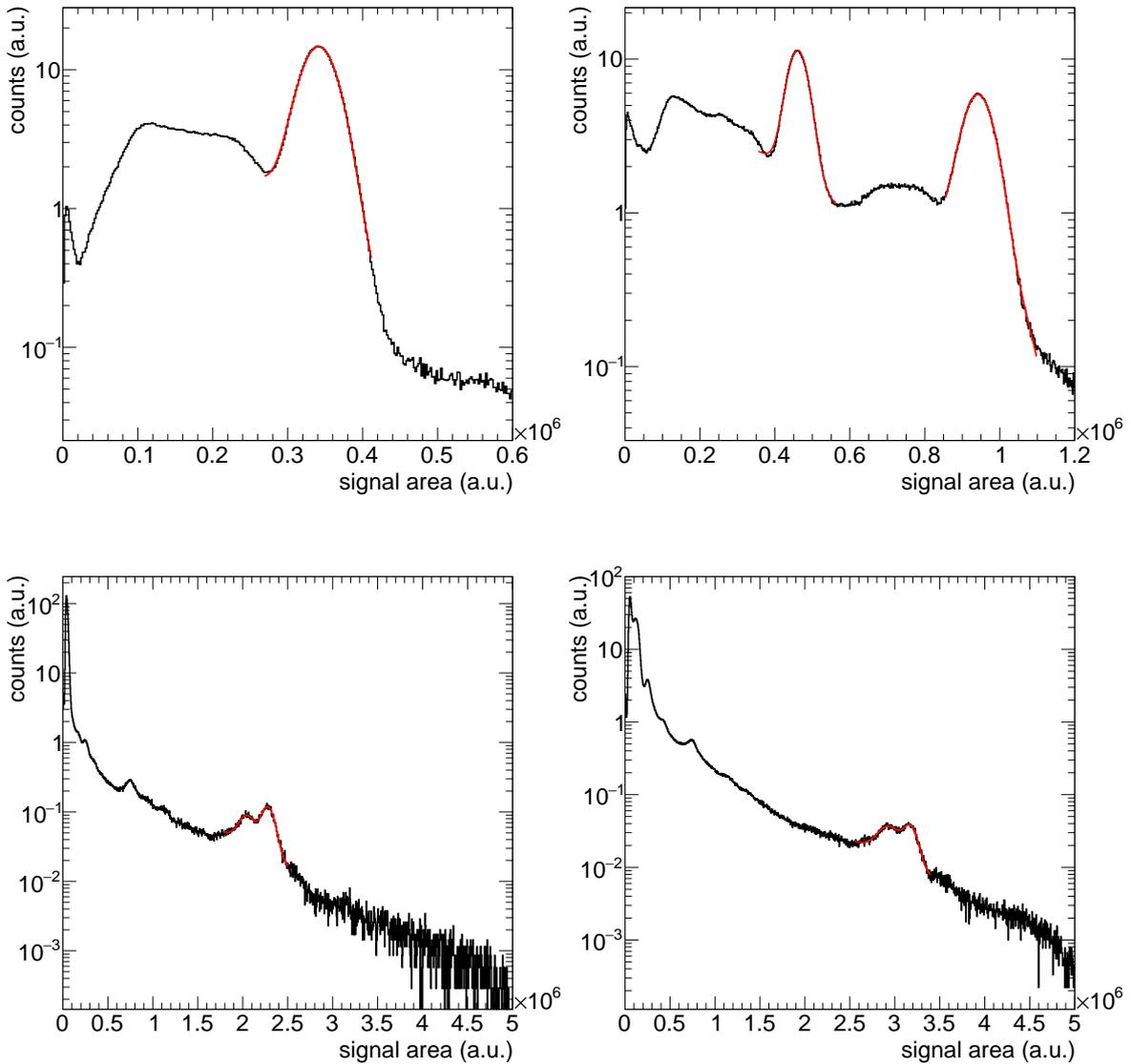
Figure 4.3: Response of BaF<sub>2</sub> module 7 to the standard calibration sources - <sup>137</sup>Cs (top left), <sup>88</sup>Y (top right), AmBe (bottom left), CmC (bottom right). Fits to the experimental data in red using different fitting functions.
