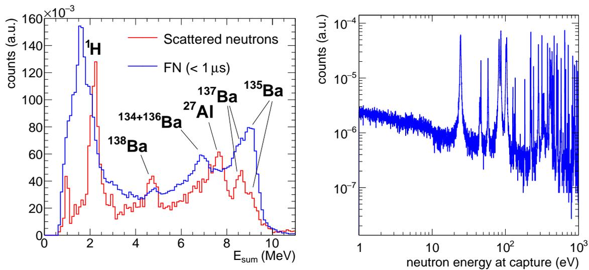
Figure 5.14: Comparison of the sum energy spectra of FN and elastic neutron scattering, obtained by using a carbon sample, for events with  $m_{cr} > 2$ . The sum-energy peaks, labeled with nucleus  $^AZ$ , correspond to the neutron separation energy of the compound nucleus  $^{A+1}Z$  after capture  $^AZ+n$  (left). Neutron energy spectrum at capture during moderation of fission neutrons from simulations (right).
