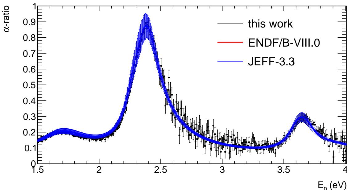
Figure 6.8: Comparison of the point wise experimental  $^{233}\text{U}$   $\alpha$ -ratio compared to the  $^{233}\text{U}$   $\alpha$ -ratio from ENDF/B-VIII.0 and JEFF-3.3 for the two big resonances from  $0.5\text{ eV} < E_n < 4\text{ eV}$ .
