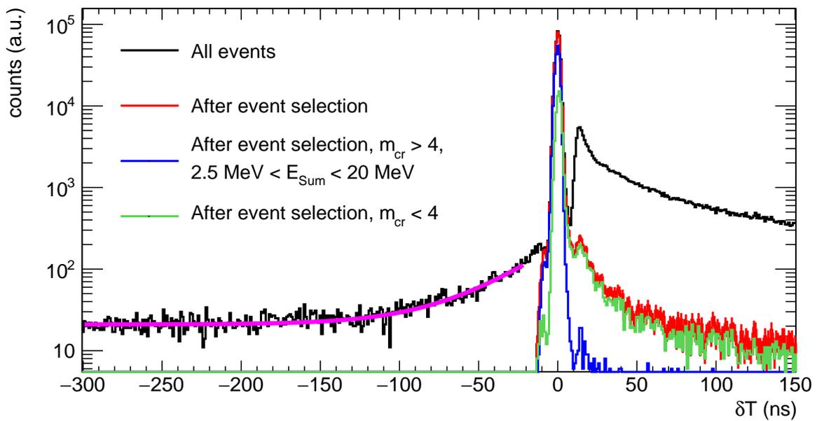
Figure 7.1: Time difference distribution between TAC and FICH events for a maximum allowed coincidence window  $T_{coinc}^{TAC-FICH} = 1\mu s$  and with different conditions applied to the TAC signals. Same Figure as 4.30.
