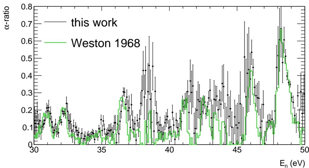
Figure 6.18: Comparison of the point wise experimental  $^{233}\text{U}$   $\alpha$ -ratio from this work and from the experimental data sets from Weston in the neutron energy region from  $30\text{ eV} < E_n < 50\text{ eV}$ . No dead time corrections have been applied.
