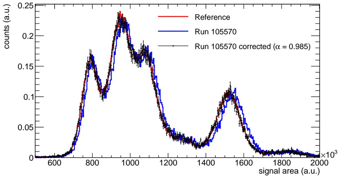
Figure 4.5: Illustration of the gain correction method for BaF<sub>2</sub> module 7.
