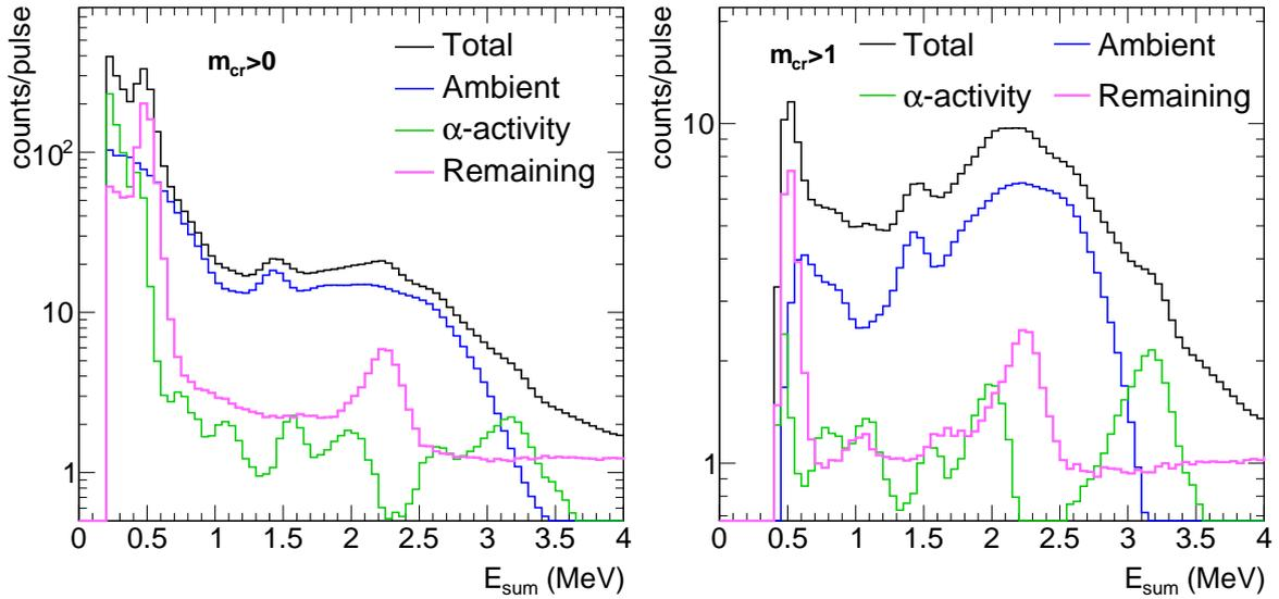
Figure 5.1: Comparison of the sum energy spectra in the TAC of the time independent background components and the total measured response in the neutron energy range from 0.02 eV up to 10 keV for  $m_{cr} > 0$  (left) and  $m_{cr} > 1$  (right).
