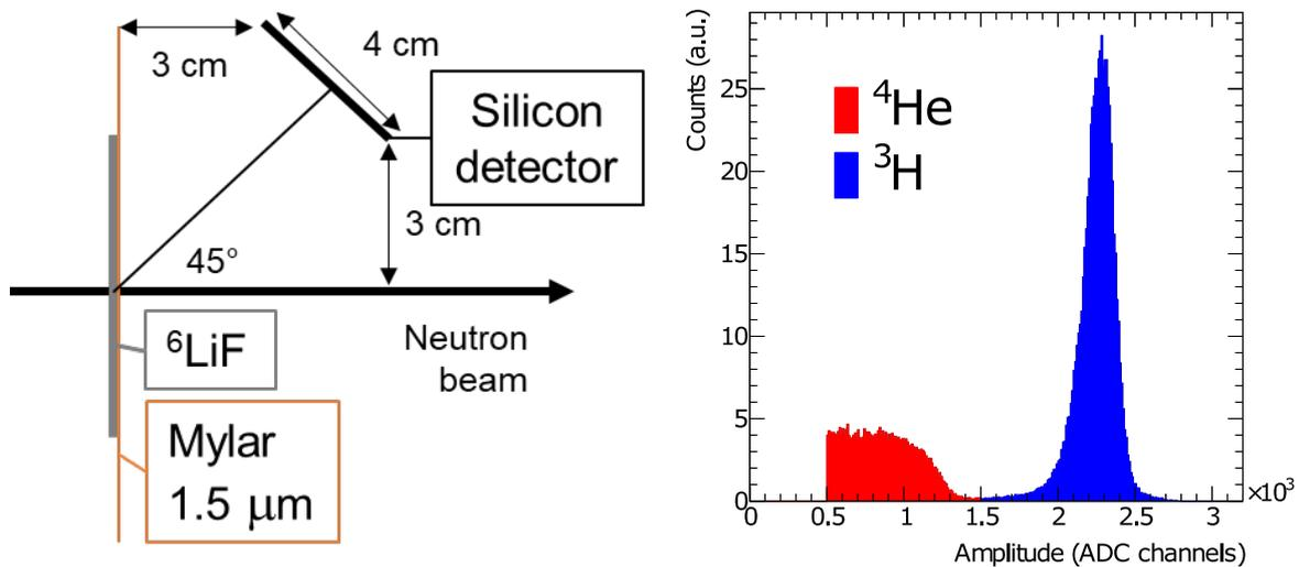
Figure 3.7: Scheme of the SiMon detector (left, from [79]) and the pulse height spectrum (right), where the alpha region and the triton peak are nicely separated.
