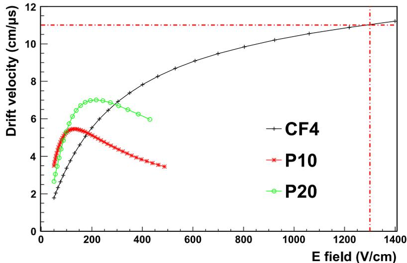
Figure 3.15: GARFIELD simulations of the electron drift velocities for different experimental gases at atmospheric pressure as a function of the applied electric field taken from Ref. [83].
