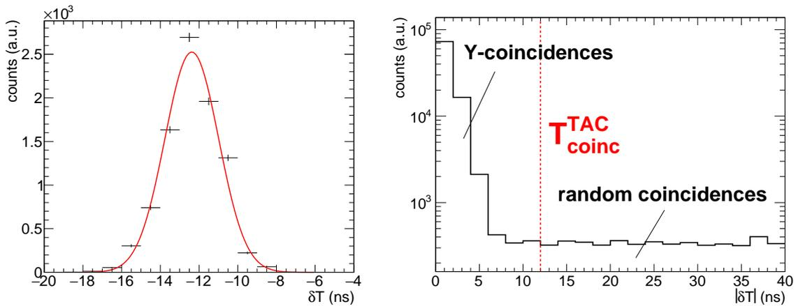
Figure 4.10: Time differences between signals from the reference detector and detector 7 where  $E_{Sum} \approx 2.7$  MeV. The timing offset between those two detectors equals the centroid of the Gaussian fit of  $-12.4$  ns (left). Time offset corrected time differences - the optimal coincidence window  $T_{coinc}^{TAC}$  is indicated at 12 ns (right).
