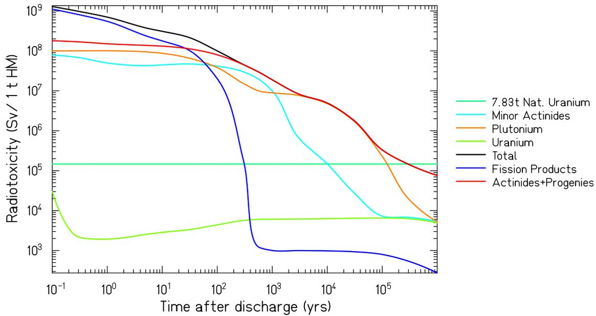
Figure 1.1: Radiotoxicity of spent nuclear fuel in Sv per 1 ton of heavy metal as a function of time after discharge from the reactor, taken from [18].
