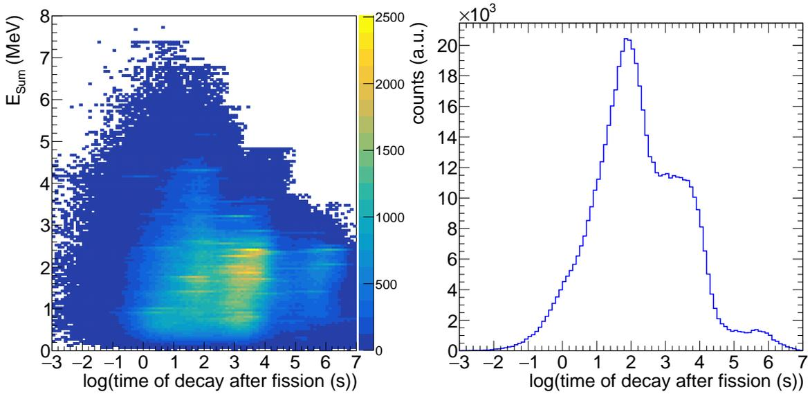
Figure 5.5: Sum energy and time distribution of the decay of fission products simulated with GEANT4 (left). Time distribution of fission product decay events with  $m_{cr} > 2$  and  $2.5 \text{ MeV} < E_{Sum} < 7 \text{ MeV}$ .
