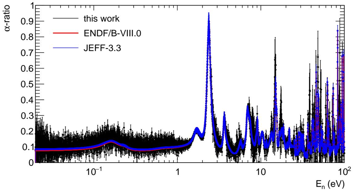
Figure 6.6: Experimental  $^{233}\text{U}$   $\alpha$ -ratio calculated from events with  $3 \leq m_{cr} \leq 7$  and  $2.5 \text{ MeV} < E_{sum} < 7 \text{ MeV}$  compared to the  $^{233}\text{U}$   $\alpha$ -ratio from ENDF/B-VIII.0 and JEFF-3.3 up to 100 eV. No dead time corrections have been applied.
