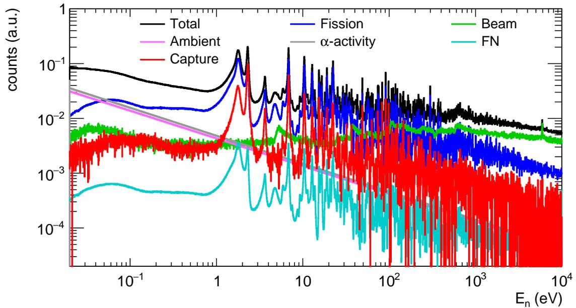
Figure 6.2: Experimental response of the TAC to the different components obtained either by direct measurement or subtraction of components from the total response for events with  $3 \leq m_{cr} \leq 7$  and  $2.5 \text{ MeV} < E_{sum} < 7 \text{ MeV}$ .
