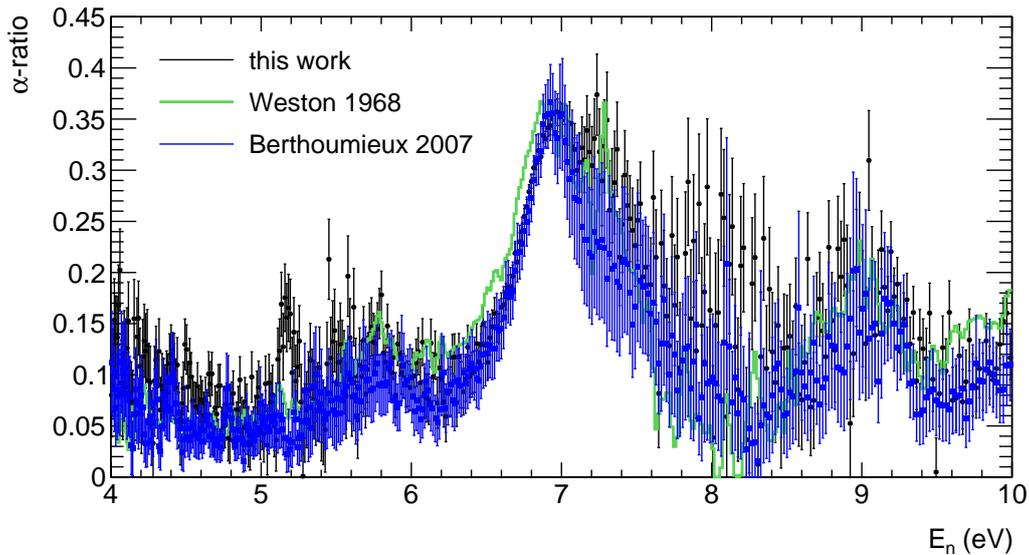
Figure 6.16: Comparison of the point wise experimental  $^{233}\text{U}$   $\alpha$ -ratio from this work and from the experimental data sets from Weston and Berthoumieux in the neutron energy region from  $4\text{ eV} < E_n < 10\text{ eV}$ . The experimental data from this work shows a structure at 5.15 eV as expected due to the 0.0496%  $^{234}\text{U}$  contamination of the samples, see section 3.4.
