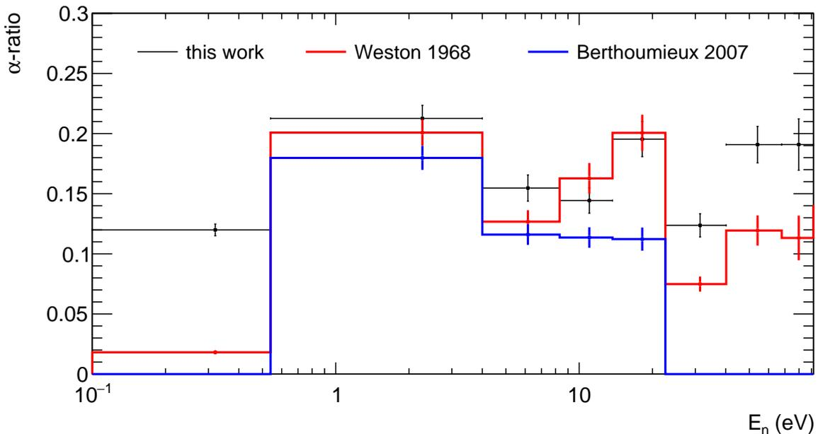
Figure 6.20: Comparison of the average values of the experimental, Weston and Berthoumieux  $^{233}\text{U}$   $\alpha$ -ratio for neutron energy intervals according to the 33 group energy structure of the WPEC Subgroup 33 (SG33) [120]. The corresponding values are summarized in Table 6.5.
