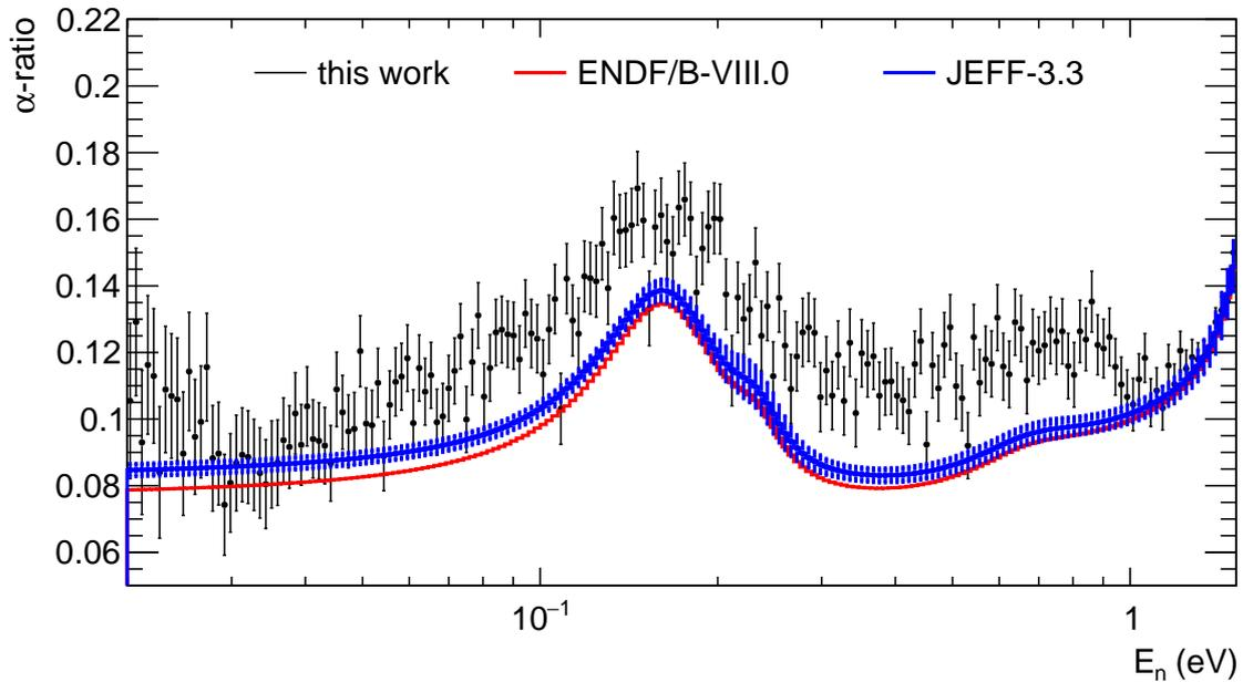
Figure 6.7: Comparison of the point wise experimental  $^{233}\text{U}$   $\alpha$ -ratio compared to the  $^{233}\text{U}$   $\alpha$ -ratio from ENDF/B-VIII.0 and JEFF-3.3 for the low energy region from 0.02 eV to 1.5 eV.
