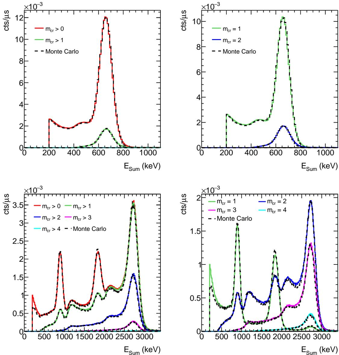
Figure 3.22: Comparison between simulated results (dashed lines) and experimental data (solid/colored lines) for the  $^{137}\text{Cs}$  (top)  $^{88}\text{Y}$  (bottom) calibration source including the absorber.
