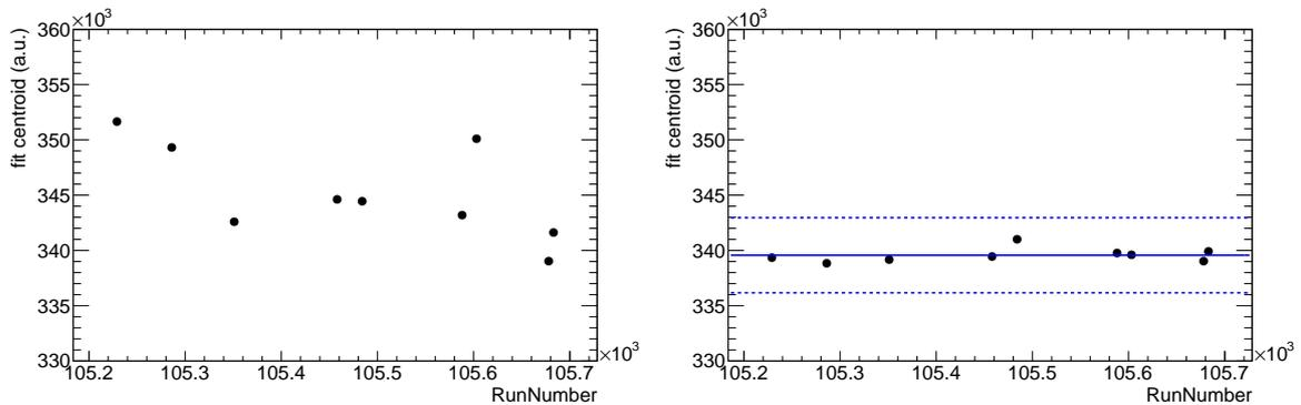
Figure 4.7: Fit centroid of the <sup>137</sup>Cs standard calibration source over time before (left) and after (right) gain correction for BaF<sub>2</sub> module 7. The blue solid line corresponds to the average and the dashed line to its error.
