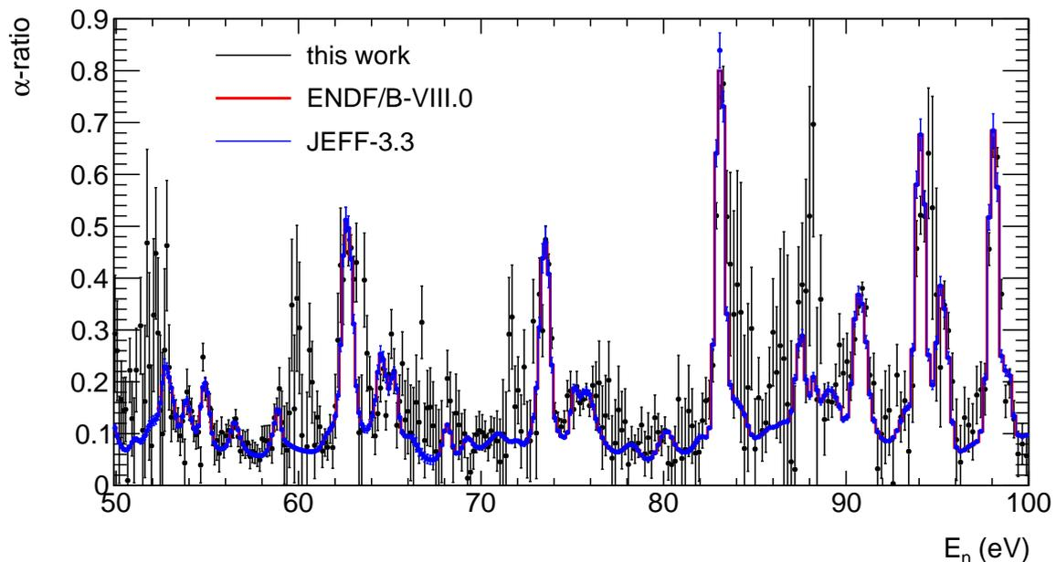
Figure 6.12: Comparison of the point wise experimental  $^{233}\text{U}$   $\alpha$ -ratio to the  $^{233}\text{U}$   $\alpha$ -ratio from ENDF/B-VIII.0 and JEFF-3.3 in the neutron energy region from 50 eV to 100 eV. No dead time corrections have been applied.
