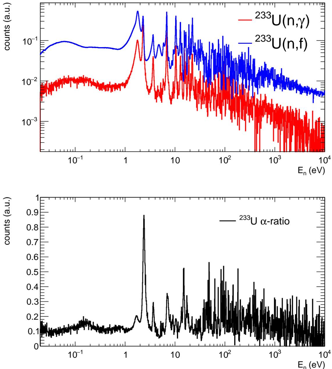
Figure 6.5: Comparison of the experimentally obtained counts for the  $^{233}\text{U}(n,\gamma)$  reaction from the TAC and for the  $^{233}\text{U}(n,f)$  reaction from FICH (top) for events with  $3 \leq m_{cr} \leq 7$  and  $2.5 \text{ MeV} < E_{sum} < 7 \text{ MeV}$  and  $A_{th} = 2500$  adc units. Experimental  $^{233}\text{U}$   $\alpha$ -ratio calculated from the spectra in the top panel (bottom). No dead time corrections have been applied.
