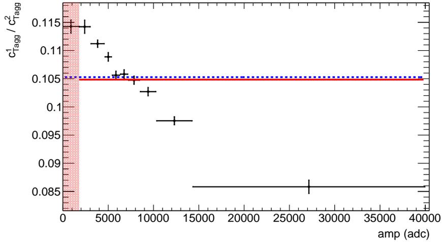
Figure 5.19: Ratio between the number of tagged fission counts with restrictive (1,  $E_{Sum} > 10$  MeV and  $m_{cr} > 6$ ) and relaxed conditions (2,  $2.5$  MeV  $< E_{Sum} < 7$  MeV and  $3 \leq m_{cr} \leq 7$ ) as a function of the FICH signal amplitude. The red and blue lines indicate the averages of the points in their respective intervals.
