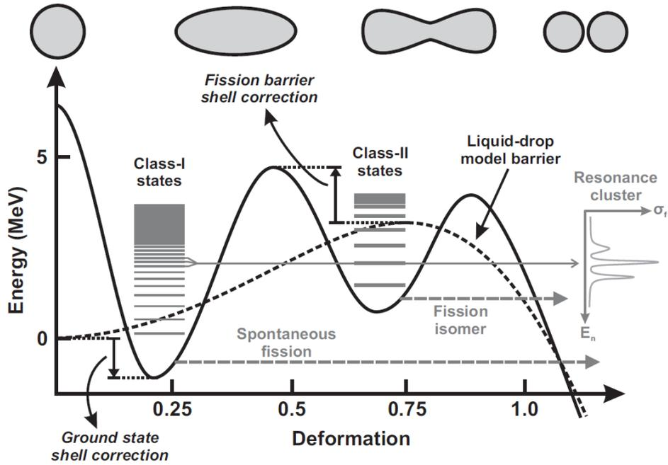
Figure 2.3: Schematic illustration of the double-humped fission potential, taken from [53]
