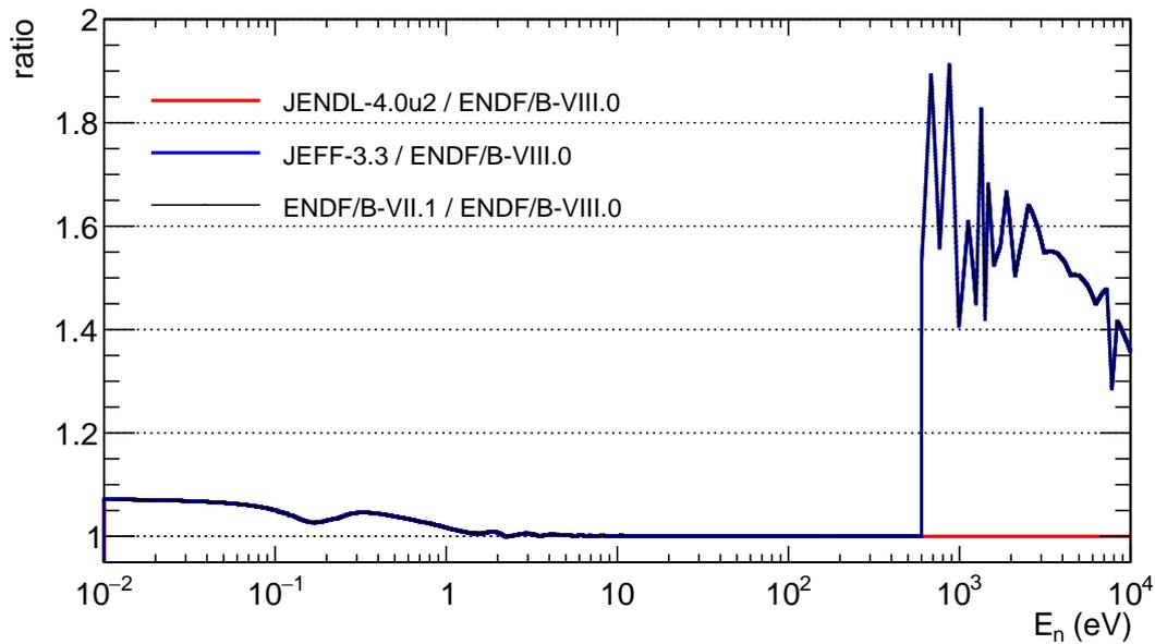
Figure 1.6: Comparison of the  $^{233}\text{U}(n,\gamma)$  cross section ratios between several evaluated libraries and the ENDF/B-VIII.0 library. Significant discrepancies can be seen in the URR above 600 eV while deviations within 8% are observed for neutron energies below 10 eV.
