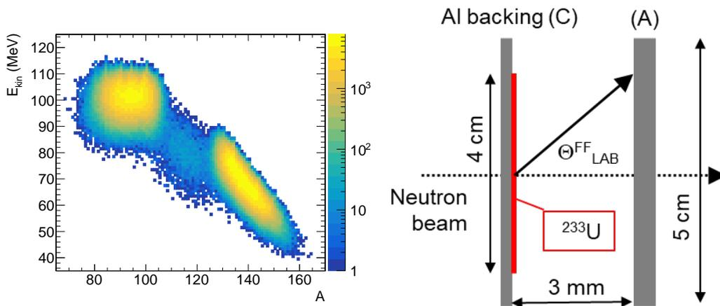
Figure 4.35: Fission fragment distribution for thermal fission of  $^{233}\text{U}$  according to the GEF code (left). Schematic illustration of the ionization cell geometry used in GEANT4 simulations (right).
