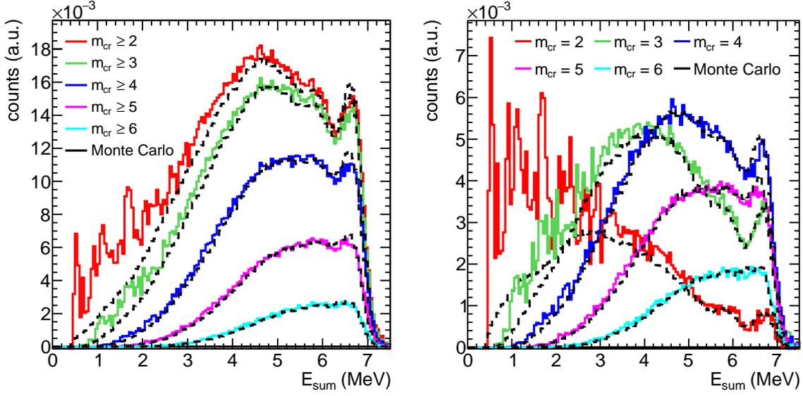
Figure 7.2: Comparison of the experimental and simulated sum energy spectra of  $^{233}\text{U}(n,\gamma)$  events for various crystal multiplicity conditions. For multiplicities larger than 2 a good agreement is achieved. Same Figure as 5.22.
