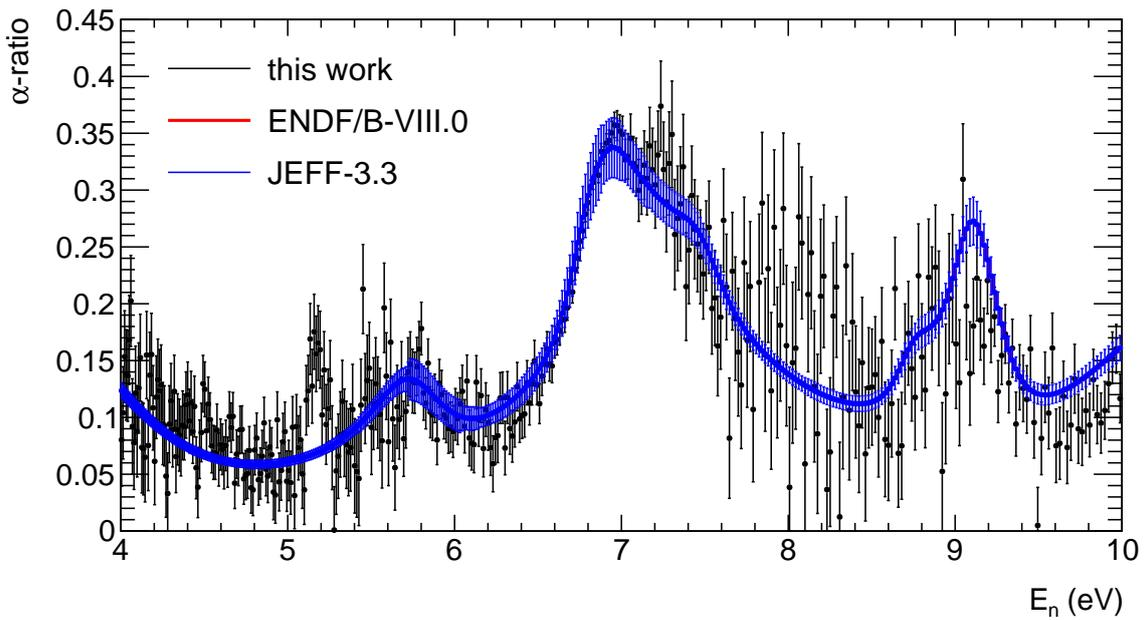
Figure 6.9: Comparison of the point wise experimental  $^{233}\text{U}$   $\alpha$ -ratio compared to the  $^{233}\text{U}$   $\alpha$ -ratio from ENDF/B-VIII.0 and JEFF-3.3 in the neutron energy region  $4\text{ eV} < E_n < 10\text{ eV}$ . The experimental data from this work shows a structure at  $5.15\text{ eV}$  as expected due to the  $0.0496\%$   $^{234}\text{U}$  contamination of the samples, see section 3.4.
