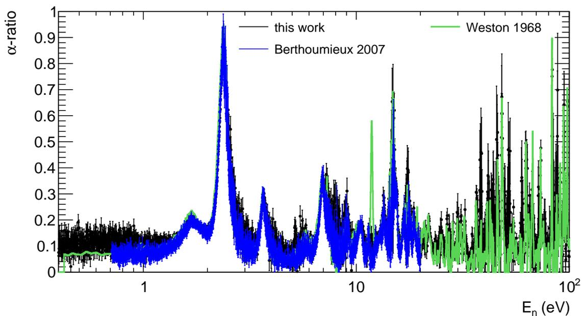
Figure 6.14: Comparison of the point wise experimental  $^{233}\text{U}$   $\alpha$ -ratio from this work and from the experimental data sets from Weston and Berthoumieux up to 100 eV. No dead time corrections have been applied.
