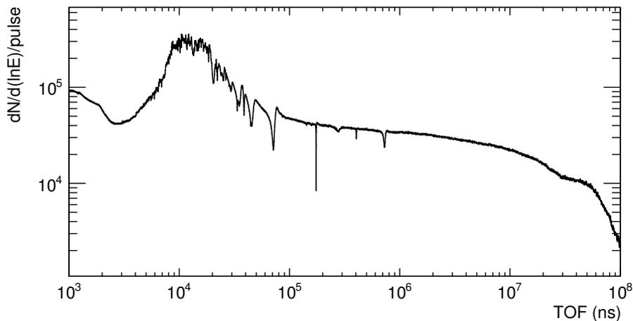
Figure 4.16: Neutron fluence in EAR1 at 185 m flight path from FLUKA simulations in isoethargic units. Note the increased fluence in the region  $5 \mu\text{s} < TOF < 15 \mu\text{s}$ .
