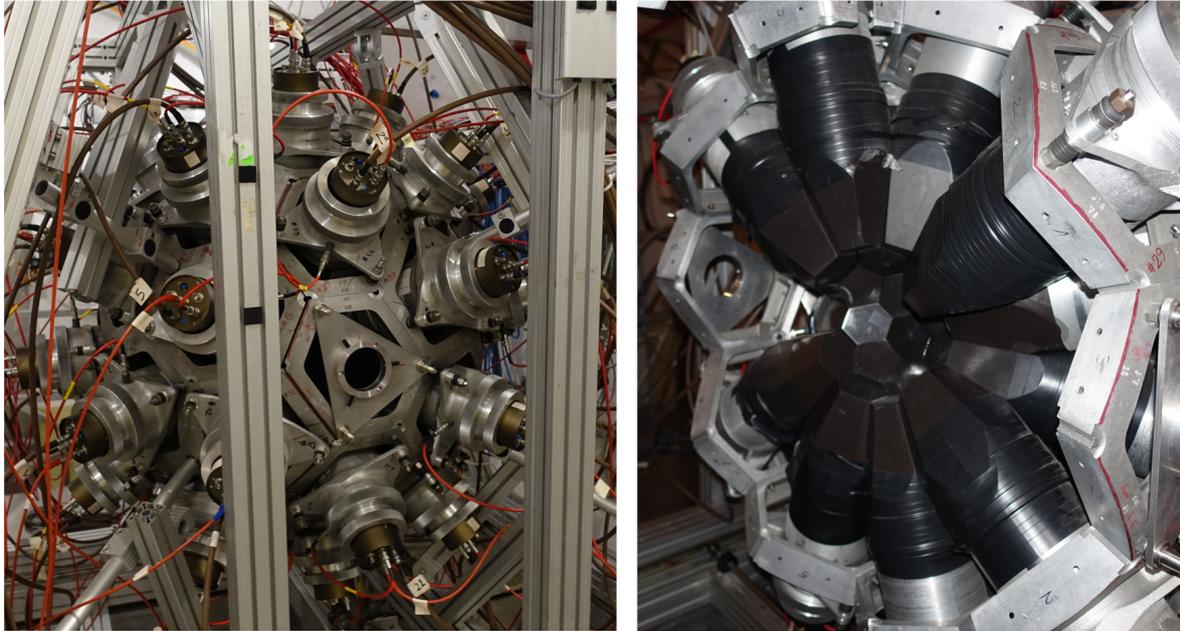
Figure 3.9: Pictures of the fully assembled (left) and open (right) TAC.
