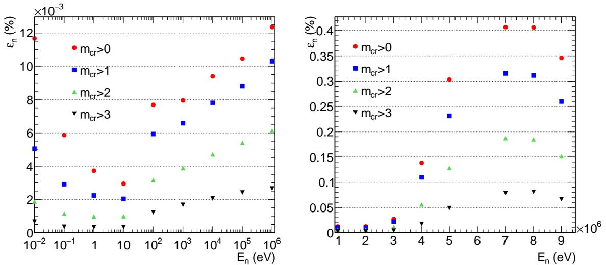
Figure 5.3: Neutron sensitivity  $\varepsilon_n(E_n; E_{Sum}, m_{cr})$  as a function of the neutron energy and crystal multiplicity for events with  $2.5\text{ MeV} < E_{Sum} < 7\text{ MeV}$  for different neutron energy ranges.
