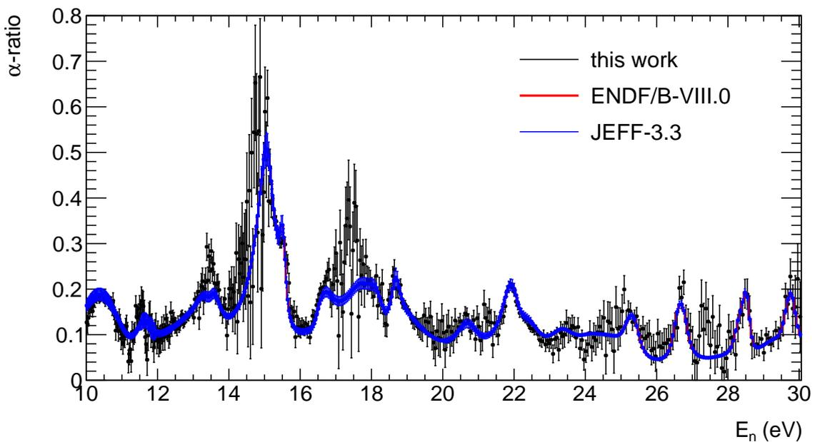
Figure 6.10: Comparison of the point wise experimental  $^{233}\text{U}$   $\alpha$ -ratio to the  $^{233}\text{U}$   $\alpha$ -ratio from ENDF/B-VIII.0 and JEFF-3.3 in the neutron energy region from  $10\text{ eV}$  to  $30\text{ eV}$ . No dead time corrections have been applied.
