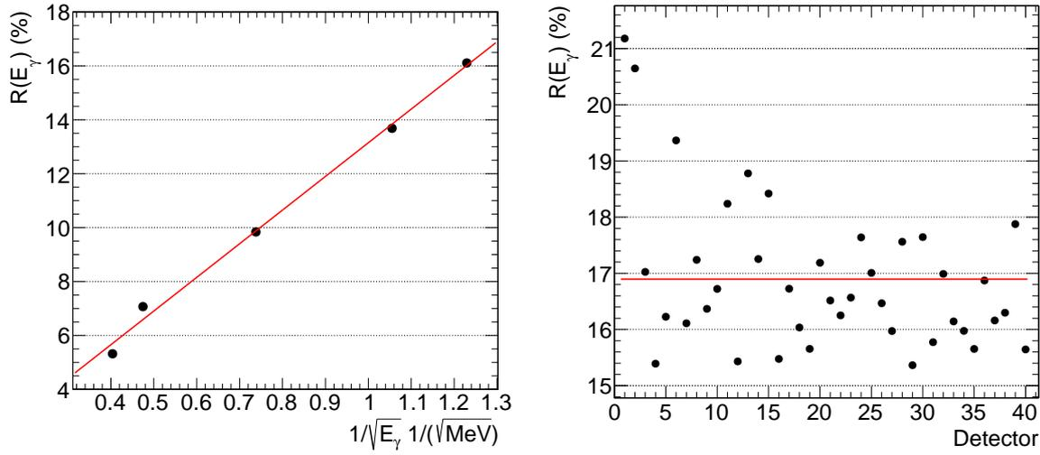
Figure 4.8: Energy resolution for BaF<sub>2</sub> module 7 - smaller  $E_\gamma$  are on the upper end of the x-axis (left). Energy resolution of all detectors at  $E_\gamma = 0.662$  MeV from <sup>137</sup>Cs. The average (red line) of all crystals is calculated to  $R(E_\gamma = 0.662 \text{ MeV}) \approx 16.9\%$  (right).
