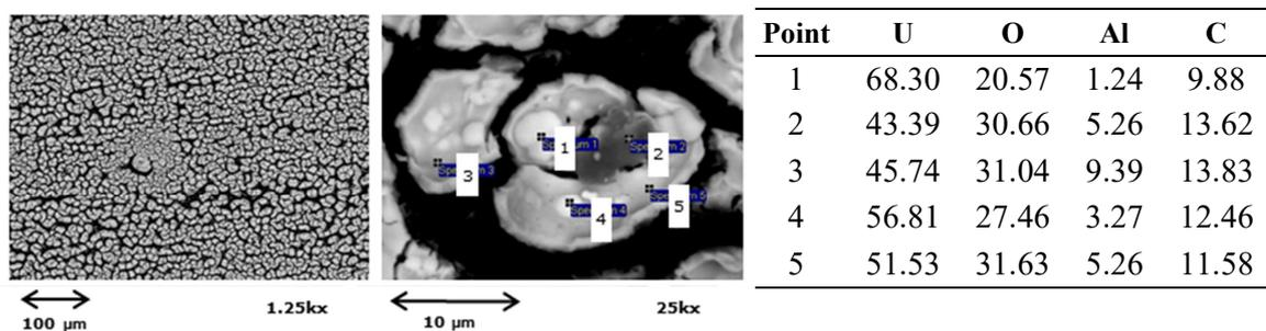
Figure 3.20: SEM image of a molecular plated  $^{238}\text{U}$  layer (left and middle). Elemental composition in wt% measured with XPS at different regions of the layer (right) as indicated in the middle panel. Image taken from [85].
