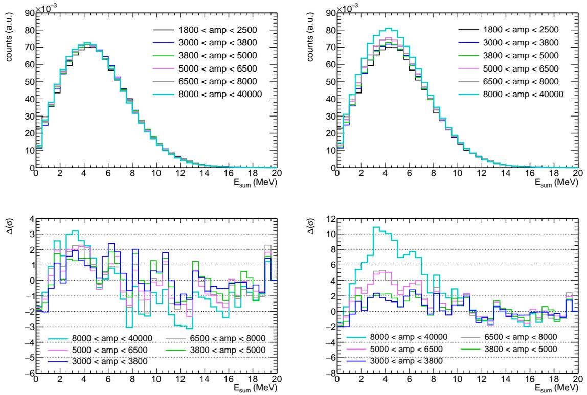
Figure 5.18: Sum energy spectra for different amplitude cuts normalized to the total integral (left) and normalized in the tail of the distribution ( $E_{sum} > 10$  MeV) (right). In the bottom panels the ratios of the corresponding amplitude regions to the region  $1800 < amp(adunits) < 2500$  are shown.
