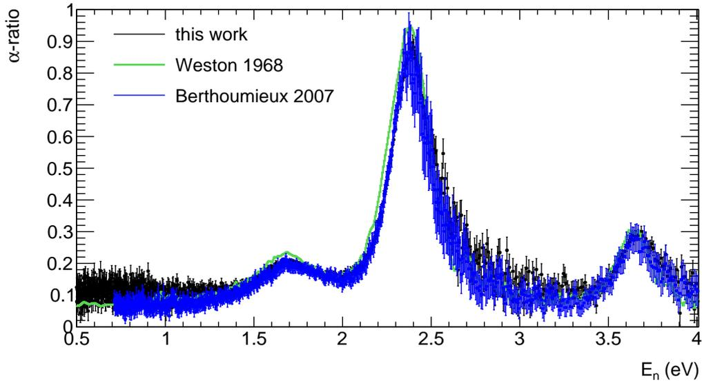
Figure 6.15: Comparison of the point wise experimental  $^{233}\text{U}$   $\alpha$ -ratio from this work and from the experimental data sets from Weston and Berthoumieux for the two largest resonances from  $0.5\text{ eV} < E_n < 4\text{ eV}$ .
