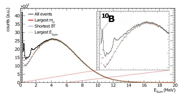
Figure 4.31: Comparison of the different event selection algorithms using either largest  $E_{sum}$ , largest  $m_{cr}$  or smallest  $\delta T^{TAC-FICH}$  as primary criteria. In the zoom in the region for  $E_{Sum} < 6$  MeV the suppression of the 480 keV  $\gamma$ -ray emitted in the <sup>10</sup>B(n, $\alpha$ ) reaction and the 1435 keV  $\gamma$ -ray from inelastic scattering of fission neutrons on <sup>138</sup>Ba can be observed.
