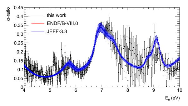
Figure 6.9: Comparison of the point wise experimental  $^{233}$ U  $\alpha$ -ratio compared to the  $^{233}$ U  $\alpha$ -ratio from ENDF/B-VIII.0 and JEFF-3.3 in the neutron energy region 4 eV  $< E_n <$  10 eV. The experimental data from this work shows a structure at 5.15 eV as expected due to the 0.0496 %  $^{234}$ U contamination of the samples, see section 3.4.
