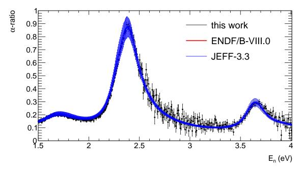
Figure 6.8: Comparison of the point wise experimental <sup>233</sup>U  $\alpha$ -ratio compared to the <sup>233</sup>U  $\alpha$ -ratio from ENDF/B-VIII.0 and JEFF-3.3 for the two big resonances from 0.5 eV  $< E_n < 4$  eV.
