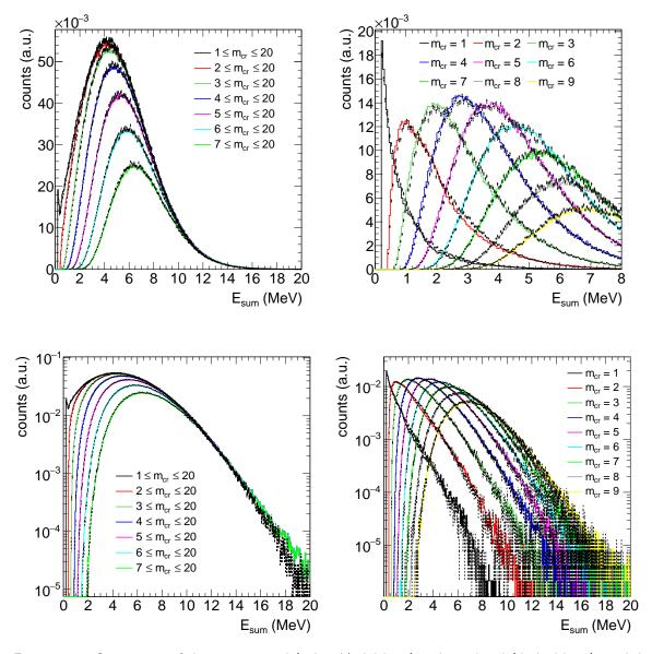
Figure 4.44: Comparison of the experimental (colored/solid lines) and simulated (dashed lines) total deposited energy  $E_{Sum}$  spectra in the TAC from prompt fission  $\gamma$ -rays for various conditions in crystal multiplicity  $m_{cr}$ . The DANCE PFG cascade generator was used with optimized parameters.
