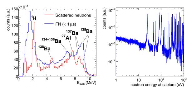
Figure 5.14: Comparison of the sum energy spectra of FN and elastic neutron scattering, obtained by using a carbon sample, for events with  $m_{cr} > 2$ . The sum-energy peaks, labeled with nucleus  ${}^{A}Z$ , correspond to the neutron separation energy of the compound nucleus  ${}^{A+1}Z$  after capture  ${}^{A}Z$ +n (left). Neutron energy spectrum at capture during moderation of fission neutrons from simulations (right).
