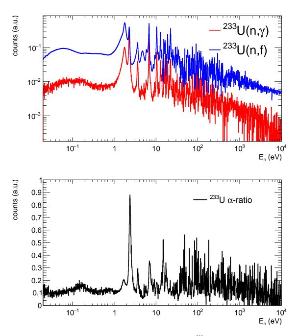
Figure 6.5: Comparison of the experimentally obtained counts for the  $^{233}U(n,\gamma)$  reaction from the TAC and for the  $^{233}U(n,f)$  reaction from FICH (top) for events with  $3 \leq m_{cr} \leq 7$  and 2.5 MeV  $< E_{sum} < 7$  MeV and  $A_{th} = 2500$  adc units. Experimental  $^{233}$ U $\alpha$ -ratio calculated from the spectra in the top panel (bottom). No dead time corrections have been applied.
