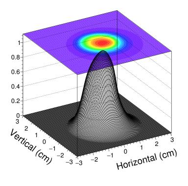
Figure 3.4: Spatial profile of the neutron beam in EAR1 at 185 m taken from FLUKA simulations for the full energy range of  $n\_TOF$ .
