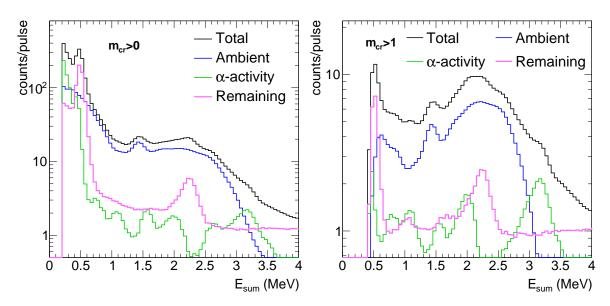
Figure 5.1: Comparison of the sum energy spectra in the TAC of the time independent background components and the total measured response in the neutron energy range from 0.02 eV up to 10 keV for  $m_{cr} > 0$  (left) and  $m_{cr} > 1$  (right).
