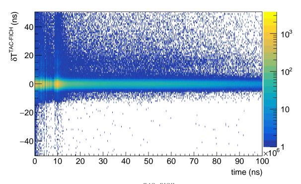
Figure 4.33: Stability of the time differences  $\delta T^{TAC-FICH}$  for fission events in coincidence with TAC events with time. No drift can be observed.
