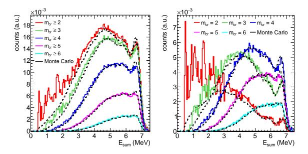
Figure 7.2: Comparison of the experimental and simulated sum energy spectra of  $^{233}U(n,\gamma)$  events for various crystal multiplicity conditions. For multiplicities larger than 2 a good agreement is achieved. Same Figure as 5.22.
