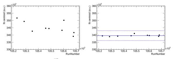
Figure 4.7: Fit centroid of the  $^{137}$ Cs standard calibration source over time before (left) and after (right) gain correction for BaF<sub>2</sub> module 7. The blue solid line corresponds to the average and the dashed line to its error.
