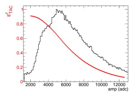
Figure 5.17: Fission tagging efficiency  $\varepsilon_{TAC}^{f}$  as a function of the FICH amplitude. The FICH amplitude spectrum in coincidence with the TAC for events with  $m_{cr} > 6$  and  $E_{Sum} > 10$  MeV is shown as well.
