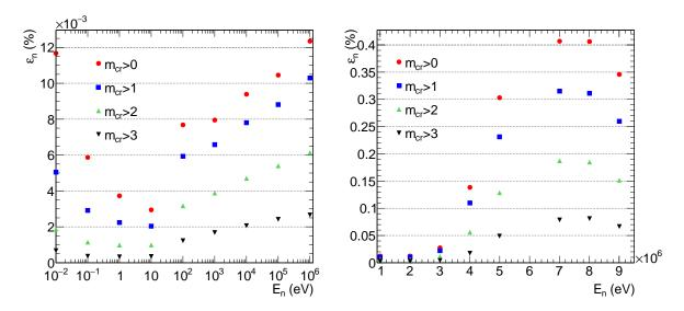
Figure 5.3: Neutron sensitivity  $\varepsilon_n(E_n; E_{Sum}, m_{cr})$  as a function of the neutron energy and crystal multiplicity for events with 2.5 MeV  $< E_{Sum} < 7$  MeV for different neutron energy ranges.
