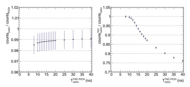
Figure 4.32: Fraction of found coincidences with respect to the total number of fission events in the FICH for different TAC-FICH coincidence windows  $T_{coinc}^{TAC-FICH}$  (left). Fraction of events where exactly one TAC event is found for one FICH event with respect to all found coincidences (right). Both for events with amp > 3000 adc units and 1.6 eV<  $E_n < 1.9$  eV.
