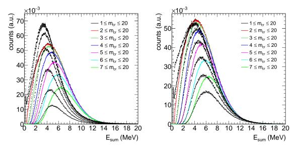
Figure 4.41: PFG spectra (dashed lines) using the model of Valentine [103] (left) and a modified model based on Valentine with modified parameters [104] used in a previous  $^{233}U(n,\gamma)$  measurement at n\_TOF (right) compared to the experimental data (solid lines).
