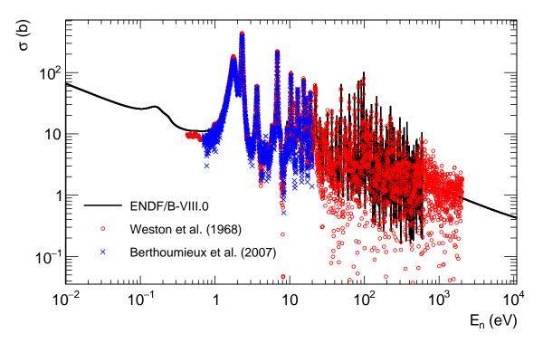
Figure 1.5: The two data sets of  $^{233}U(n,\gamma)$  from EXFOR compared to the ENDF/B-VIII.0 evaluation.
