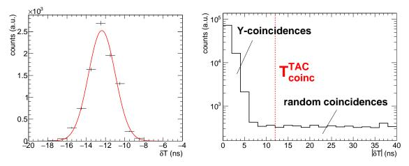
Figure 4.10: Time differences between signals from the reference detector and detector 7 where  $E_{Sum} \approx 2.7 \,\text{MeV}$ . The timing offset between those two detectors equals the centroid of the Gaussian fit of  $-12.4 \,\text{ns}$  (left). Time offset corrected time differences - the optimal coincidence window  $T_{coinc}^{TAC}$  is indicated at 12 ns (right).
