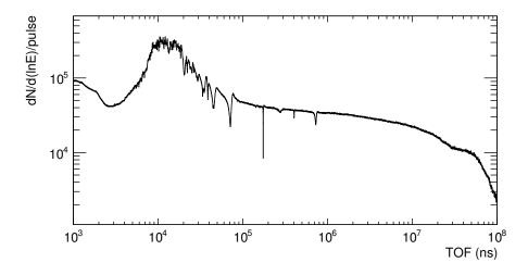
Figure 4.16: Neutron fluence in EAR1 at 185 m flight path from FLUKA simulations in isolethargic units. Note the increased fluence in the region  $5 \,\mu s < TOF < 15 \,\mu s$ .
