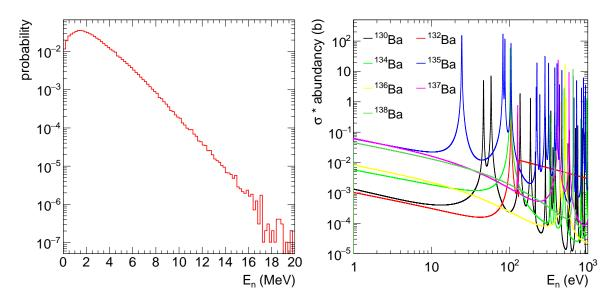
Figure 5.10: Fission neutron energy spectrum of <sup>233</sup>U taken from ENDF/B-VIII.0 (left). Capture cross sections of all stable barium isotopes weighted by their natural abundance (right).
