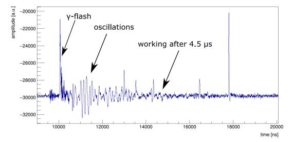
Figure 3.17: Reponse of the FICH to the  $\gamma$ -flash. A time-of-flight of 4.5 µs corresponds to a neutron energy of roughly 7 MeV.
