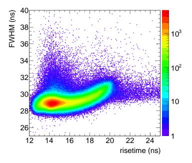
Figure 4.19: Fission fragment (amp>3000) signal shape parameters from FICH channel 4 reading only from a single <sup>233</sup>U deposit.
