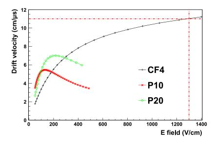
Figure 3.15: GARFIELD simulations of the electron drift velocities for different experimental gases at atmospheric pressure as a function of the applied electric field taken from Ref. [83].
