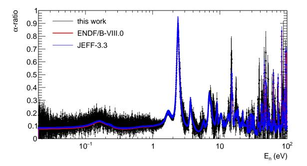
Figure 6.6: Experimental  $^{233}$ U  $\alpha$ -ratio calculated from events with  $3 \leq m_{cr} \leq 7$  and 2.5 MeV  $< E_{sum} <$  7 MeV compared to the  $^{233}$ U  $\alpha$ -ratio from ENDF/B-VIII.0 and JEFF-3.3 up to 100 eV. No dead time corrections have been applied.
