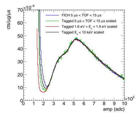
Figure 4.34: Pulse-height spectra of the events in the fission chamber for  $5 \,\mu s < TOF < 15 \,\mu s$  compared to tagged events for different  $TOF/E_n$  regions.
