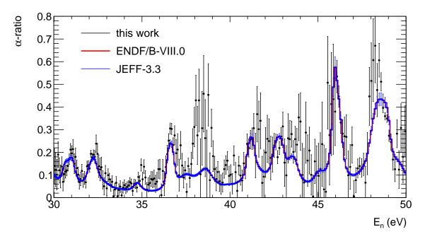
Figure 6.11: Comparison of the point wise experimental  $^{233}$ U  $\alpha$ -ratio to the  $^{233}$ U  $\alpha$ -ratio from ENDF/B-VIII.0 and JEFF-3.3 in the neutron energy region from 30 eV to 50 eV. No dead time corrections have been applied.
