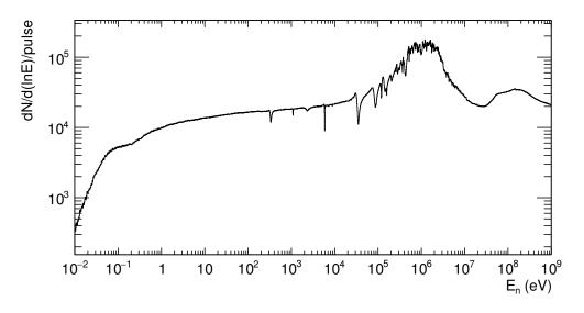
Figure 3.3: Neutron fluence in EAR1 from FLUKA simulations in isolethargic units.
