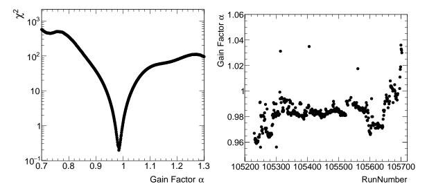
Figure 4.6:  $\chi^2$  for various gain factors  $\alpha$  for BaF<sub>2</sub> module 7 and Runnumber 105570 (left). Gain variation over time for BaF<sub>2</sub> module 7 (right).
