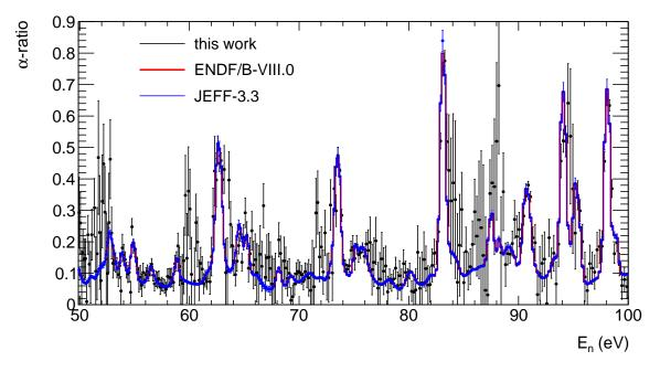
Figure 6.12: Comparison of the point wise experimental  $^{233}$ U  $\alpha$ -ratio to the  $^{233}$ U  $\alpha$ -ratio from ENDF/B-VIII.0 and JEFF-3.3 in the neutron energy region from 50 eV to 100 eV. No dead time corrections have been applied.
