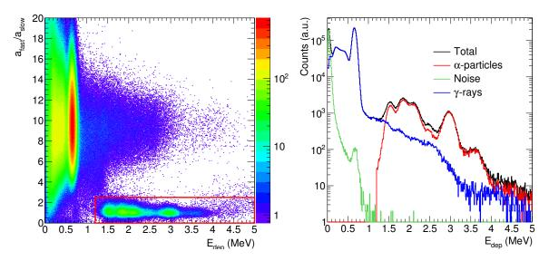
Figure 4.2: Particle discrimination of  $\alpha$ -particles in a BaF<sub>2</sub> crystal with improved  $\alpha$ -particle cut indicated by the red framed region (left). Contributions to the total spectrum in a crystal (right) measured with a <sup>137</sup>Cs calibration source (approx. 340 kBq).
