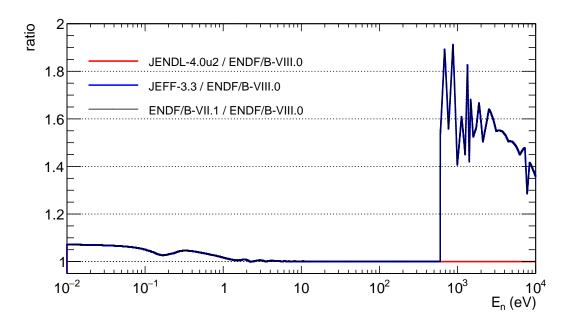
Figure 1.6: Comparison of the  $^{233}U(n,\gamma)$  cross section ratios between several evaluated libraries and the ENDF/B-VIII.0 library. Significant discrepancies can be seen in the URR above 600 eV while deviations within 8 % are observed for neutron energies below 10 eV.
