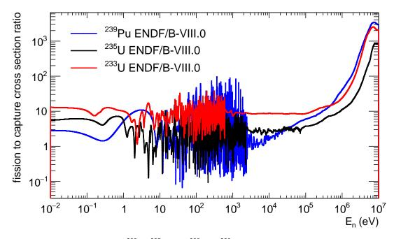
Figure 1.3: Inverse  $\alpha$ -ratio for <sup>233</sup>U, <sup>235</sup>U and <sup>239</sup>Pu. <sup>233</sup>U has the largest inverse  $\alpha$ -ratio leading to a reduction in the amount of transuranic waste per energy unit produced.
