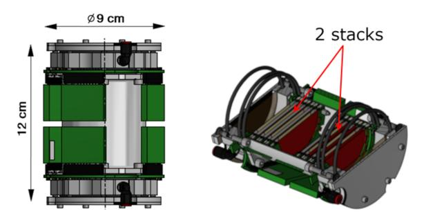
Figure 3.12: 3D-CAD drawing of the fission chamber and a sectional view. The green blocks around the chamber represent the preamplifiers.
