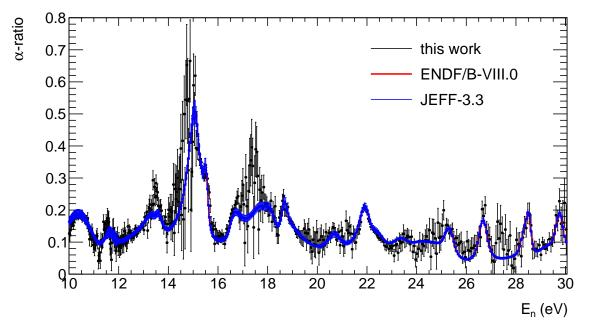
Figure 6.10: Comparison of the point wise experimental  $^{233}$ U  $\alpha$ -ratio to the  $^{233}$ U  $\alpha$ -ratio from ENDF/B-VIII.0 and JEFF-3.3 in the neutron energy region from 10 eV to 30 eV. No dead time corrections have been applied.
