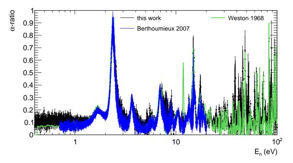
Figure 6.14: Comparison of the point wise experimental  $^{233}$ U  $\alpha$ -ratio from this work and from the experimental data sets from Weston and Berthoumieux up to 100 eV. No dead time corrections have been applied.
