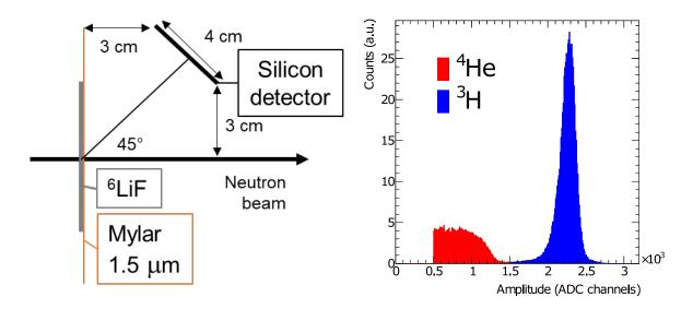
Figure 3.7: Scheme of the SiMon detector (left, from [79]) and the pulse height spectrum (right), where the alpha region and the triton peak are nicely separated.
