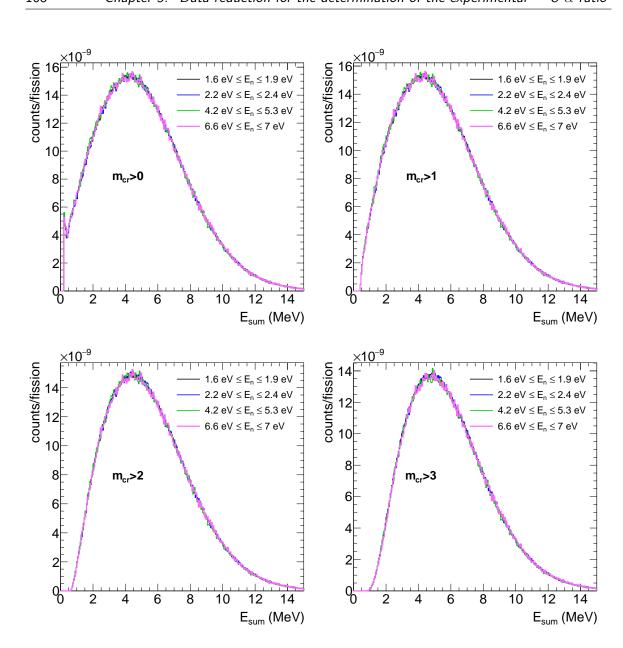
Figure 5.7: Comparison of the sum energy spectra of the prompt fission response for different multiplicity conditions. No difference is observed with the incident neutron energy.
