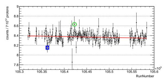
Figure 4.24: Gain drift over time: number of events with amp > 3500 adc units per protons per Run - typically 4 hours make a Run. The red line is a linear fit to the data points, with  $p_0 = 27.0097$  and  $p_1 = -1.77E - 4$ .
