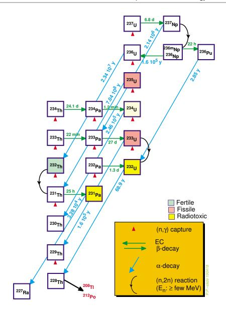
Figure 1.2: Schematic view of the Th-U fuel cycle [19].
