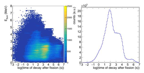
Figure 5.5: Sum energy and time distribution of the decay of fission products simulated with GEANT4 (left). Time distribution of fission product decay events with  $m_{cr} > 2$  and 2.5 MeV  $< E_{Sum} <$  7 MeV.
