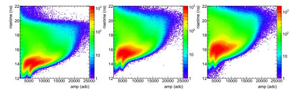
Figure 4.21: Rise time versus amplitude of FICH signals from the two single <sup>233</sup>U deposit FICH channels 4 (left) and 8 (middle) and FICH channel 7 (right) reading signals from two ionization cells. For short rise times (i.e.  $cos\theta_{LAB}^{FF} \approx 1$ ) the light and heavy fission fragment peaks become visible.
