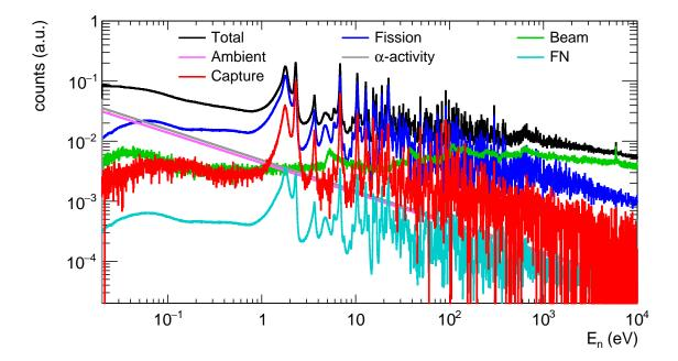
Figure 6.2: Experimental response of the TAC to the different components obtained either by direct measurement or subtraction of components from the total response for events with  $3 \le m_{cr} \le 7$  and  $2.5 \text{ MeV} < E_{sum} < 7 \text{ MeV}.$
