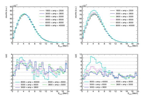
Figure 5.18: Sum energy spectra for different amplitude cuts normalized to the total integral (left) and normalized in the tail of the distribution ( $E_{sum} > 10 \text{ MeV}$ ) (right). In the bottom panels the ratios of the corresponding amplitude regions to the region 1800 < amp(adcunits) < 2500 are shown.
