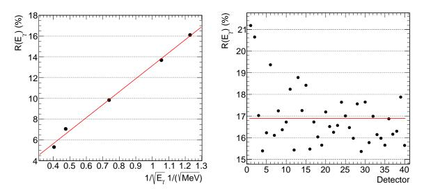
Figure 4.8: Energy resolution for BaF<sub>2</sub> module 7 - smaller  $E_{\gamma}$  are on the upper end of the x-axis (left). Energy resolution of all detectors at  $E_{\gamma} = 0.662 \text{ MeV}$  from <sup>137</sup>Cs. The average (red line) of all crystals is calculated to  $R(E_{\gamma} = 0.662 \text{ MeV}) \approx 16.9\%$  (right).
