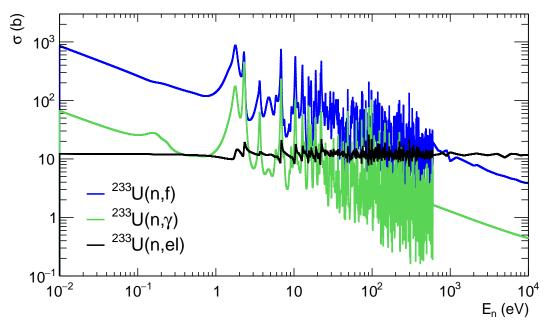
Figure 2.4:  ${}^{233}U(n,\gamma)$ ,  ${}^{233}U(n,\gamma)$  and  ${}^{233}U(n,n)$  cross sections from ENDF/B-VIII.0.
