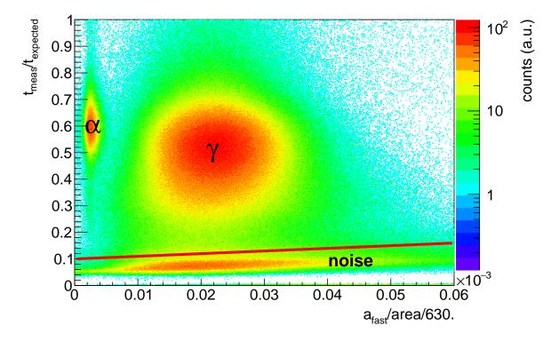
Figure 4.1: Particle discrimination in  $BaF_2$ . The region below the red line corresponds to noise. The upper left hotspot corresponds to  $\alpha$ -particles while the central region corresponds to  $\gamma$ -rays.
