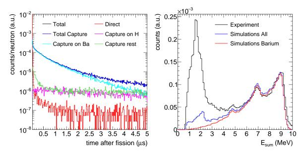
Figure 5.11: Distribution of events with  $m_{cr} > 2$  registered in the TAC (simulated) as a function of the time after neutron emission (left). Comparison of the simulated and experimental sum energy response of the TAC to fission neutrons for events with  $m_{cr} > 2$  and 14 ns  $< \delta T < 1 \,\mu$ s (right).
