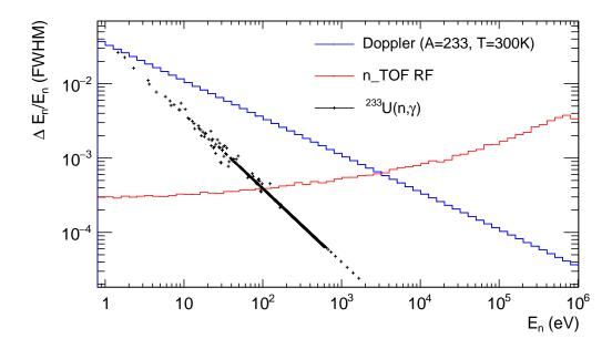
Figure 3.5: Comparison of the effects of Doppler Broadening (T = 297 K) for <sup>233</sup>U and of the n\_TOF resolution function on the resolution of the <sup>233</sup>U  $\alpha$ -ratio measurement. The resonance widths  $\Gamma_{\gamma}$  of the <sup>233</sup>U(n, $\gamma$ ) resonances according to ENDF/B-VIII.0 are plotted.
