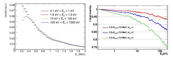
Figure 6.3: Individual  $\gamma$ -ray energies in the prompt fission cascades for different neutron energy intervals from this work (left). Decrease of the efficiency with neutron energy in the  $^{235}U(n,\gamma)$  cross section measurement [60, 107] performed at n\_TOF applying the fission tagging technique taken from [107] (right).
