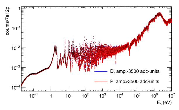
Figure 4.28: Count rate in the FICH normalized to a standard proton pulse for dedicated and parasitic beam types.
