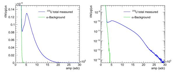
Figure 4.15: Pulse height spectra of the events in the fission chamber with and without beam in linear (left) and logarithmic (right) scale. Only events with  $E_n < 10$  keV are considered.
