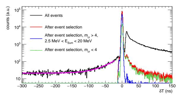
Figure 4.30: Time difference distribution between TAC and FICH events for a maximum allowed coincidence window  $T_{coinc}^{TAC-FICH} = 1 \,\mu s$ . The features of the distribution are explained in the text.
