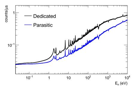
Figure 4.13: Count rate in the TAC for dedicated and parasitic beam types.
