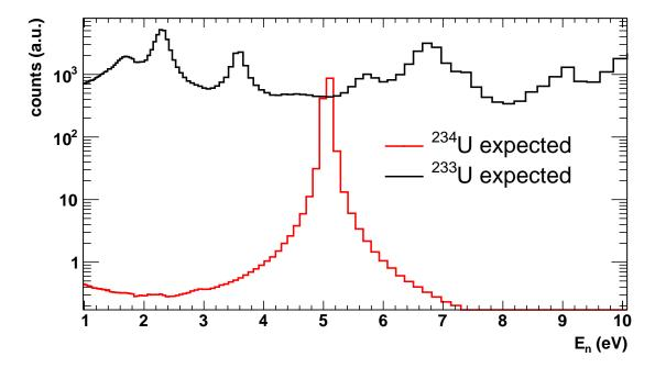
Figure 3.19: Expected counts from <sup>233</sup>U and <sup>234</sup>U according to the isotopic composition using the capture cross-sections from ENDF/B-VIII.0.
