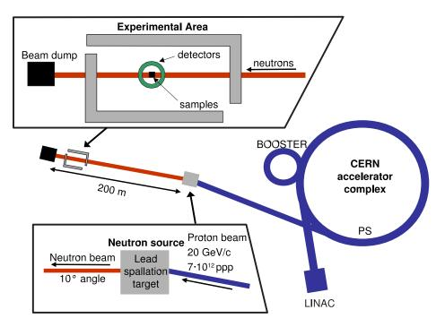
Figure 3.1: Schematical overview of the n\_TOF facility at CERN, only showing experimental area 1, picture taken from [65].
