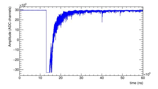
Figure 3.6: Example of the response of a BaF<sub>2</sub> module to the  $\gamma$ -flash.
