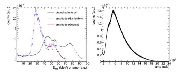
Figure 4.37: Deposited energy and calculated amplitude of fission fragments from a  $U_3O_8$  layer with a density of  $8.2 \text{ g/cm}^3$  and an areal density of  $\sigma = 305 \,\mu\text{g/cm}^2 \,{}^{233}\text{U}$  (left). Experimental amplitude spectra of FICH channel 4 with an areal density of  $\sigma = 305 \,\mu\text{g/cm}^2 \,{}^{233}\text{U}$  (right).
