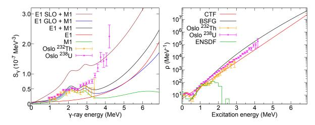
Figure 5.21: Photon strength function used to reproduce the experimental <sup>234</sup>U  $\gamma$ -ray decay (black, red, green) [109] compared to suggested model as defined in the RIPL-3 data base [110] (brown and blue lines, SLO/GLO in the legend) and other data sets from the Oslo group (left). Two level density models compared to experimental data from the Oslo group and experimental level counting from ENSDF (right), for detailed explanation see section 5.4.1.
