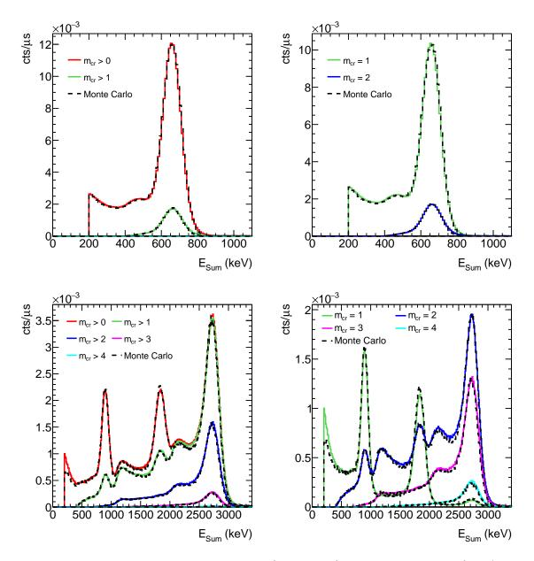
Figure 3.22: Comparison between simulated results (dashed lines) and experimental data (solid/colored lines) for the <sup>137</sup>Cs (top) <sup>88</sup>Y (bottom) calibration source including the absorber.
