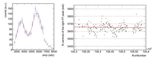
Figure 4.26: Using the rise time gates from Table 4.3 the heavy and the light fission fragment peaks can be fitted with gaussians (left). The centroid of the fit to the light FF peak in FICH channel 4 during all runs of the <sup>233</sup>U  $\alpha$ -ratio campaign. The red line is a linear fit to the data points, with  $p_0 = 9751.77$  and  $p_1 = -3.887E - 2$ . (right).
