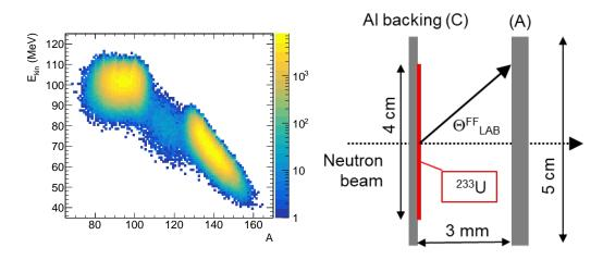
Figure 4.35: Fission fragment distribution for thermal fission of <sup>233</sup>U according to the GEF code (left). Schematic illustration of the ionization cell geometry used in GEANT4 simulations (right).
