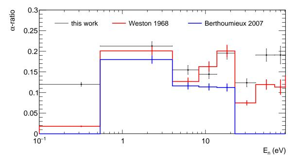
Figure 6.20: Comparison of the average values of the experimental, Weston and Berthoumieux  $^{233}$ U  $\alpha$ -ratio for neutron energy intervals according to the 33 group energy structure of the WPEC Subgroup 33 (SG33) [120] The corresponding values are summarized in Table 6.5.
