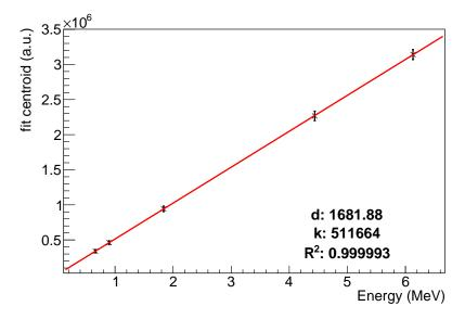
Figure 4.4: Calibration curve for  $BaF_2$  module 7.
