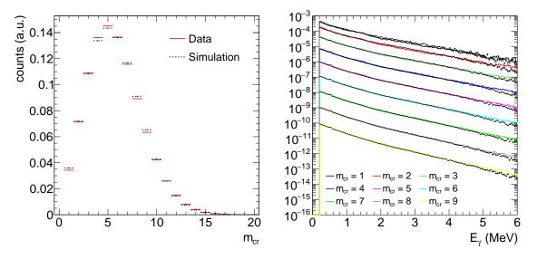
Figure 4.45: Comparison of the experimental (colored/solid lines) and simulated (dashed lines) PFG crystal multiplicity  $m_{cr}$  spectra (left) and the individual  $\gamma$ -ray energy  $E_{\gamma}$  spectra (right). The  $E_{\gamma}$  spectra have arbitrary scaling factors for better visualization. The DANCE PFG cascade generator was used with optimized parameters.
