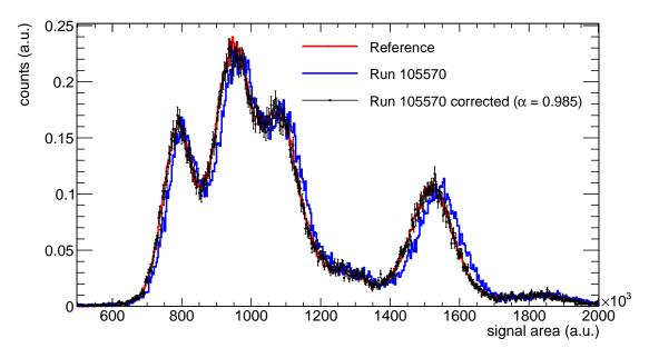
Figure 4.5: Illustration of the gain correction method for  $BaF_2$  module 7.
