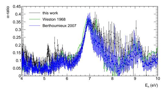
Figure 6.16: Comparison of the point wise experimental  $^{233}$ U  $\alpha$ -ratio from this work and from the experimental data sets from Weston and Berthoumieux in the neutron energy region from 4 eV  $< E_n <$  10 eV. The experimental data from this work shows a structure at 5.15 eV as expected due to the 0.0496 %  $^{234}$ U contamination of the samples, see section 3.4.
