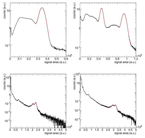
Figure 4.3: Response of  $BaF_2$  module 7 to the standard calibration sources - <sup>137</sup>Cs (top left), <sup>88</sup>Y (top right), AmBe (bottom left), CmC (bottom right). Fits to the experimental data in red using different fitting functions.
