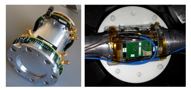
Figure 3.13: Pictures of the dummy fission chamber in the lab (left) and the <sup>233</sup>U loaded fission chamber with electronics and gas connected and embedded in one half of the absorber inside the TAC (right).
