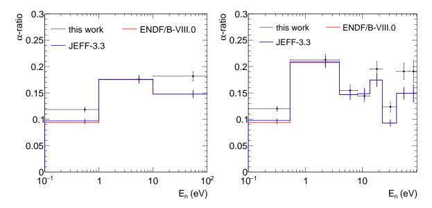
Figure 6.13: Comparison of the average values of the experimental, ENDF/B-VIII.0 and JEFF-3.3  $^{233}$ U $\alpha$ -ratio for neutron energy decades (left) and neutron energy intervals according to the 33 group energy structure of the WPEC Subgroup 33 (SG33) [120] (right) The corresponding values are summarized in Table 6.2. No dead time corrections have been applied.
