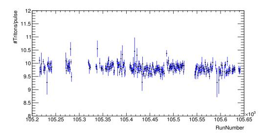
Figure 3.8: Averaged number of tritons per standard proton pulse per run during the whole experimental campaign.
