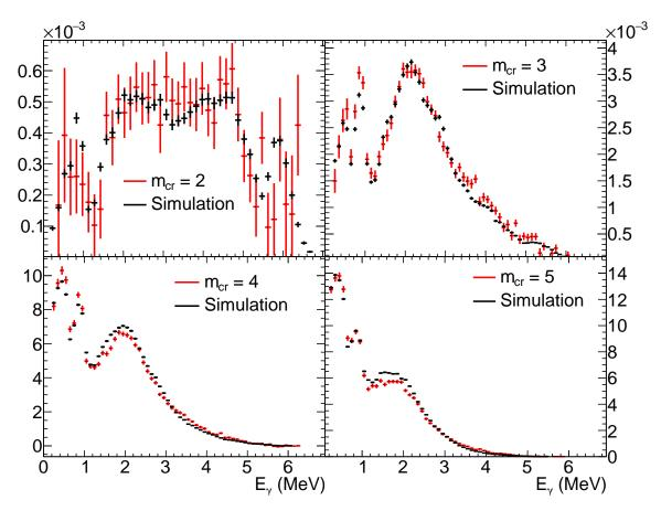
Figure 5.23: Comparison of the experimental and simulated  $\gamma$ -ray energies  $E_{\gamma}$  for capture events with 6.4 MeV  $< E_{sum} <$  7 MeV.
