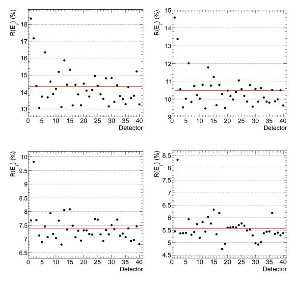
Figure 4.9: Energy resolution of all detectors at various  $E_{\gamma}$ : 0.898 MeV (top left), 1.836 MeV (top right), 4.438 MeV (bottom left), 6.130 MeV (bottom right). The average values are indicated in red and summarized in Table 4.2.
