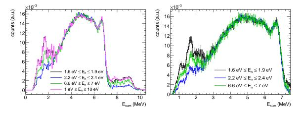
Figure 5.9: Sum energy spectra for TAC events with  $m_{cr} > 2$  in several neutron energy intervals without (left) and with (right) statistical errors displayed. The spectra have been normalized in the region 3.5 MeV  $< E_{Sum} < 7$  MeV to compare the shapes.
