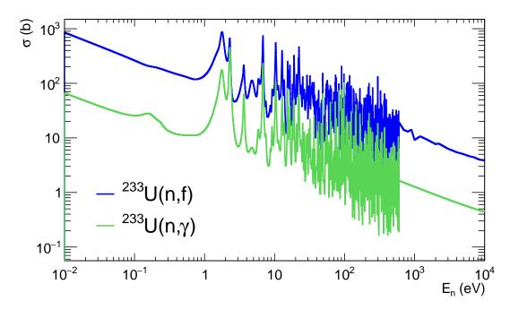
Figure 1.7: Capture and fission cross section of <sup>233</sup>U in the ENDF/B-VIII.0 evaluated library. Note the end of the resolved resonance region at 600 eV.
