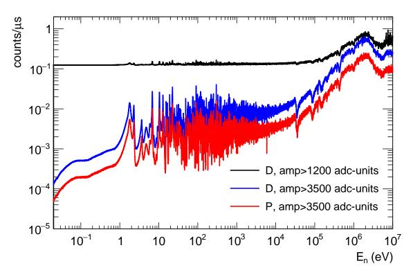
Figure 4.27: Count rate in the FICH for dedicated and parasitic beam types and different amplitude cuts.
