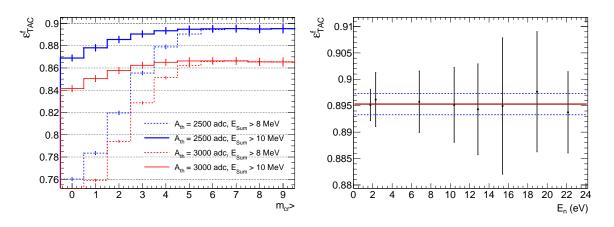
Figure 5.16: Fission tagging efficiency  $\varepsilon_{TAC}^{f}$  as a function of the crystal multiplicity and sum energy for two different amplitude thresholds  $A_{th}$  in the neutron energy interval from 1.6 eV to 1.9 eV (left). Fission tagging efficiency calculated in several neutron resonances for  $A_{th} = 2500$  adc units,  $m_{cr} > 6$  and  $E_{Sum} > 10$  MeV, their average (red line) and the associated error of the average (blue dashed lines) (right).
