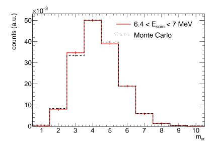
Figure 5.24: Comparison of the experimental and simulated crystal multiplicity distribution for capture events with 6.4 MeV  $< E_{sum} < 7$  MeV.
