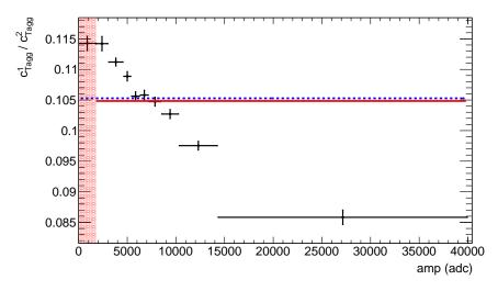
Figure 5.19: Ratio between the number of tagged fission counts with restrictive (1,  $E_{Sum} > 10 \text{ MeV}$  and  $m_{cr} > 6$ ) and relaxed conditions (2, 2.5 MeV  $< E_{Sum} < 7 \text{ MeV}$  and  $3 \le m_{cr} \le 7$ ) as a function of the FICH signal amplitude. The red and blue lines indicate the averages of the points in their respective intervals.
