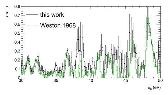
Figure 6.18: Comparison of the point wise experimental  $^{233}$ U $\alpha$ -ratio from this work and from the experimental data sets from Weston in the neutron energy region from 30 eV  $< E_n < 50$  eV. No dead time corrections have been applied.
