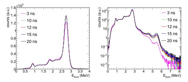
Figure 4.11: Sum energy spectra of the <sup>88</sup>Y calibration source using different time coincidence windows in linear (left) and logarithmic (right) scale.
