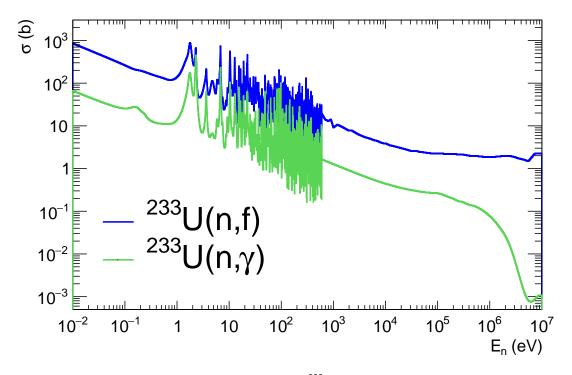
Figure 2.1: Capture and fission cross section of <sup>233</sup>U in the ENDF/B-VIII.0 evaluated library.
