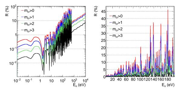
Figure 5.4: Ratio of expected scattered neutron and  $^{233}U(n,\gamma)$  events depending on the neutron energy and crystal multiplicity for events with 2.5 MeV  $< E_{Sum} < 7$  MeV.
