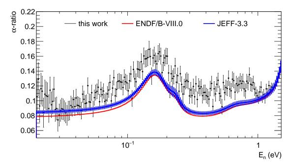
Figure 6.7: Comparison of the point wise experimental  $^{233}$ U  $\alpha$ -ratio compared to the  $^{233}$ U  $\alpha$ -ratio from ENDF/B-VIII.0 and JEFF-3.3 for the low energy region from 0.02 eV to 1.5 eV.
