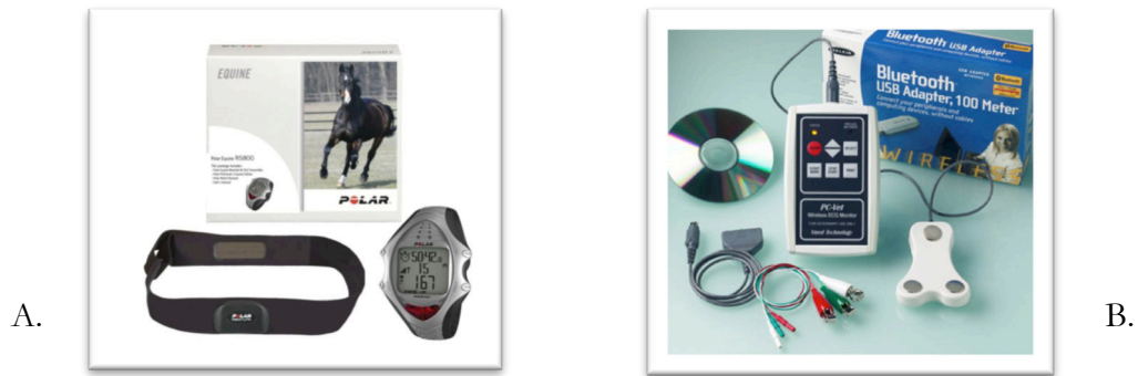
Figure 5. Devices to measure the cardiac activity: Polar Equine RS800CX® (A), PC-Vetgard®+tm Multiparameter wireless system for telemetric measurements (B).
