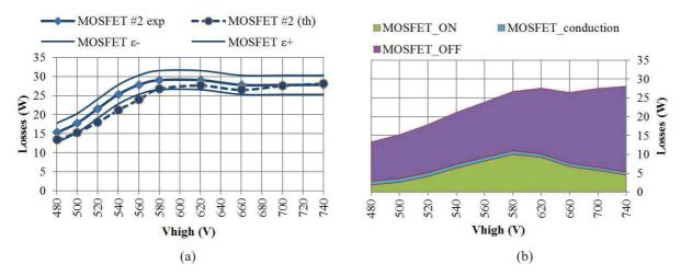
Figure 10: MOSFET losses: (a) comparison between experimental measurements (measurement errors being the small lines) and analytical model, (b) MOSFET losses in each phase ratio
