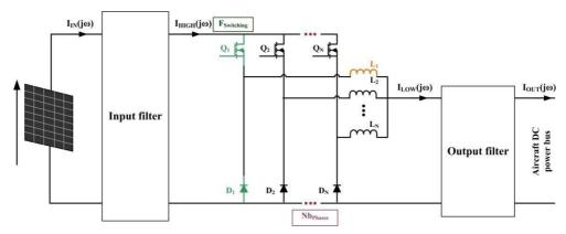
Figure 24: IBC schematic to represent the computed spectra
