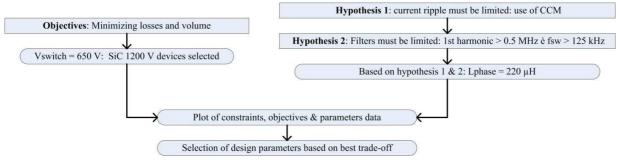
Figure 5: Design of IBC using sequential method summary
