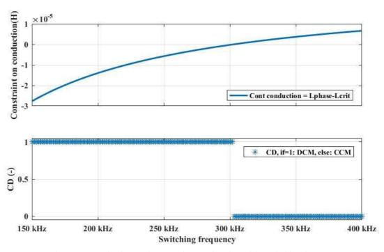
Figure 19: Conduction mode constraint as a function of the switching frequency
