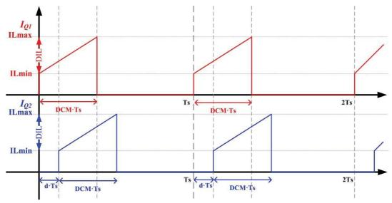
Figure 25: IBC current waveforms in the MOSFETs
