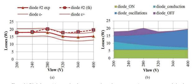
Figure 14: Diode losses: (a) comparison between experimental measurements (measurement errors being the small lines) and analytical model, (b) diode losses in each phase ratio
