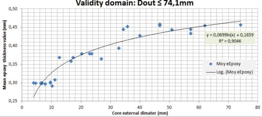
Epoxy thickness:  $eEpoxy := 0.0699 \cdot ln \left( \frac{Lphase\_Dout}{mm} \right) \cdot mm + 0.1659 \cdot mm = 0.413 \cdot mm$
