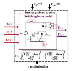
Figure 5: Identification of stray elements by optimization method
