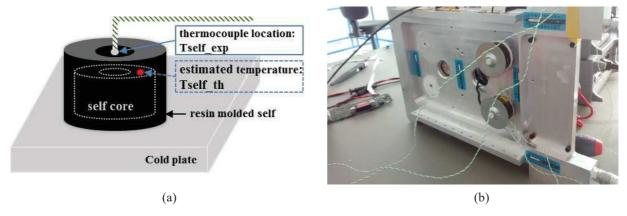
Figure 8: Inductor external temperature measurement, (a) schematic, (b) picture
