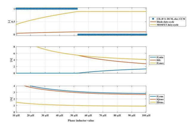
Figure 18: Impact of condition "if" and conduction mode on IBC waveforms model outputs as a function of the phase inductor value
