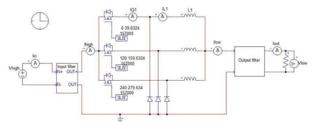
Figure 26: Time simulation schematic of a 157 kHz 3-phases IBC working at 1484 W, 700V to 200 V
