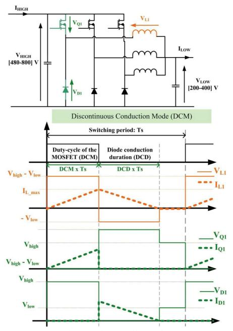
Figure 1: Buck converter ideal waveforms
