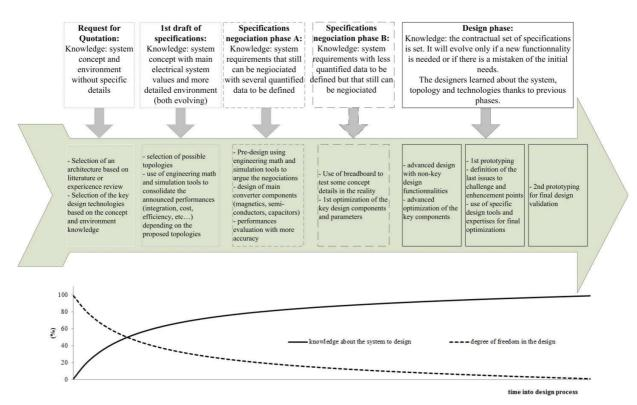
Figure 5: Pre-design and design phases conduct in power electronics
