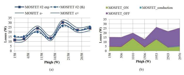
Figure 17: MOSFET losses: (a) comparison between experimental measurements (measurement errors being the small lines) and analytical model, (b) MOSFET losses in each phase ratio
