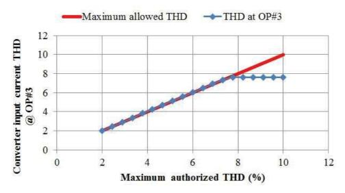
Figure 10: Converter input current THD for the operating point #3
