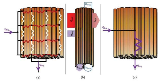
Figure 20: Definition of Litz wire thermal conductivities. (a) Path of different heat sources, (b) the transverse and longitudinal resistances set as a thermal network inside the Litz wire, (c) definition of the longitudinal equivalent thermal resistance with a conductivity of  $k_{leq}$  substituing the thermal network in (b).
