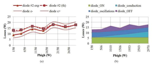
Figure 18: Diode losses: (a) comparison between experimental measurements (measurement errors being the small lines) and analytical model, (b) diode losses in each phase ratio
