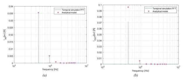
Figure 31: Comparison between temporal simulation FFT and analytical input (a) and output (b) current disturbances models
