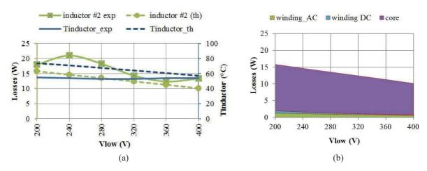
Figure 16: Phase inductor losses and temperatures: (a) comparison between experimental measurements (measurement errors being the small lines) and analytical model, (b) inductor winding and core losses theoretical ratio
