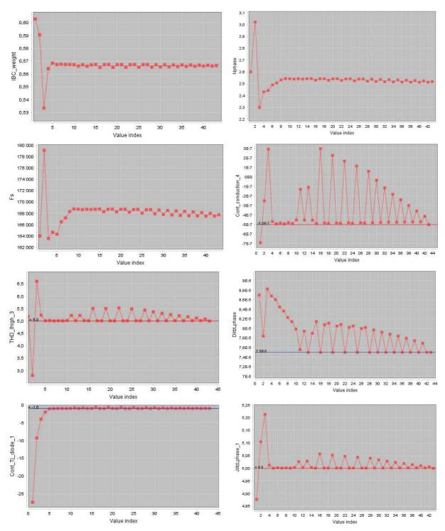
Figure 2: Optimization of the IBC in DCM with MPP 26µ material on the initial set of specifications
