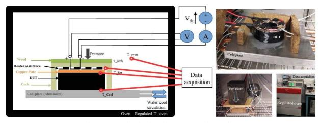
Figure 17: Test bench schematic: top, set-up pictures: bottom
