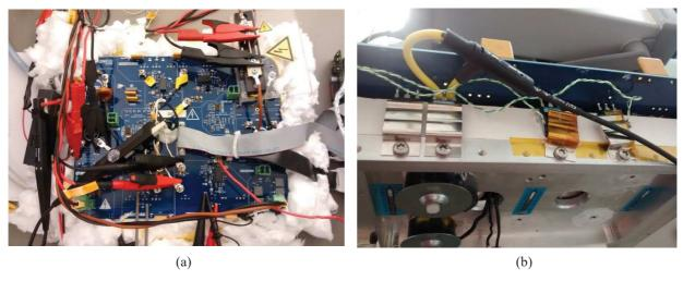
Figure 7: Prototype pictures: (a) top view with probes and thermal fiber, (b) aside view of semiconductors of switching cell #1 (at the left of the picture) and #2 (at the right of the picture)
