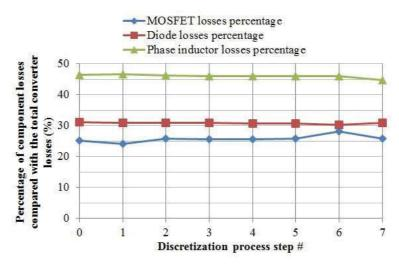
Figure 7: Evolution of the losses ratio of the power components
