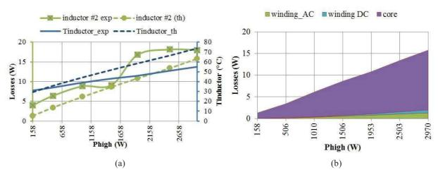
Figure 19: Phase inductor losses and temperatures: (a) comparison between experimental measurements (measurement errors being the small lines) and analytical model, (b) inductor winding and core losses theoretical ratio
