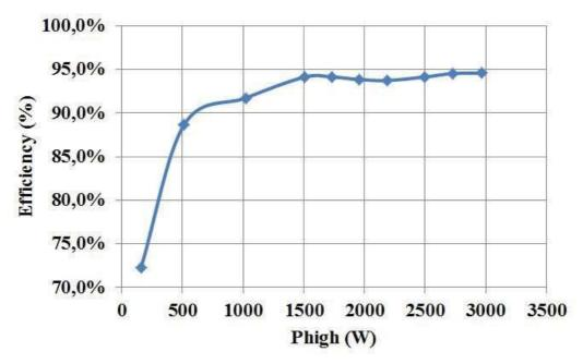
Figure 22: Measured efficiency of a 3-Phases IBC in DCM mode
