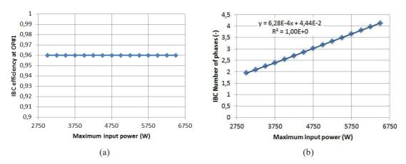
Figure 3: IBC (a) efficiency, (b) optimal number of phases evolution, during the parameterized optimization of the converter maximum power
