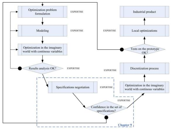
Figure 1: Flowchart of the preliminary design in the imaginary world approach
