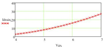
It is quite different from the curve given in the datasheet, since the scale given in the datasheet is not convenient: the threshold voltage is given for few mA when the gradutation is in A. It conducts into a bad interpolation. Besides, the curve given in the datasheet is for Vds=Vgs<20V while we use these parameters for Vds > 200 V... So it is not really meticulous but it seems that the model gives quite good results so it may not have a lot of influence...
