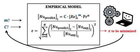
Figure 5: Identification by optimization of model parameters
