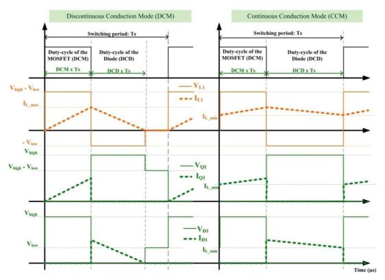
Figure 5: Interleaved Buck Converter schematic and components ideal current and voltage waveforms
