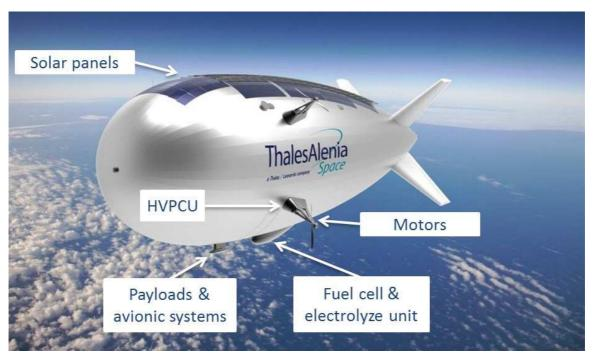
Figure 1: Stratobus airship illustration
