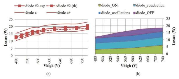
Figure 11: Diode losses: (a) comparison between experimental measurements (measurement errors being the small lines) and analytical model, (b) diode losses in each phase ratio
