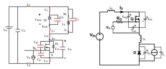
Figure 4: Switching cell under study in [1] paper
