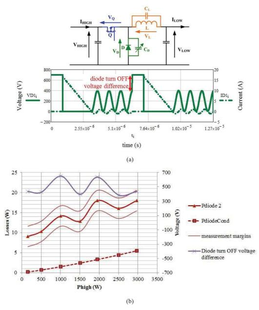
Figure 7: SiC Schottky diode in a 3-phase IBC (a) theorical waveforms at Phigh = 2.5 kW, Vhigh = 700 V and Vlow = 200 V, (b) losses measurement (Pdiode2) with its error margins, theoretical conduction losses (evaluated with Eq. 2) and the measured diode turn OFF voltage difference (as shown in picture (a) for the operating point Vhigh = 700 V to Vlow = 200 V, input power Phigh being swept
