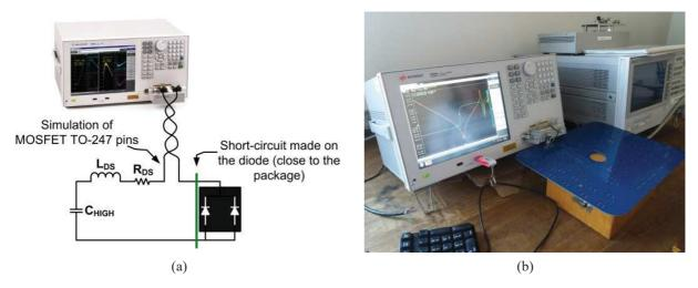
Figure 3: PCB inductance measurement (a) schematic, (b) picture
