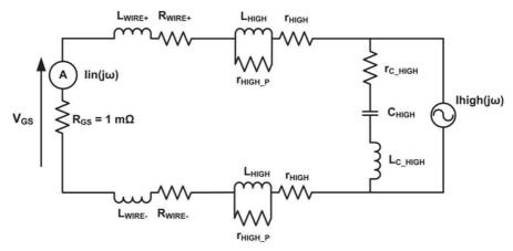
Figure 29: Input filter and wires of the IBC frequency circuit model
