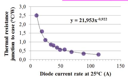
Thermal exchange surface (TO-247 case):
