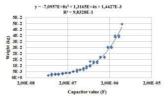
Figure 10: Example of weight interpolation of capacitor
