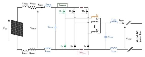
Figure 7: IBC to optimize schematic
