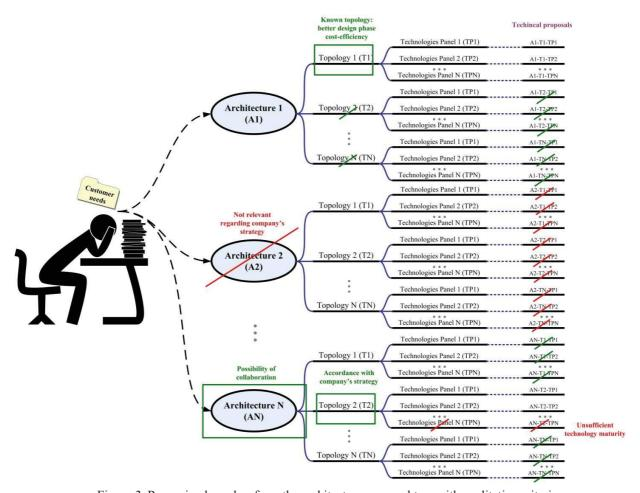
Figure 2: Removing branches from the architecture proposal tree with qualitative criteria
