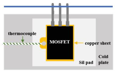
Figure 6: Semiconductor case temperature measurement schematic
