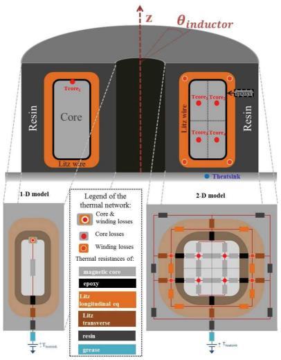
Figure 16: Phase inductor 1-D or 2-D thermal models
