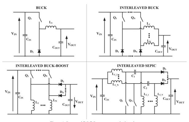
Figure 4: Compared DC-DC converter topologies schemes
