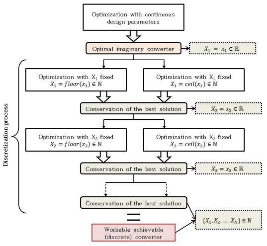
Figure 1: Heuristic discretization process with  $X_n$  the  $n^{th}$  discrete variable, with the objective function more sensitive to  $X_1$  than  $X_2$ , etc.
