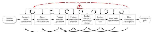
Figure 2: Pre-design process according Ulrich and Eppinger [3]
