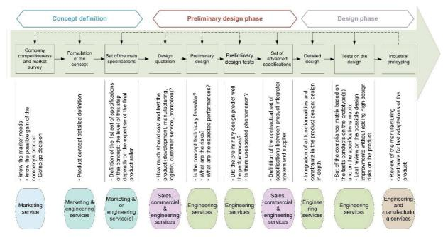
Figure 4: Design process in power electronics
