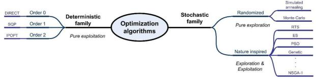
Figure 4: Optimization algorithm non-exhaustive classification tree
