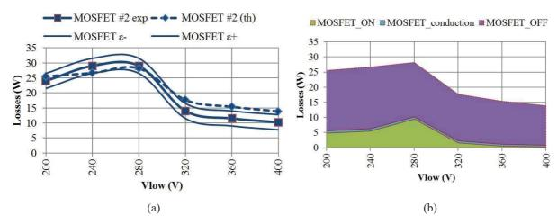
Figure 13: MOSFET losses: (a) comparison between experimental measurements (measurement errors being the small lines) and analytical model, (b) MOSFET losses in each phase ratio
