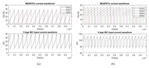
Figure 23: Interleaved Buck Converter MOSFETs and input current waveforms: (a) 3-phases IBC in DCM, (b) 4-phases IBC in CCM
