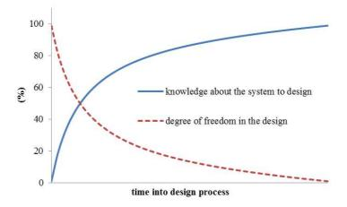
Figure 3: Design process paradox
