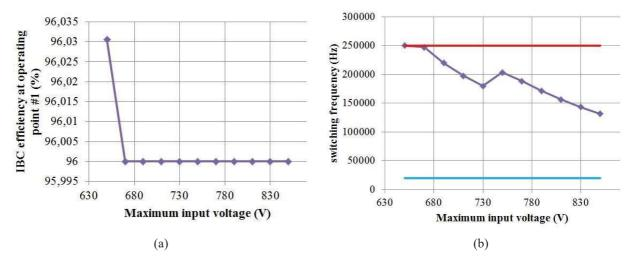
Figure 6: Evolution of the (a) converter efficiency of operating point #1, (b) switching frequency value, as a function of the maximum input voltage of the converter
