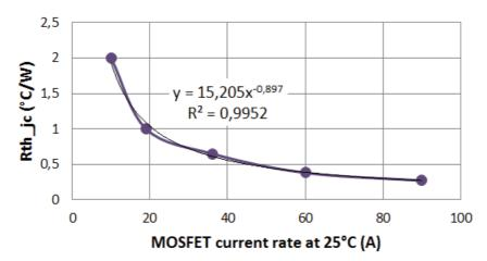
Thermal exchange surface (TO-247 case):
