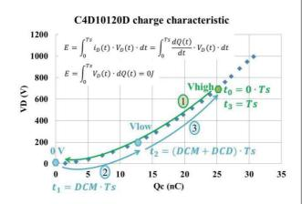
Figure 8: Illustration of the charging and discharging of the diode junction capacitance in a Buck converter working in DCM
