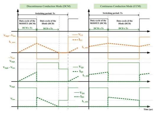
Figure 17: Single phase Buck converter waveforms
