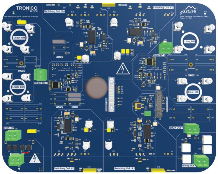
Figure 1: Prototype printed circuit board 3D view from CAO software
