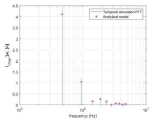
Figure 32: Comparison between temporal simulation FFT and analytical models of the current spectrum in the output filtering capacitor
