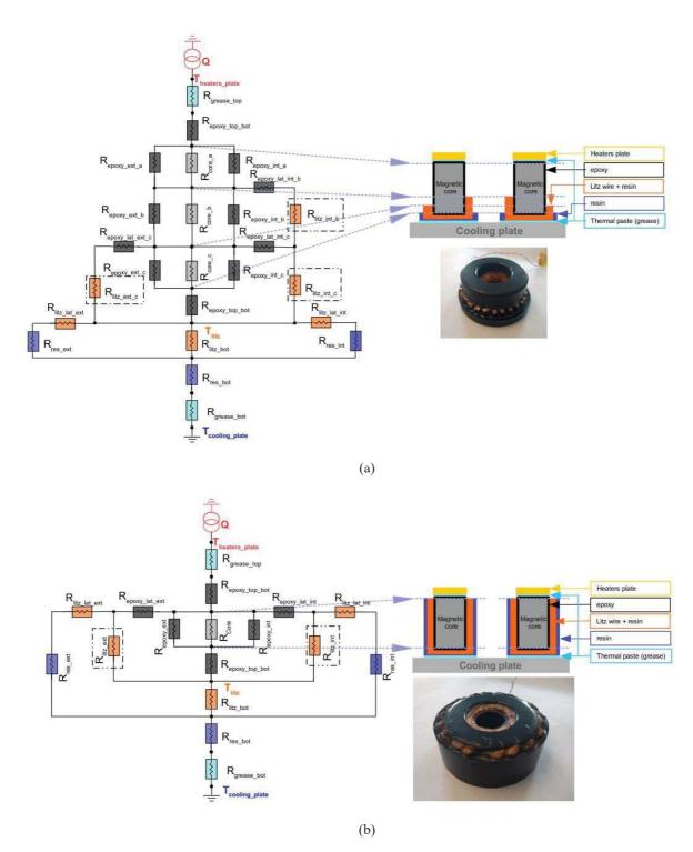
Figure 21: Thermal network models for samples 1 to 4 (a), and 5-6 (b), showing thermal resistances corresponding to the core material (light grey), epoxy (dark grey), grease (light blue), resin (dark blue) and Litz wire (orange). Litz wire thermal resistances calculated using the equivalent longitudinal conductivity are surrounded by dashed rectangle; the other Litz wire thermal resistances are calculated using the transverse conductivity.
