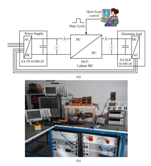
Figure 5: Electrical power test bench: (a) schematic, (b) picture
