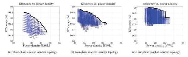
Figure 9: Feasible and Pareto-optimal designs for the three topologies under investigation in terms of efficiency and power density with Tcore  $\leq 155$  °C from [4]
