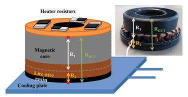
Figure 19: Measured thermal resistances on the DUT
