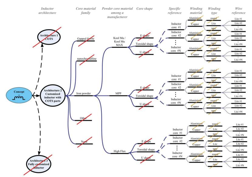
Figure 8: Architecture proposals tree for the IBC phase inductor
