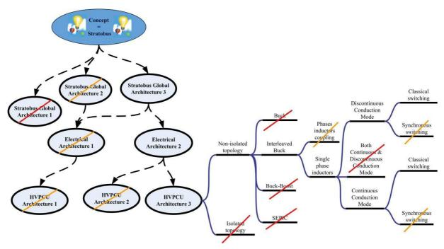
Figure 6: HVPCU DC-DC converters architecture proposals tree
