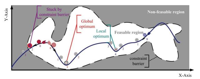
Figure 9: Illustration of optimal point search using a gradient-based optimization algorithm
