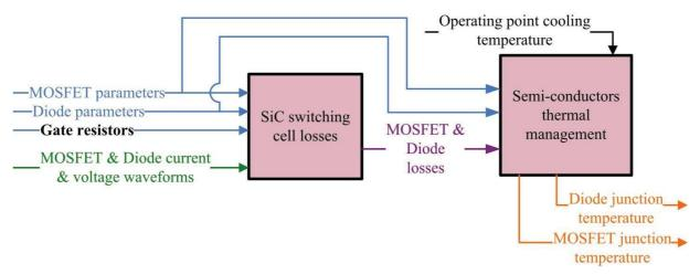
Figure 2: IBC switching cell losses and thermal models schematic
