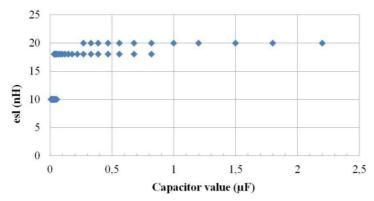
Figure 12: Parasitic inductance value of the capacitors taken in the datasheet (depends on the lead spacing, industrially discretized)
