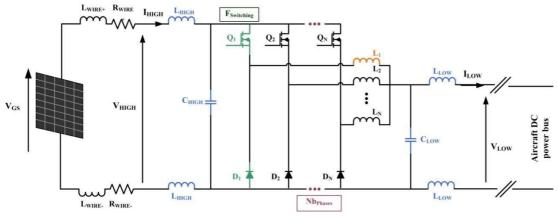
Figure 1: IBC to optimize schematic
