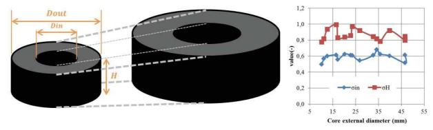
Figure 15: Core dimension coefficients value from the manufacturer catalog
