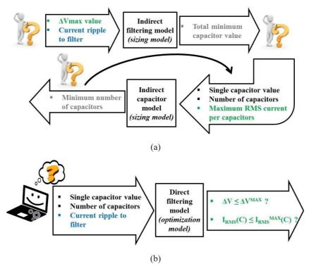
Figure 2: Illustration of sizing (a) and optimization (b) models
