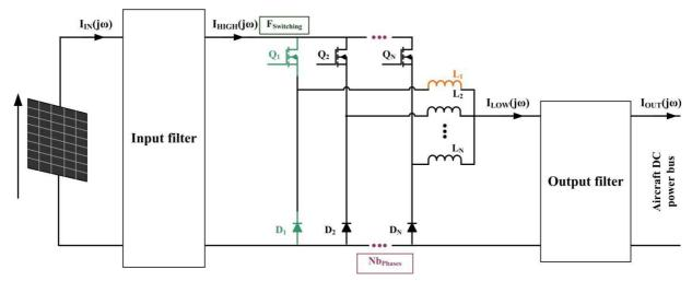
Figure 28: Interleaved Buck Converter schematic
