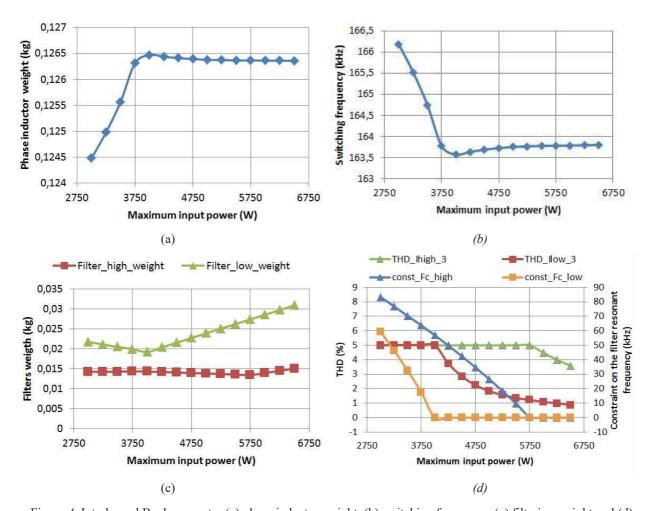
Figure 4: Interleaved Buck converter (a) phase inductor weight, (b) switching frequency, (c) filtering weight and (d) input and output currents THD at OP#3 (must be < 5%) and constraints on filters resonant frequency (must be > 0 kHz), as function of its maximum input power
