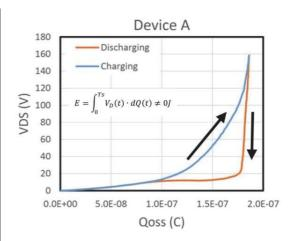
Figure 9: VDS versus QOSS of Super-Junction MOSFET curve measured with the Sawyer-Tower circuit at F = 10 kHz and Vpk-pk = 160 V from [6]
