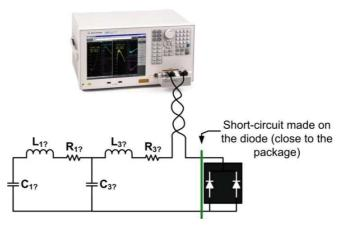
Figure 4: Measure of the apparent inductance L1-3
