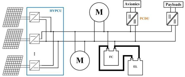
Figure 3: Global electrical architecture of Stratobus
