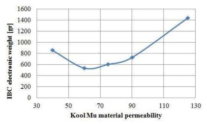
Figure 4: Weight of the IBC in CCM for different permeabilities of the Kool Mu inductor core (that are optimization results)
