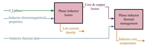
Figure 15: Power inductor losses and thermal models organization
