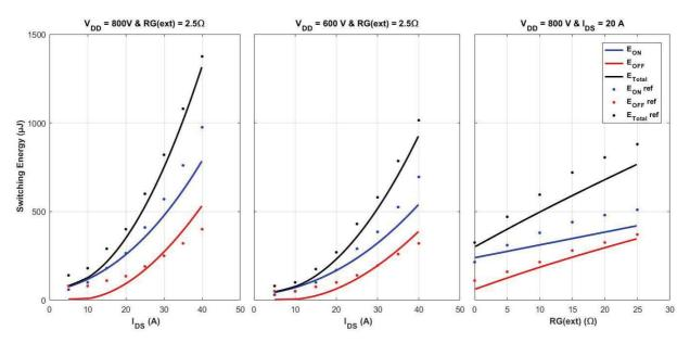
Figure 7: C2M0080120D switching energies evolvements: comparison between the estimation based on the analytical model with the identified parasitic elements (curves) and the manufacturer datasheet (points)
