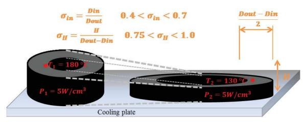
Figure 14: Power inductor quasi-homothetic coefficients definition
