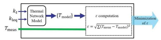
Figure 22: Inverse problem for calculating the thermal properties of Litz wire
