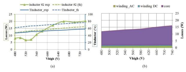
Figure 12: Phase inductor losses and temperatures: (a) comparison between experimental measurements (losses in green and temperature in blue lines) and analytical model (same colors than for the experiments but dashed lines), (b) inductor winding and core losses theoretical ratio
