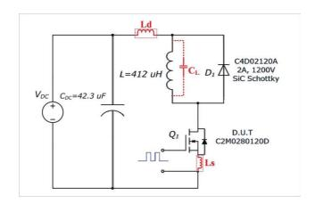
Figure 6: Clamped inductive switching waveform test circuit from [6]
