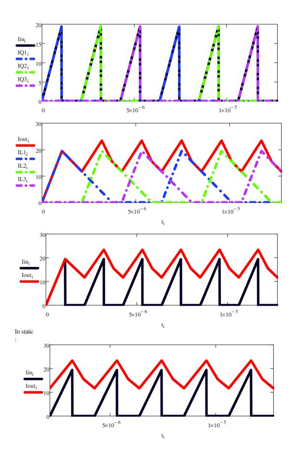
Appendix 2: Components parameters evaluation and IBC waveforms models capitalization
