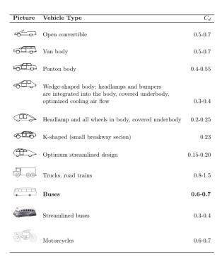
Figure 2.3: Coefficients of aerodynamic resistance [Schaltz, 2011]
