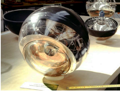
Figure 2.10 – Photograph and schematic of an ANTARES optical module.
