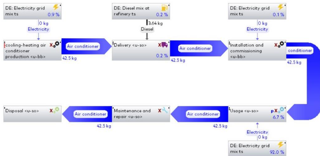
Figure 56 air conditioner lifecycle processes for Scenario 1
