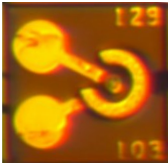
Figure 1.14: Top view of a VCSEL.
