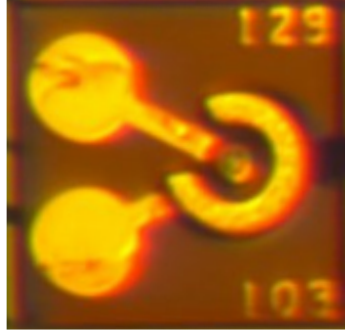
Figure 1.14: Top view of a VCSEL.
