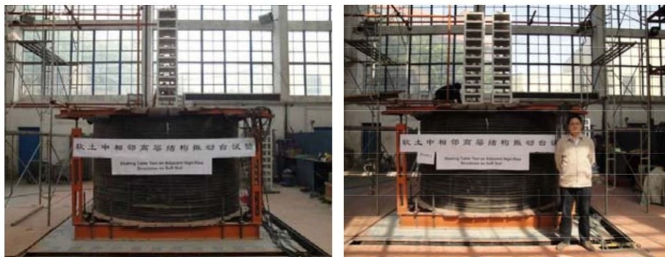
Figure 1-10 Prototype of a shaking table model scaled to the 1/15, SSI test model (left) and SSSI test model (right). (Li et al. 2012)
