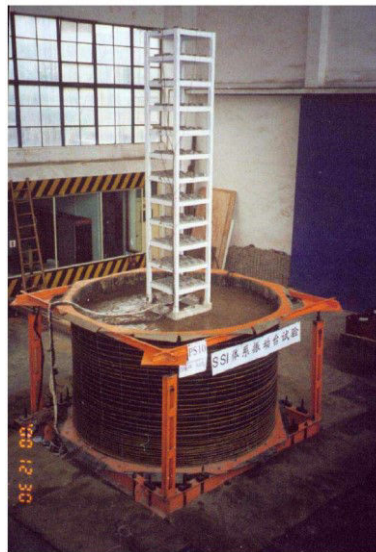
Figure 1-8 Photograph of a prototype model for the shaking table test. (Lu et al. 2004)
